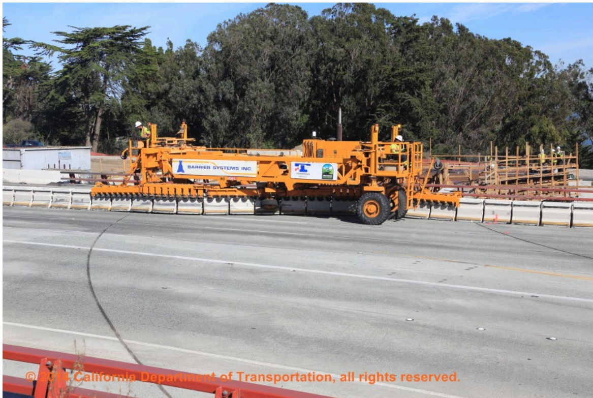
Figure 2: Movable Barrier System
