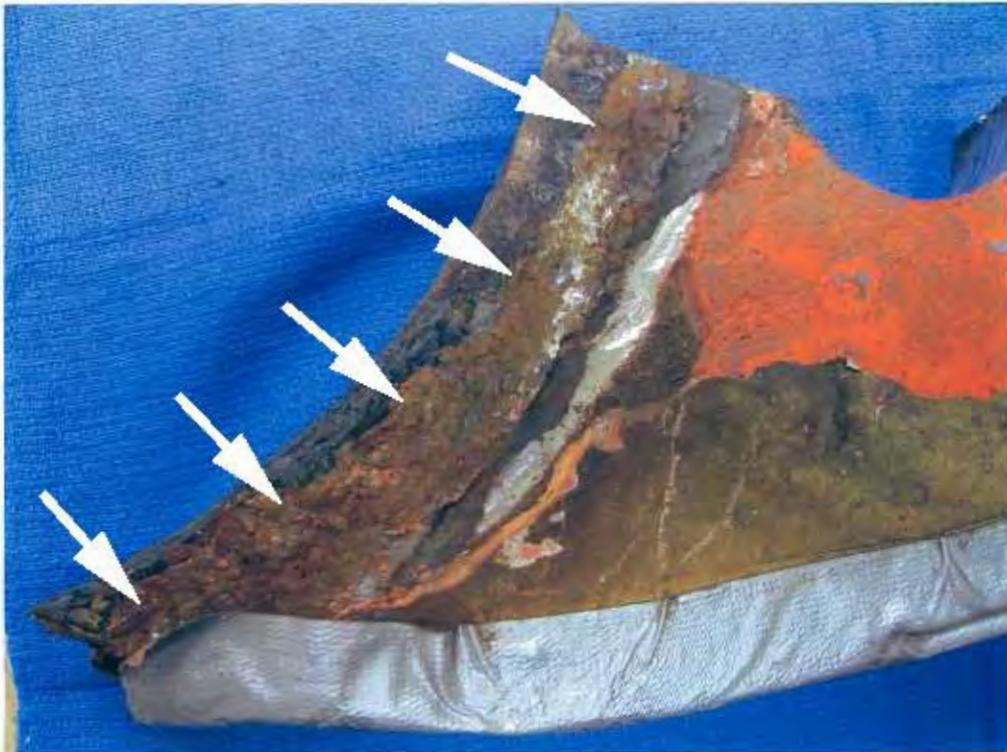
**Fig. 12 Corrosion and wear at sleeve location.**
