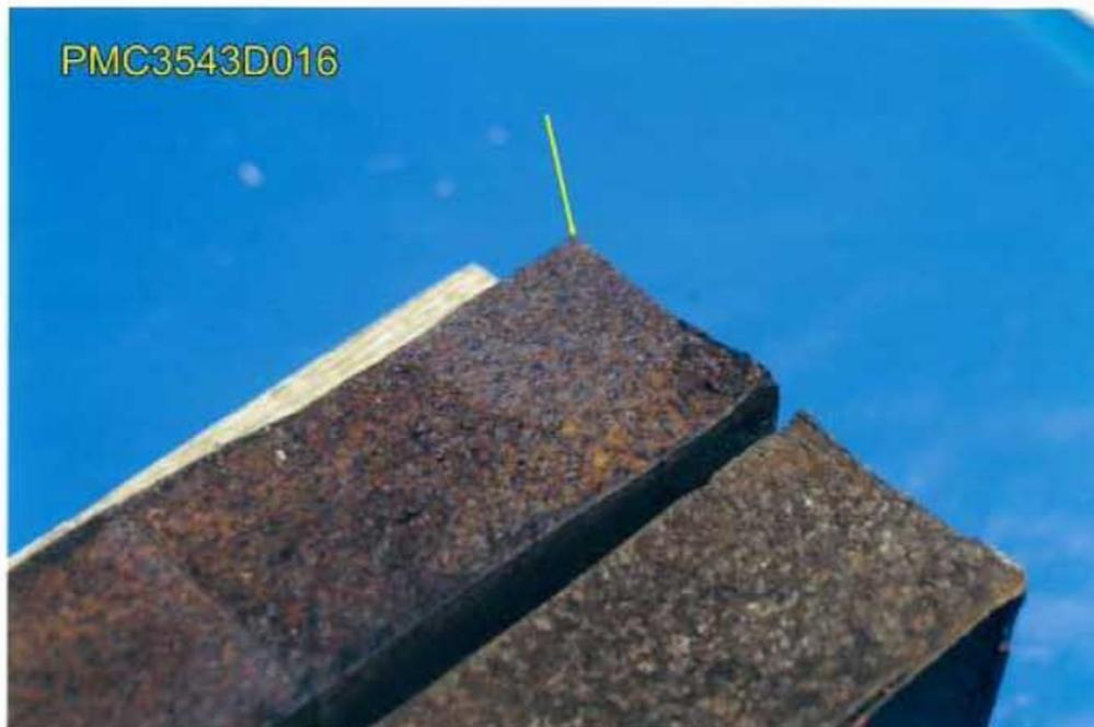
**Fig. 36 Fracture face outer edge. Fracture origin at arrow location.**
