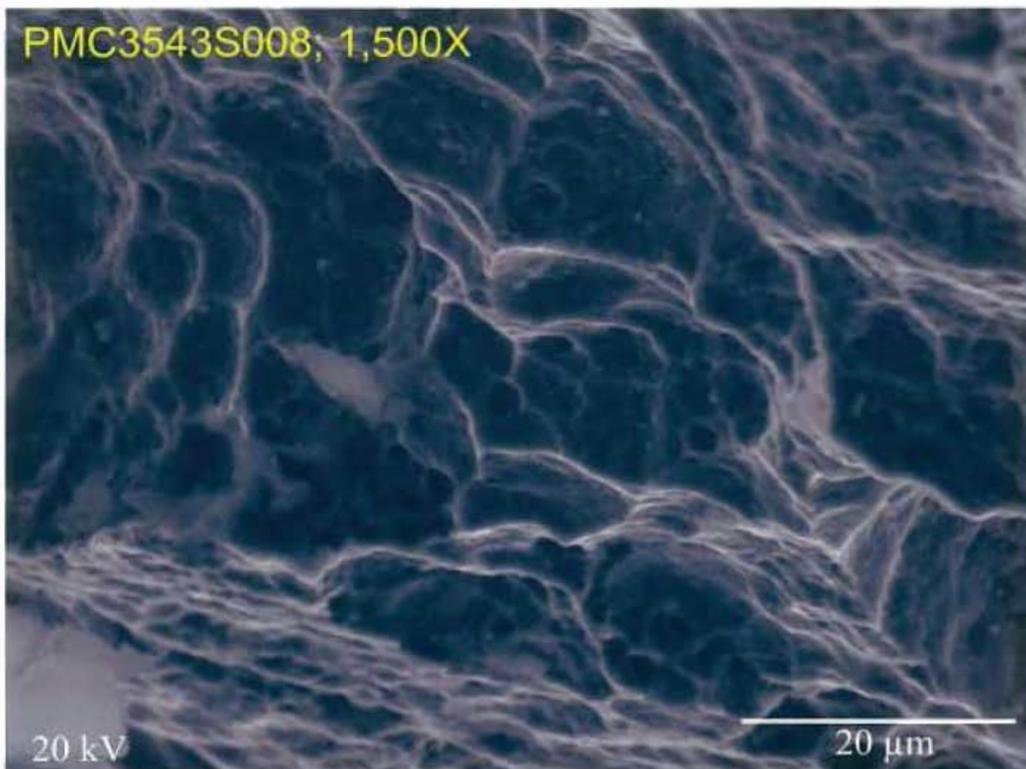
**Fig. 48 S.E.M photo of eye bar fracture surface at fracture origin, location 8 in fig. 47. 1,500X.**
