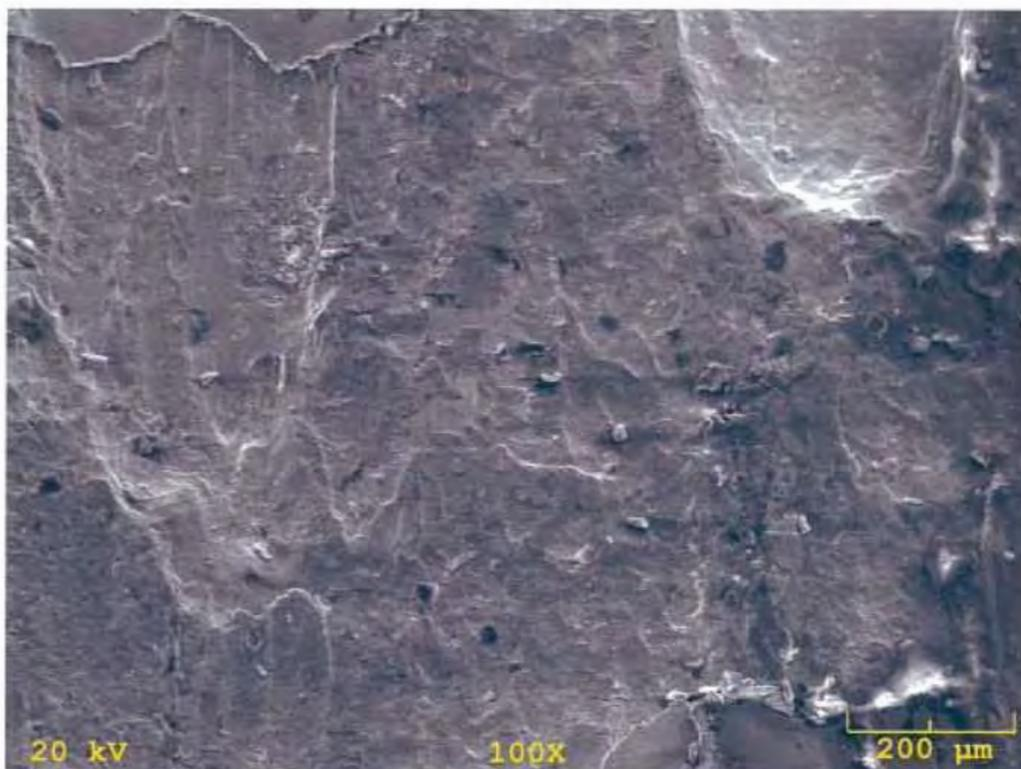
**Fig. 26 S.E.M photo of failed support rod from east span. Edge, below fracture origin. 100X.**
