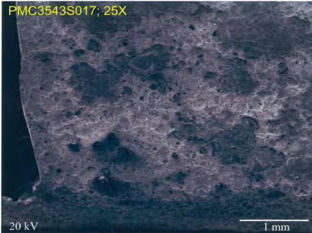
**Fig. 61 S.E.M photo of eye bar fracture surface, 2nd segment in fig. 35 at location 2, Shear lip. 25X.**
