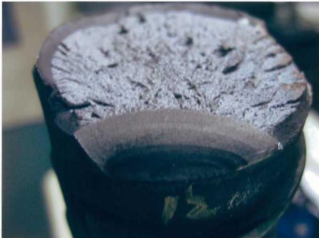
**Fig. 12 As received failed support rod from east span. Fracture sureface.**
