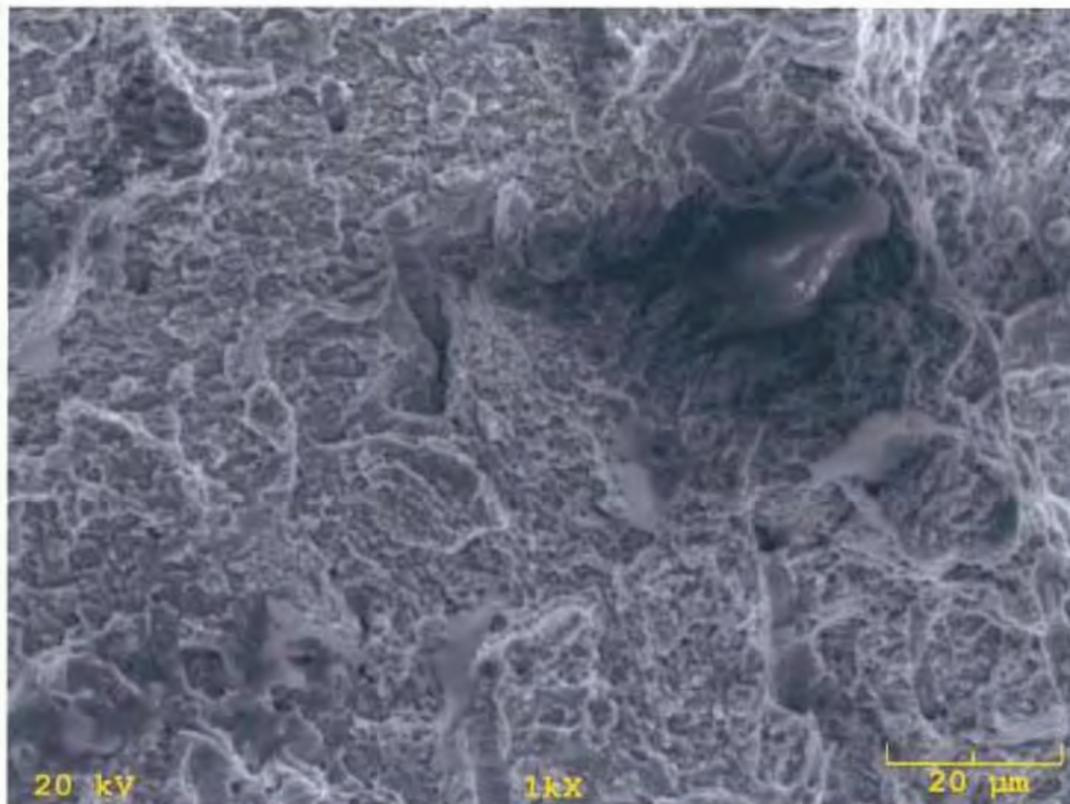
Fig. 42 S.E.M photo of failed support rod from east span shear lip edge, 1000X.
