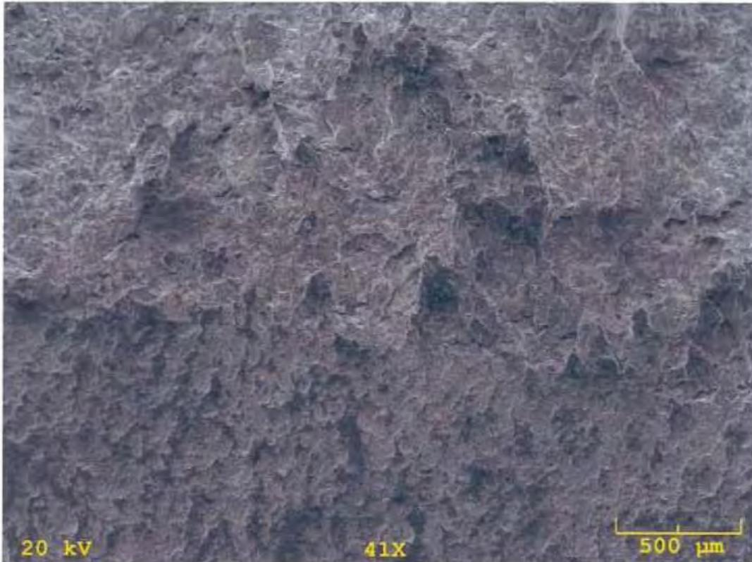
**Fig. 35 S.E.M photo of failed support rod from east span. Transition Zone 2-3. 41X.**
