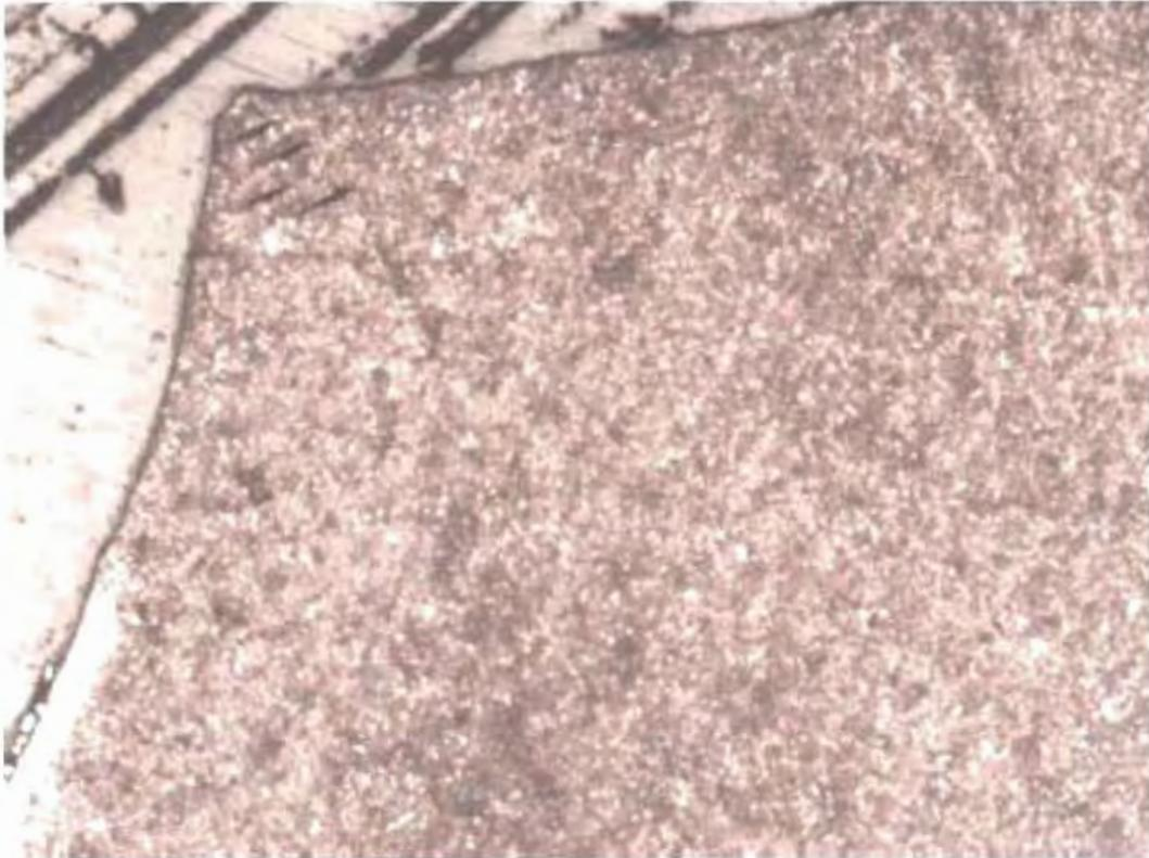
**Fig. 49** Cross-section of failed support rod from east span at fracture origin in fig. 16. 50X. Etched.
