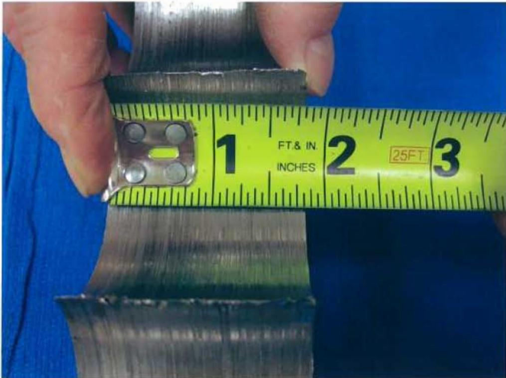
**Fig. 17 Thickness of eye bar.**
