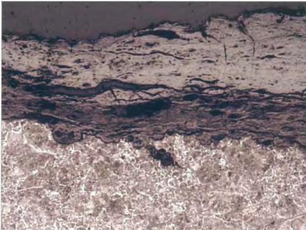
**Fig. 101** Longitudinal microsection of eye bar near the center pin location, in fig. 98, location A, showing fracture surface. 50X. Etched.
