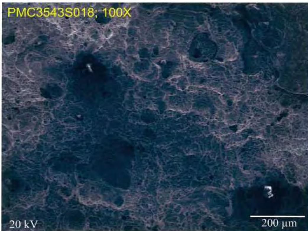
**Fig. 62 S.E.M photo of eye bar fracture surface, 2nd segment in fig. 35 at location 2, shear lip. 100X.**
