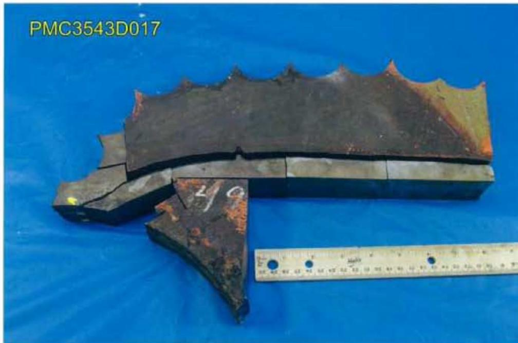
**Fig. 38 Upper and lower portion of fractured eye bar, opposite side.**
