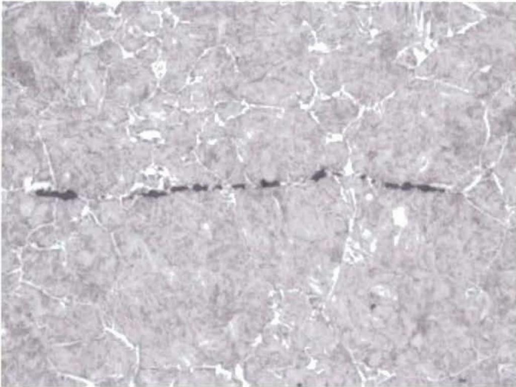
**Fig. 85 Microstructure of sample # 4 showing elongated inclusion. 200X. Etched.**
