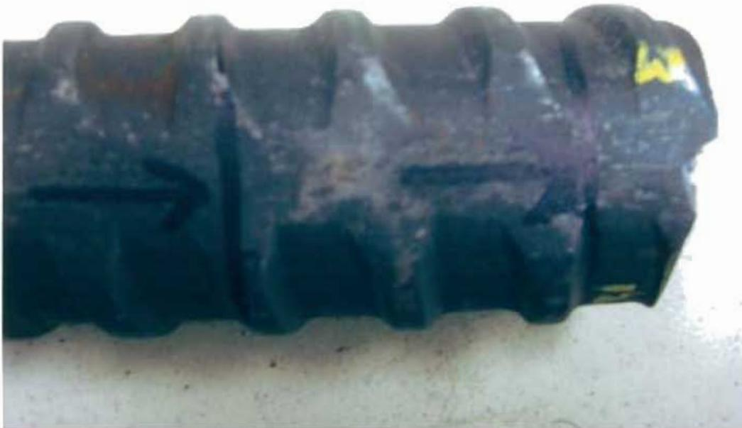
**Fig. 14 As received failed support rod from east span. Location where longitudinal microsection was made.**
