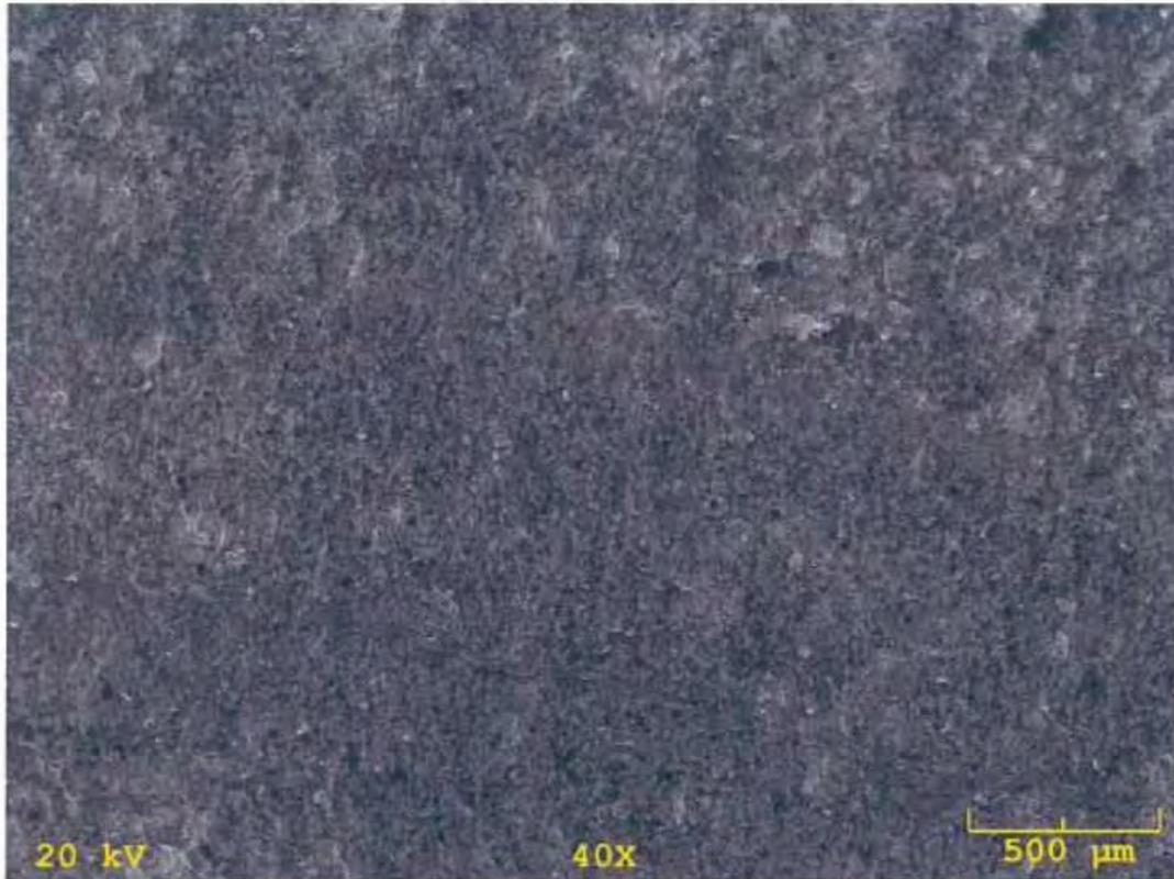
**Fig. 31 S.E.M photo of failed support rod from east span at fracture origin. Zone 1. 40X.**
