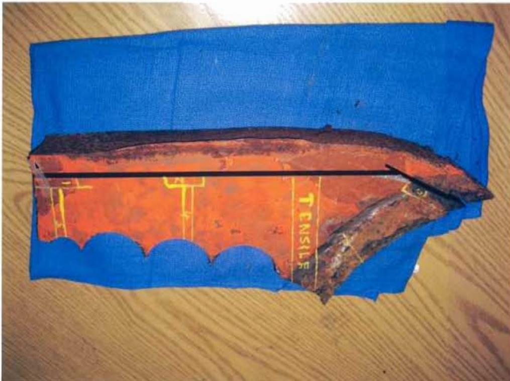
**Fig. 18 Cut locations to remove micros, tensile, and chemistry samples.**
