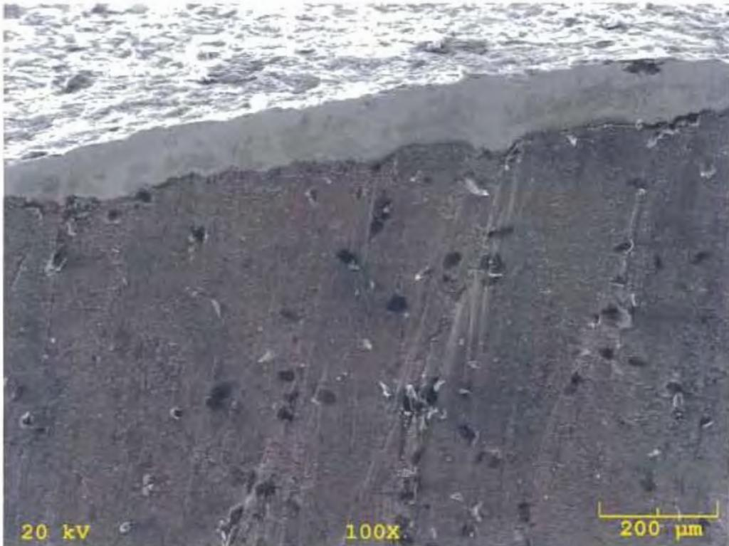
Fig. 23 S.E.M photo of failed support rod from east span. Edge, below fracture origin. 100X.
