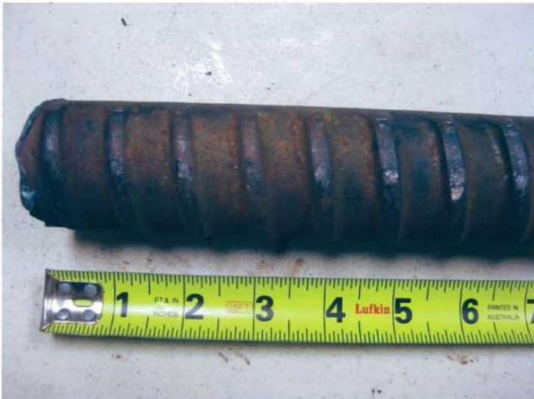
**Fig. 6** As received failed support rod from east span. 12 O'clock position.
