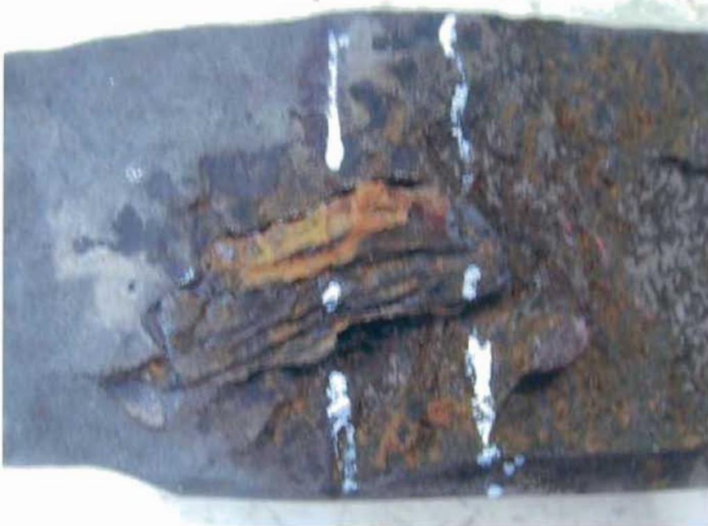
**Fig. 89** Transverse cross-section made of eye bar near the center pin location.
