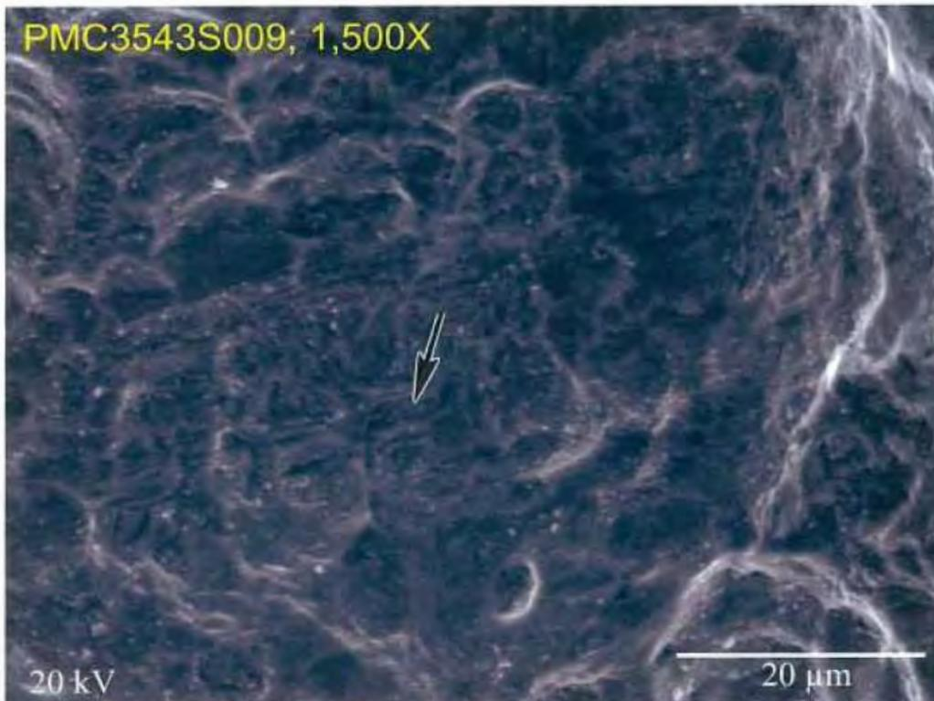
**Fig. 49 S.E.M photo of eye bar fracture surface at fracture origin, location 9 in fig. 45. 1,500X.**
