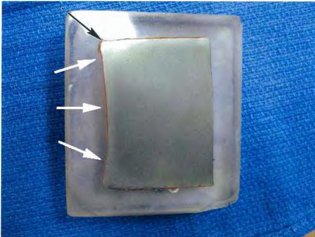
**Fig. 71 Microsection made below fracture surface at location 1, in fig 20.**
