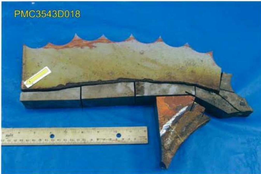
**Fig. 37 Upper and lower portion of fractured eye bar.**
