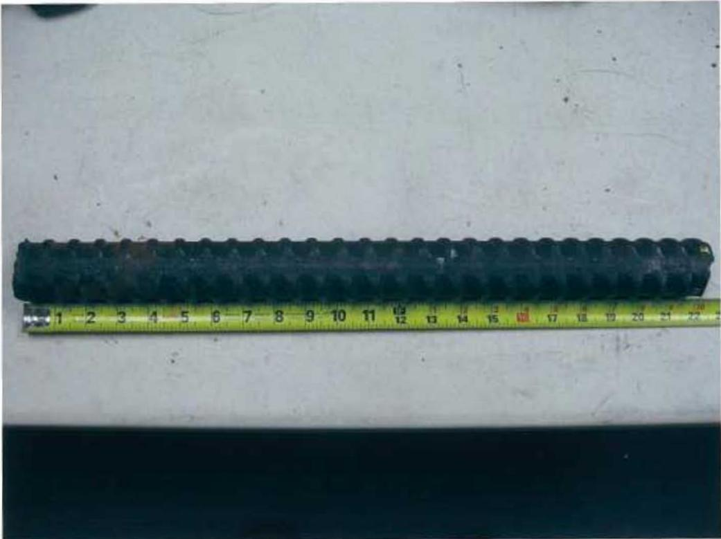
Fig. 1 As received failed support rod from east span.
