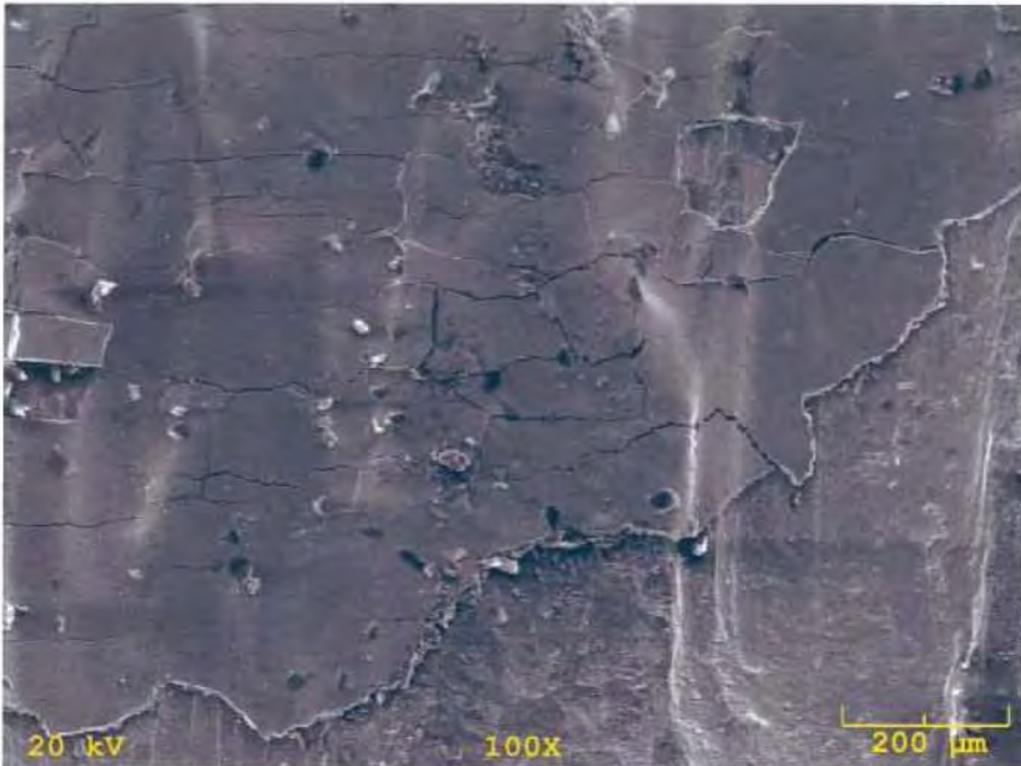
**Fig. 25 S.E.M photo of failed support rod from east span. Edge, below fracture origin. 100X.**
