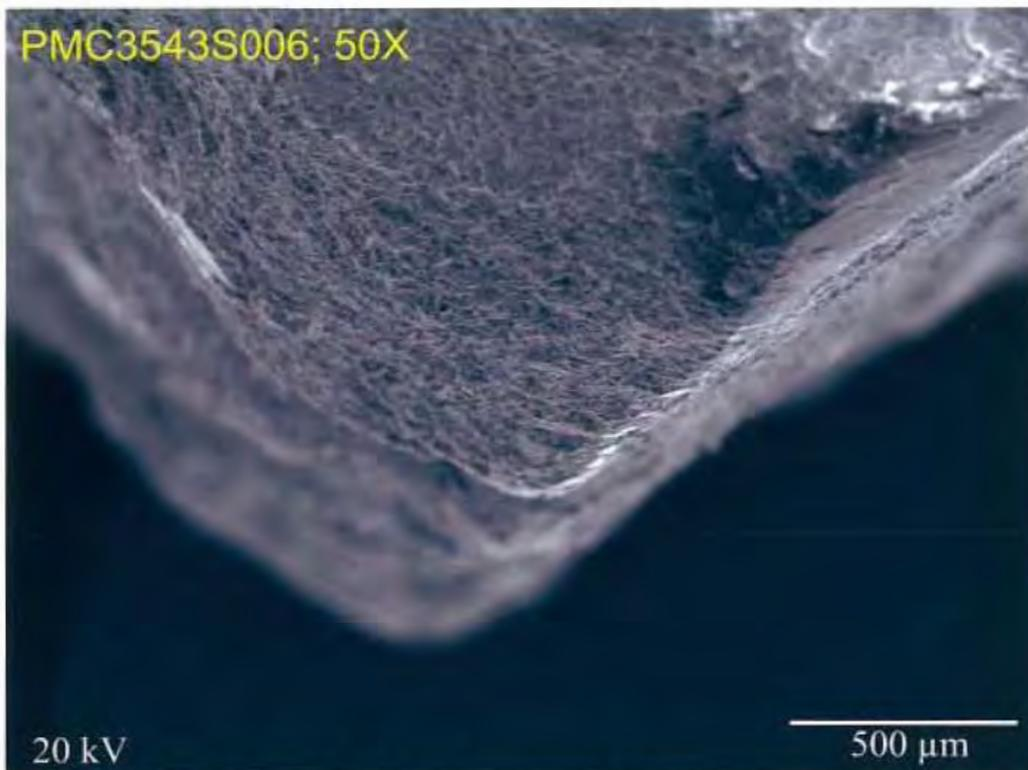
Fig. 46 S.E.M photo of eye bar fracture surface at fracture origin, location 6 in fig. 45. 50X.
