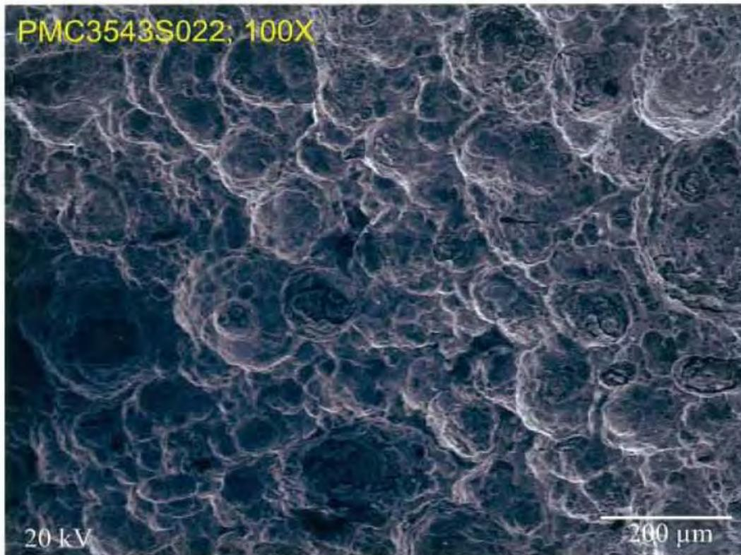
**Fig. 66 S.E.M photo of eye bar fracture surface, 4th segment in fig. 35 at location 4, top edge, area 1. 100X.**
