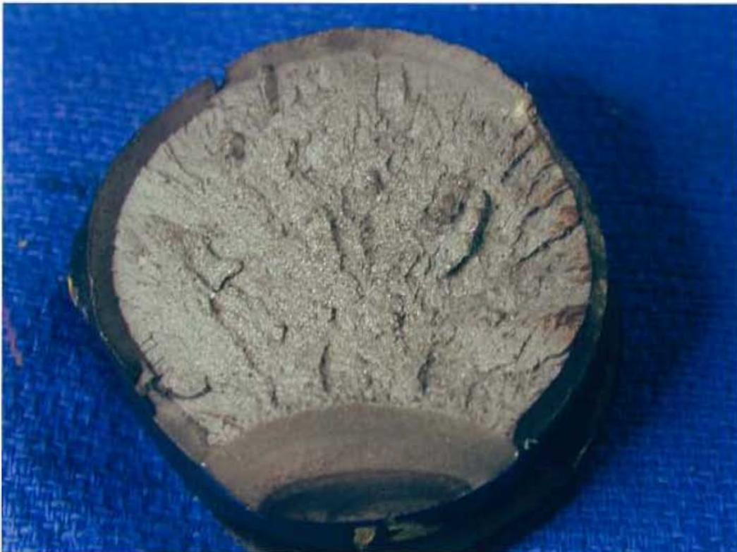
**Fig. 16** As received failed support rod from east span. Fracture surface.
