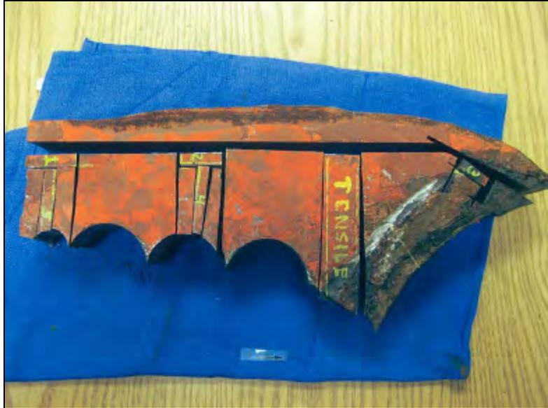
**Figure 9: Cut locations to remove micros.**
