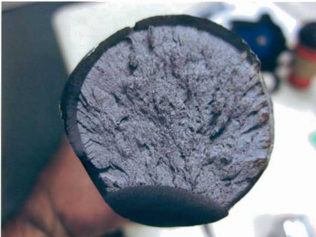
**Fig. 10 As received failed support rod from east span. Fracture sureface.**
