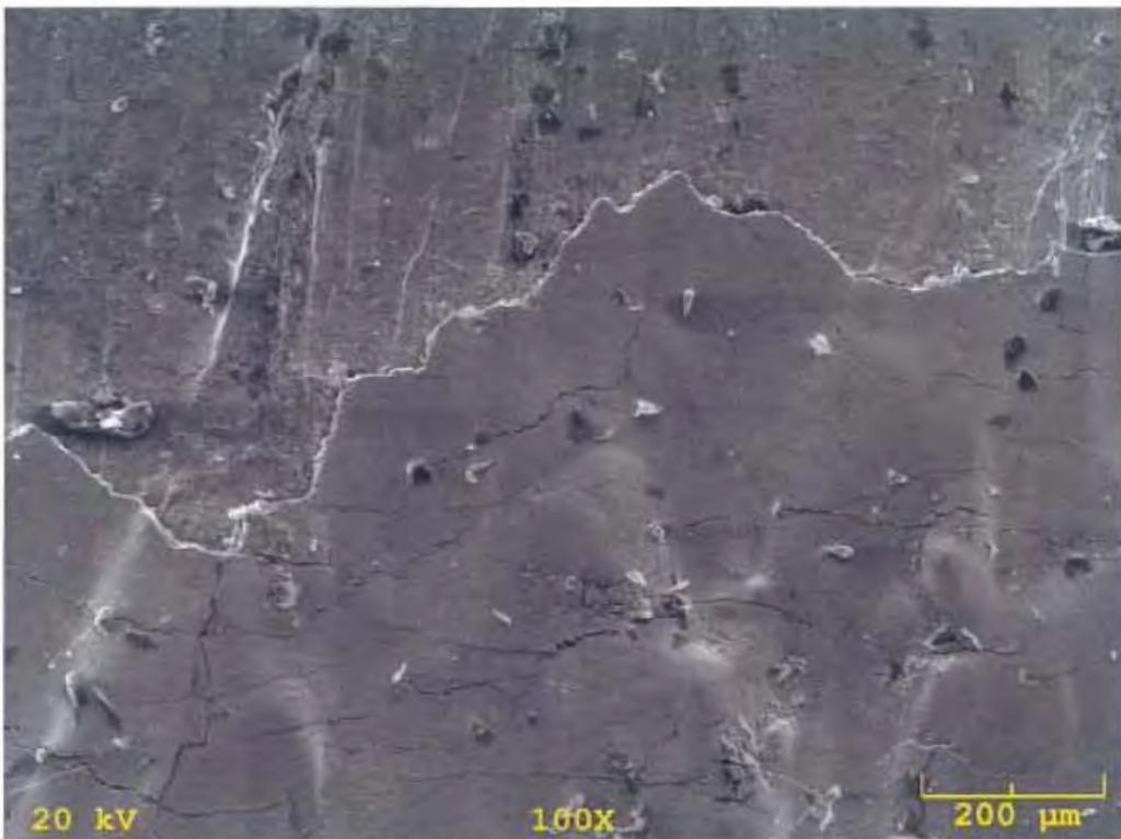
Fig. 24 S.E.M photo of failed support rod from east span. Edge, below fracture origin. 100X.
