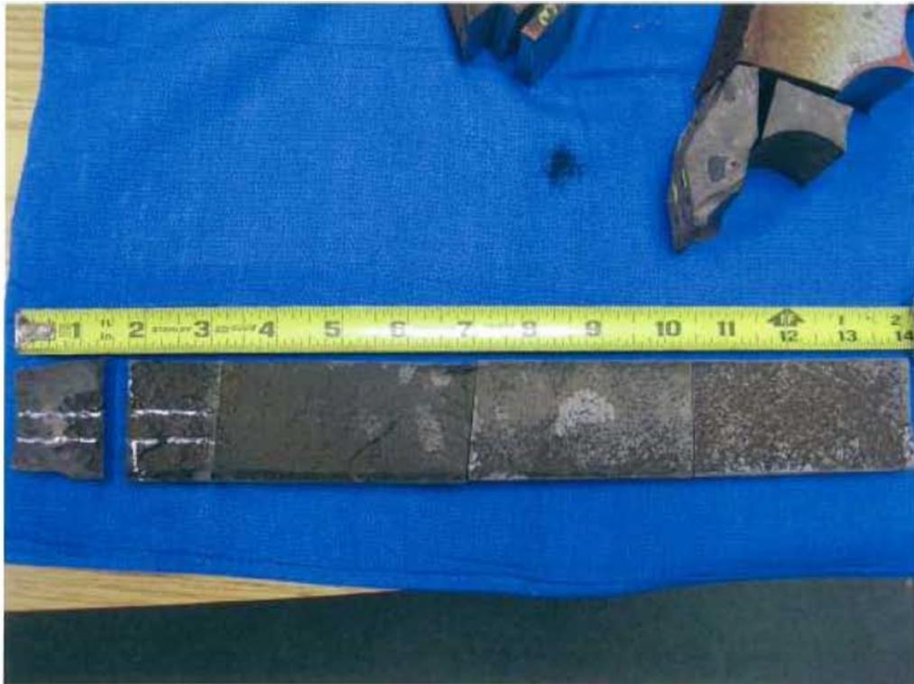
**Fig. 97** Location where longitudinal microsections were made of eye bar near the center pin location.
