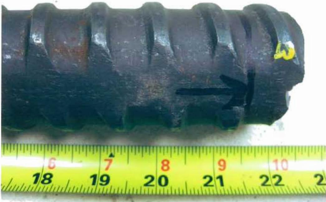
Fig. 7 As received failed support rod from east span. 3 O'clock position.
