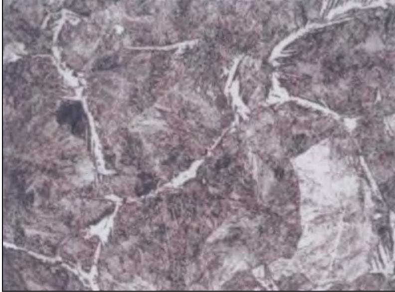
**Figure 11: Core microstructure of sample #1 in Figure 10. 500x Etched.**
