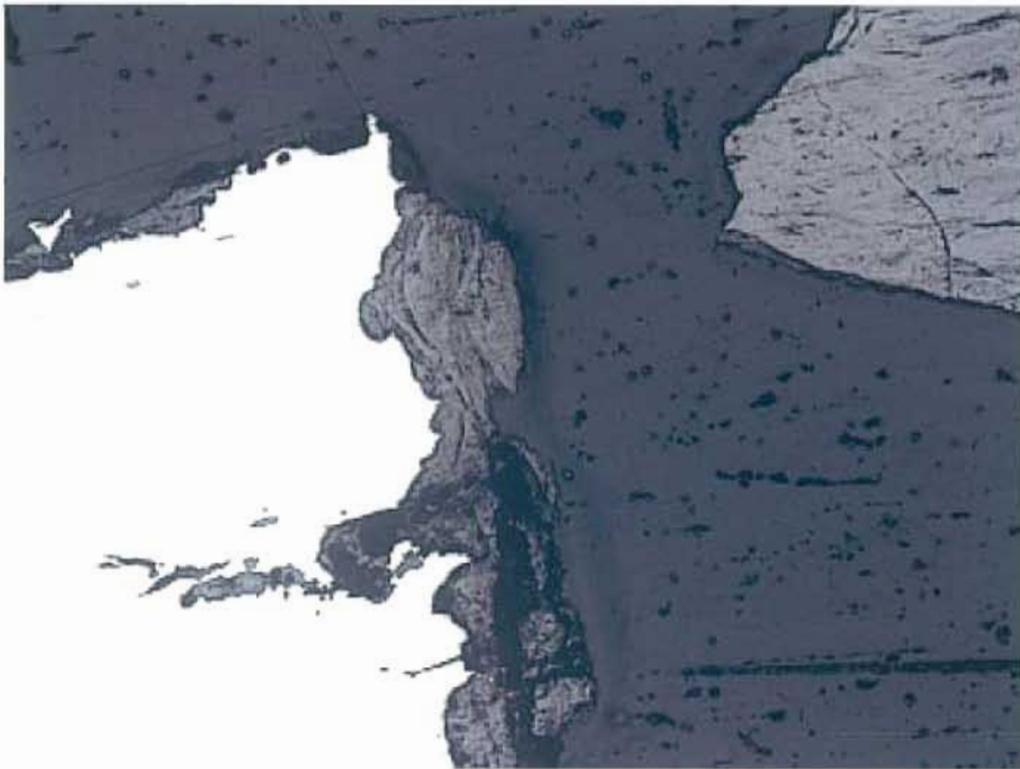
**Fig. 92** Transverse cross-section made of eye bar near the center pin location, showing fracture face and scale. 100X.
