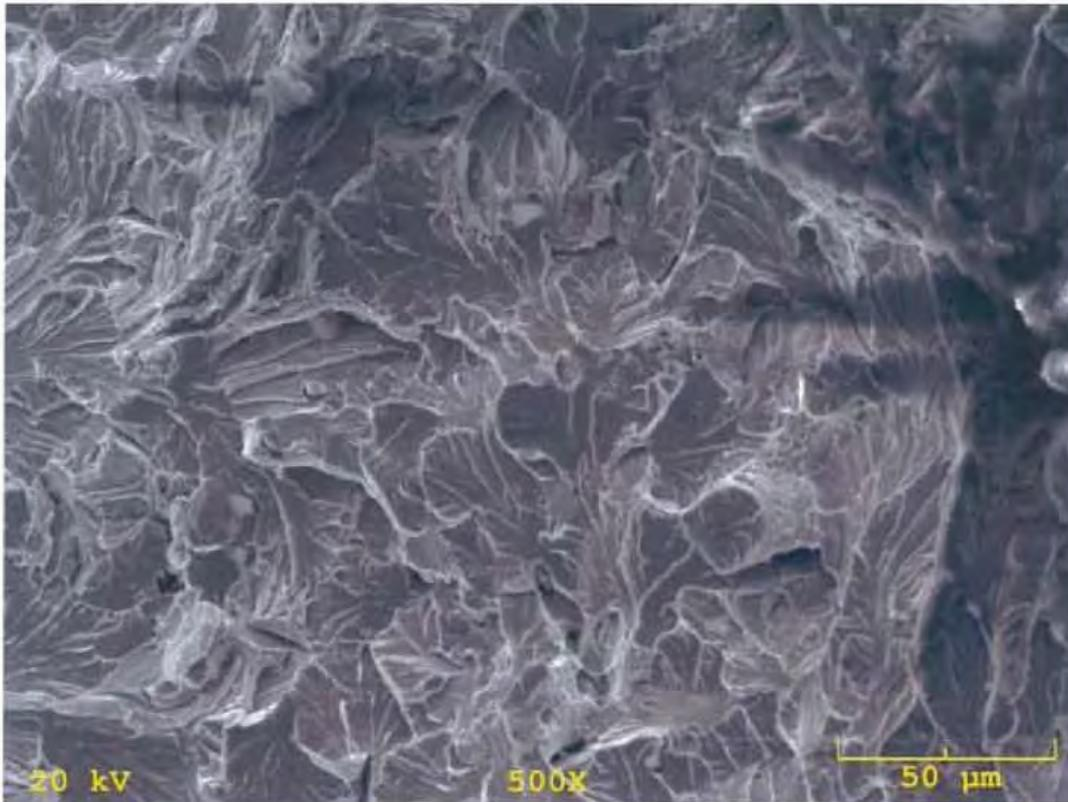
**Fig. 39 S.E.M photo of failed support rod from east span on fracture surface. Above zone 2 in zone 3. 500X.**
