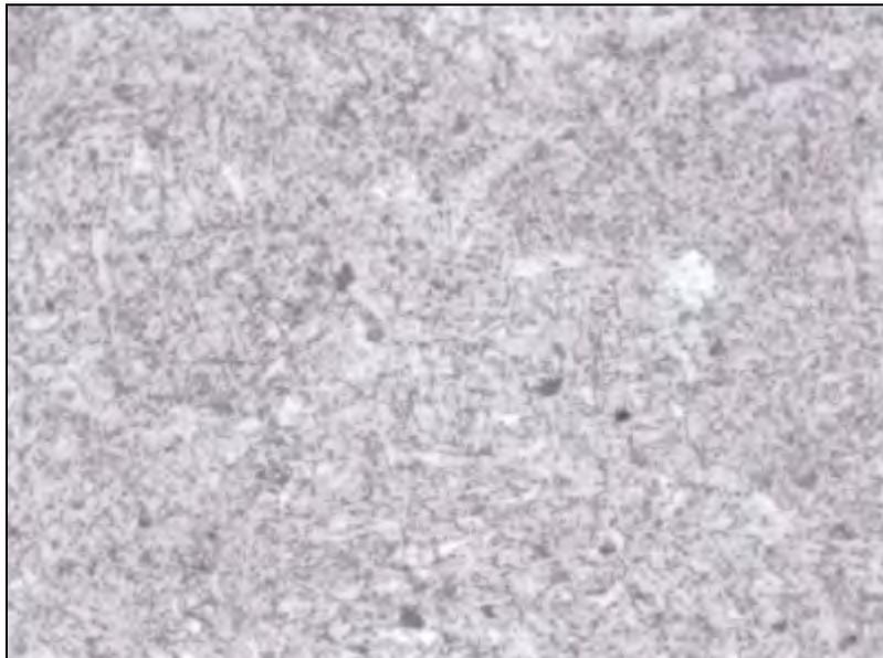
**Figure 10: Microstructure near top corner of sample #1 in Figure 6. 500x Etched.**
