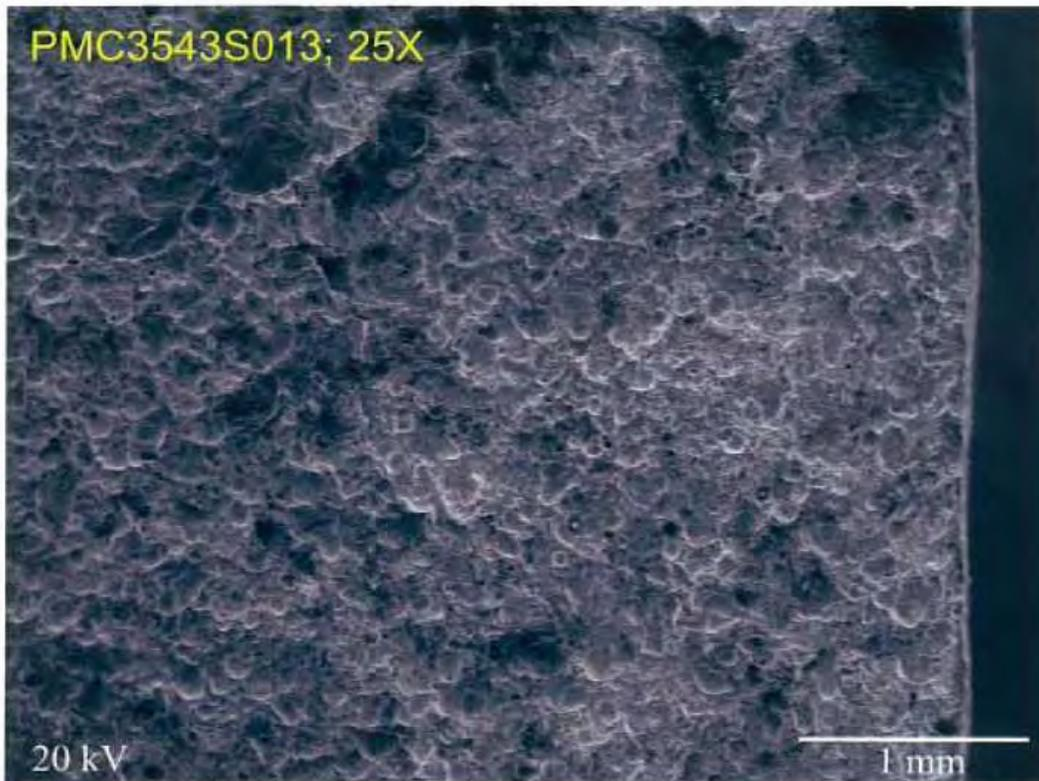
**Fig. 57 S.E.M photo of eye bar fracture surface, 2nd segment in fig. 35 at location 2, right edge. 25X.**
