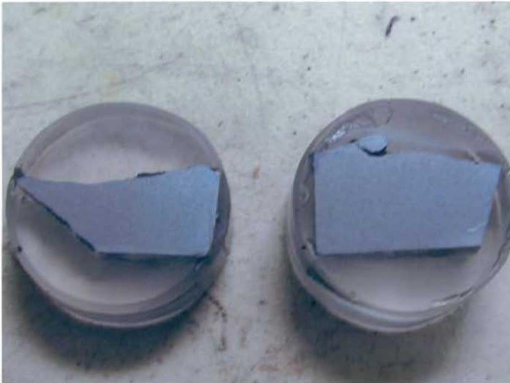
**Fig. 99** Longitudinal microsections of eye bar near the center pin location, in fig. 98.
