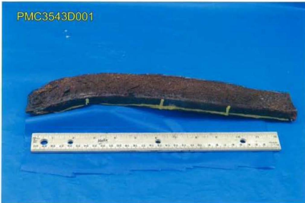
**Fig. 21 Fracture face of eye bar, upper portion.**
