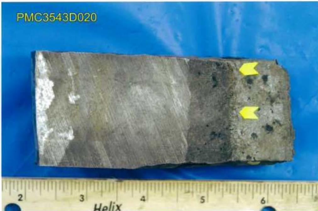
**Fig. 40 Inside portion of fracture face, adjacent to pin location, after cleaning of oxide layer.**
