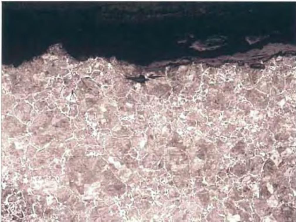
**Fig. 95** Transverse cross-section made of eye bar near the center pin location, showing microstructure below fracture face. 100X. Etched.
