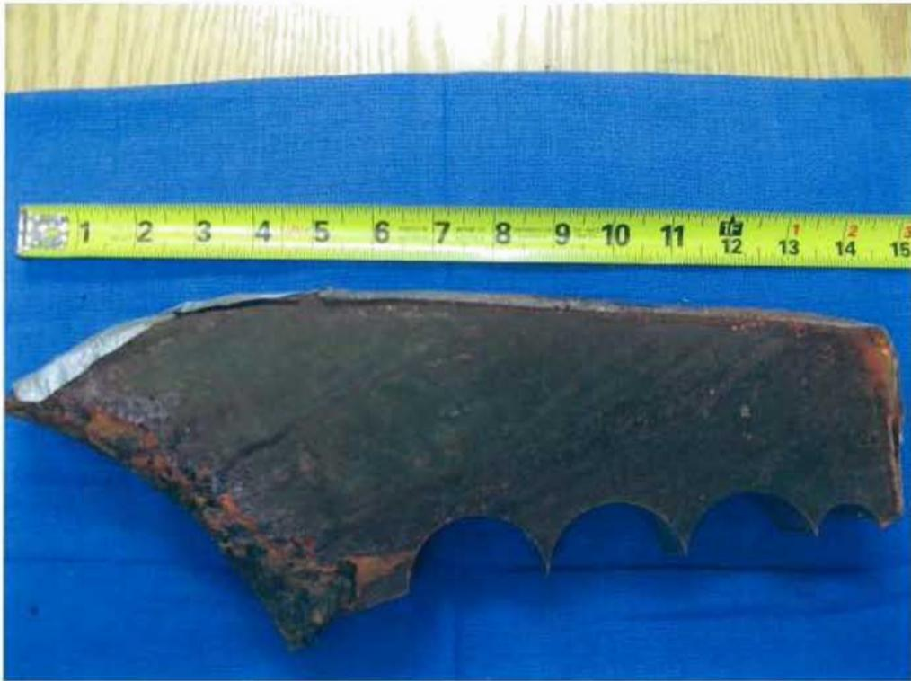
**Fig. 15 Fracture face segment upper portion, opposite side.**
