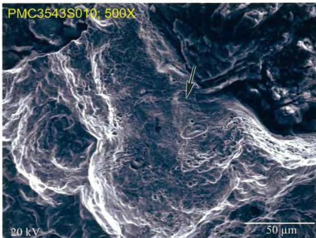
**Fig. 50 S.E.M photo of eye bar fracture surface at fracture origin, in fig. 45. 500X.**
