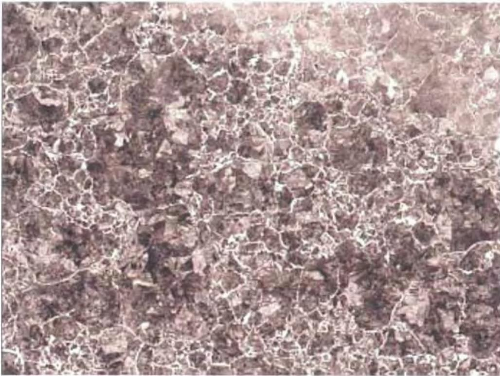
**Fig. 96** Transverse cross-section made of eye bar near the center pin location, showing microstructure below fracture face. 100X. Etched.
