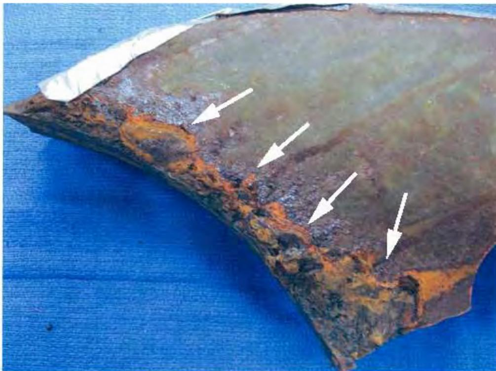
**Fig. 14** Corrosion and wear at sleeve location, opposite side.
