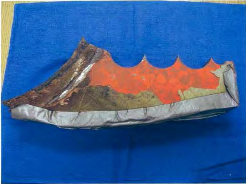
**Fig. 11 Fracture face segment upper portion.**
