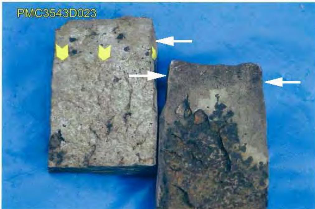
**Fig. 43** Mating fracture faces of eye bar outboard from pin location, after cleaning of oxide layer.
