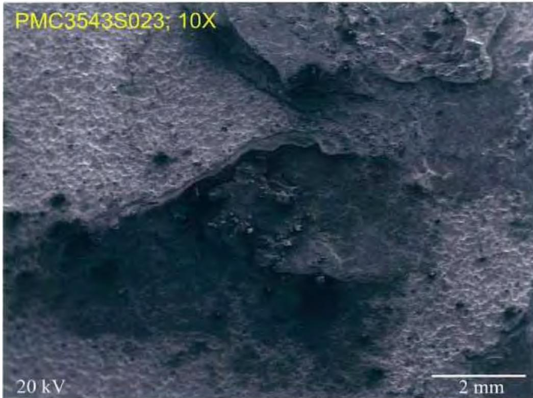
**Fig. 67 S.E.M photo of eye bar fracture surface, 4th segment in fig. 35 at location 4, transition, area 2. 10X.**
