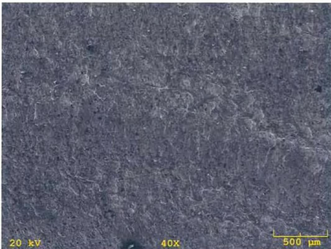
**Fig. 30 S.E.M photo of failed support rod from east span. inboard from fracture origin. 40X.**
