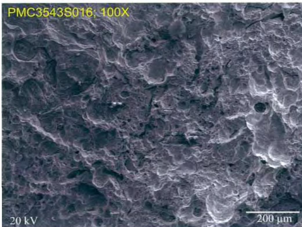
**Fig. 60 S.E.M photo of eye bar fracture surface, 2nd segment in fig. 35 at location 2, Center zone. 100X.**
