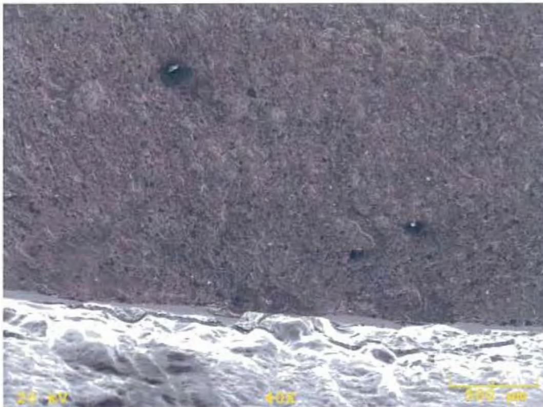
**Fig. 28 S.E.M photo of failed support rod from east span. Edge, at fracture origin. 40X.**
