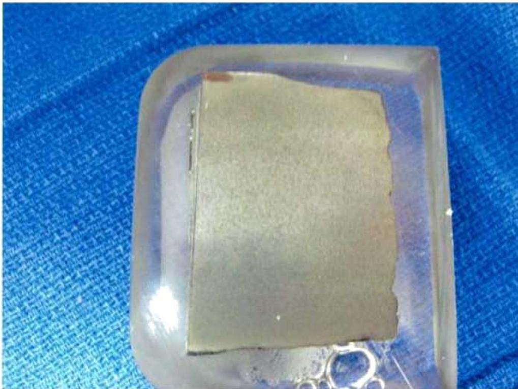
**Fig. 78 Microsection made below fracture surface at location 3 in fig. 20.**
