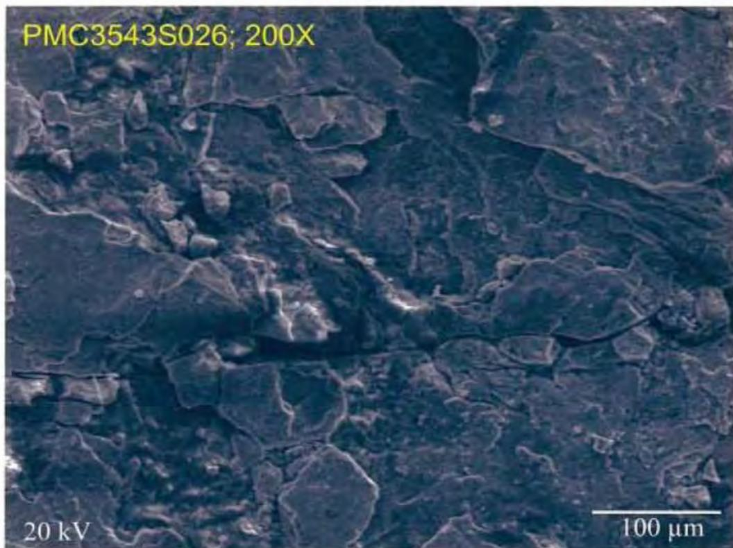
**Fig. 70 S.E.M photo of eye bar fracture surface, 4th segment in fig. 35 at location 4, oxide layer in fig. 68. 200X.**
