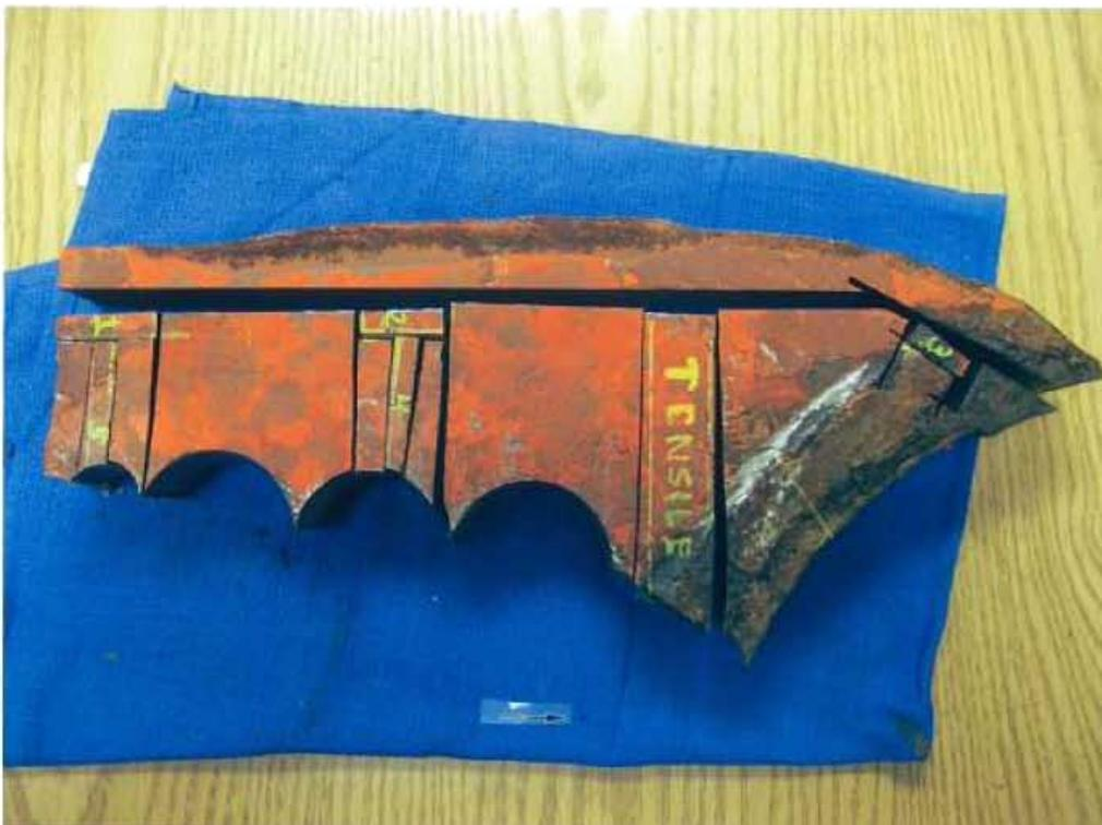
**Fig. 20 Cut locations to remove micros, tensile, and chemistry samples.**
