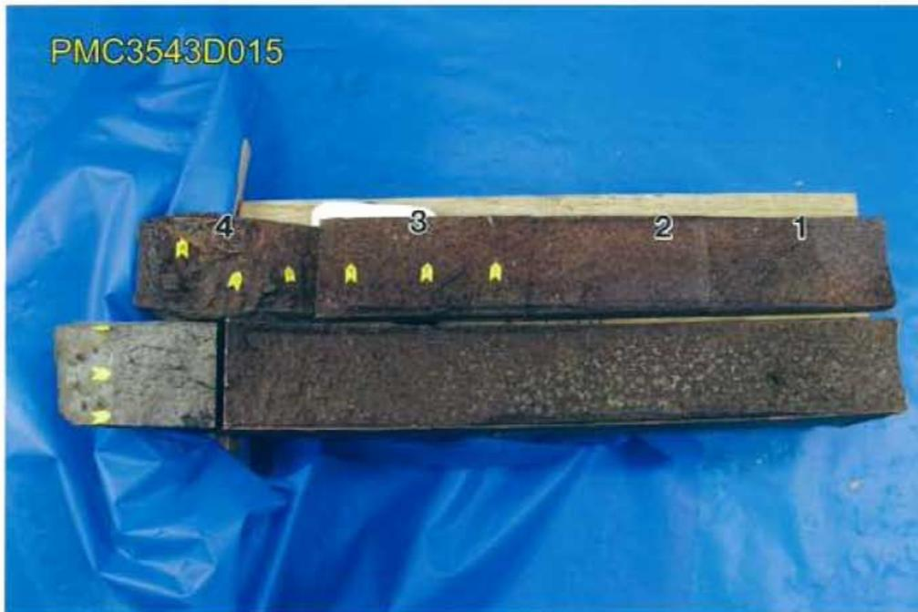
**Fig. 35 Mating fracture faces.**
