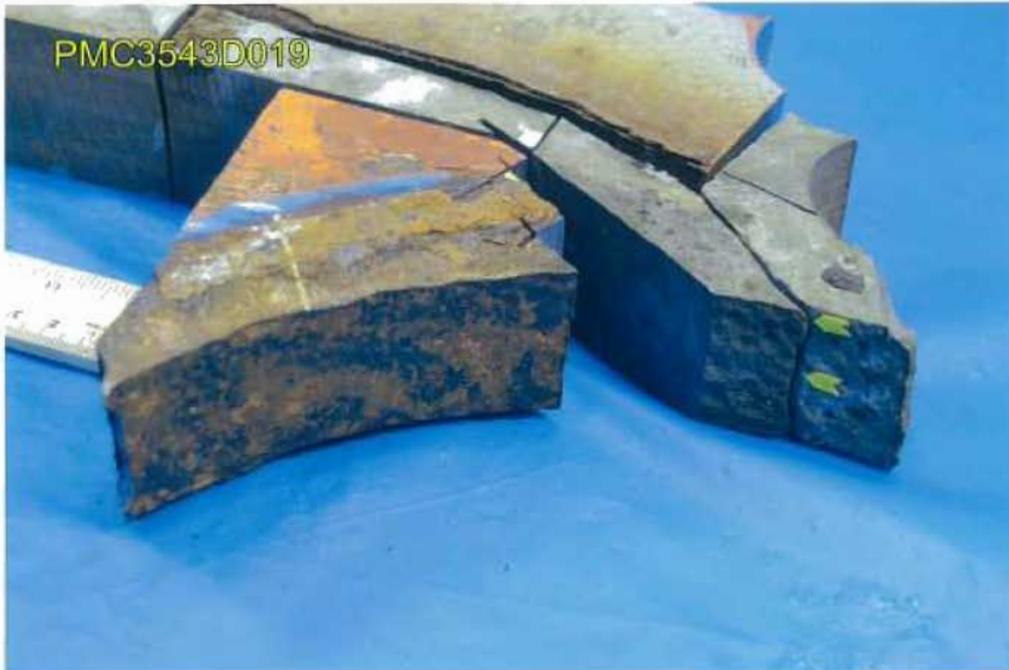
**Fig. 39 Inside diameter surface of eye bar pin location.**
