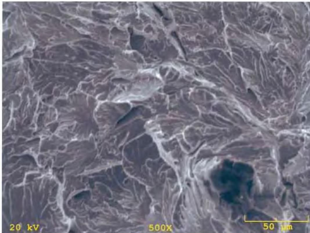
**Fig. 40 S.E.M photo of failed support rod from east span middle of fracture surface. 500X.**
