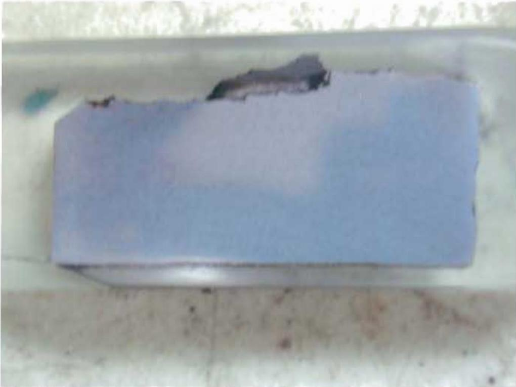
**Fig. 91** Transverse cross-section made of eye bar near the center pin location.
