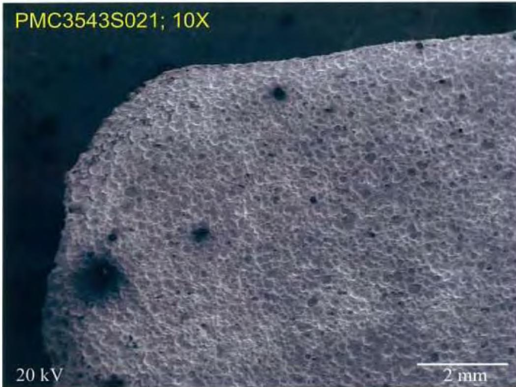
**Fig. 65 S.E.M photo of eye bar fracture surface, 4th segment in fig. 35 at location 4, top edge, area 1. 10X.**
