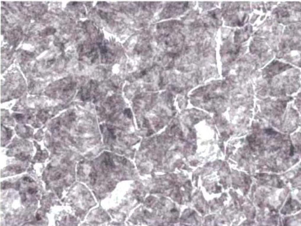
**Fig. 74 Core microstructure of sample #1 in fig. 71. 200X Etched.**
