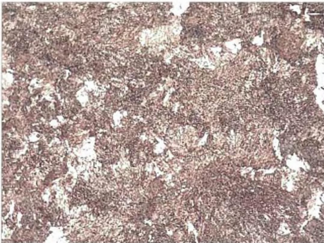
**Fig. 46** Longitudinal cross-section of failed support rod from east span. Microstructure at location 3 in fig. 43. 500X. Etched.
