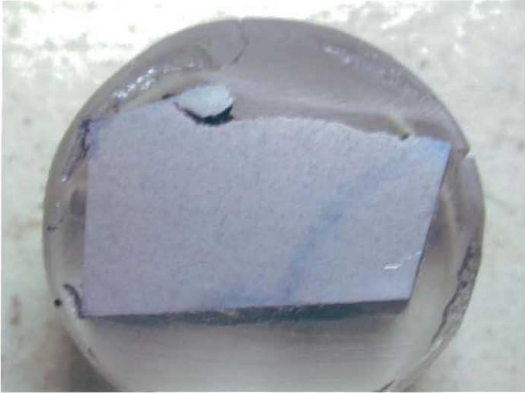
**Fig. 105** Longitudinal microsection of eye bar near the center pin location, in fig. 98, location B.
