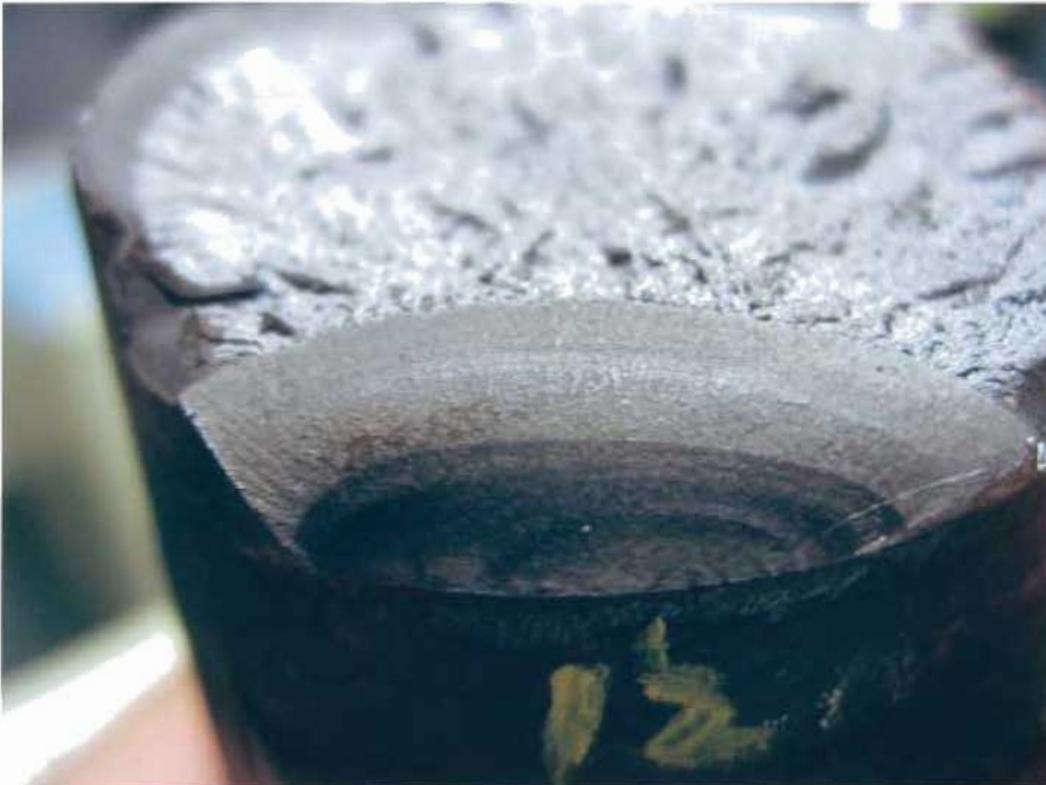
**Fig. 13 As received failed support rod from east span. Fracture sureface.**
