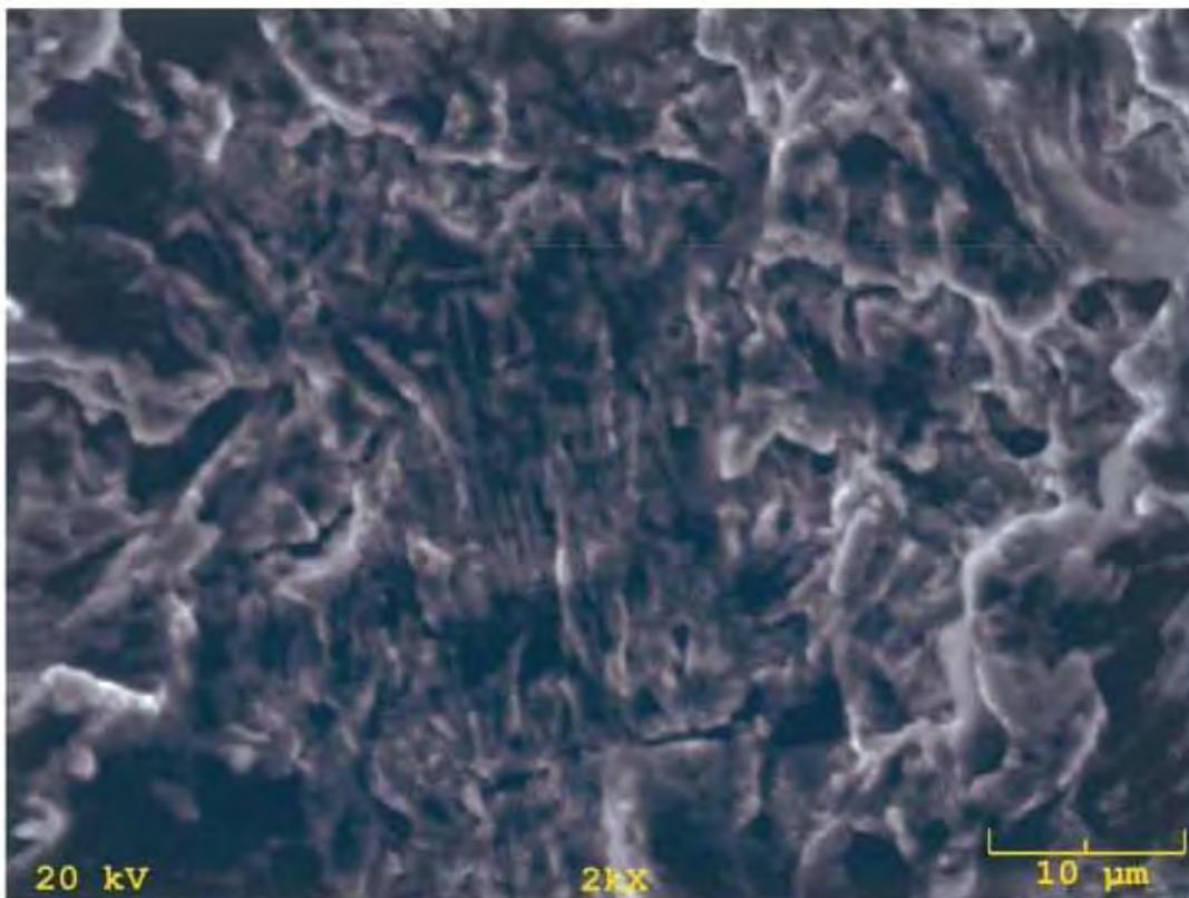
**Fig. 34 S.E.M photo of failed support rod from east span at fracture origin. Zone 2. 2000X.**
