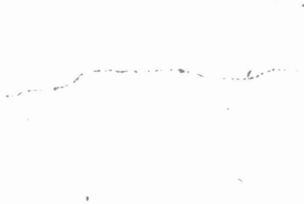
**Fig. 82** Elongated inclusion in microsection sample # 4. 100X
