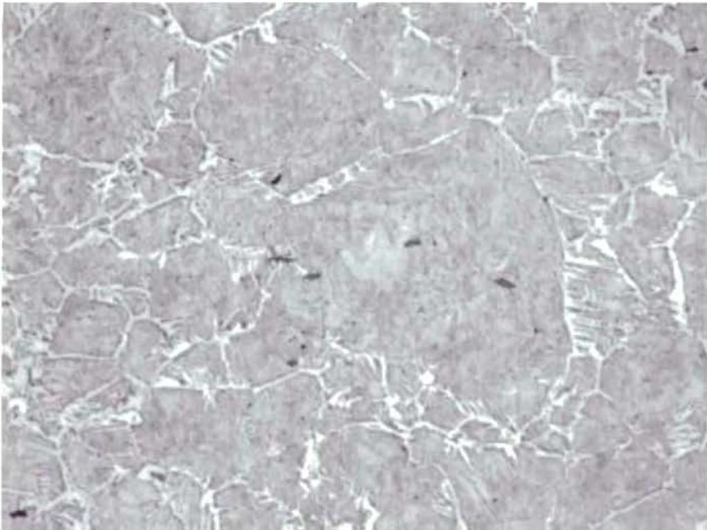
**Fig. 77 Core microstructure of sample # 2 in fig. 76. 200X Etched.**
