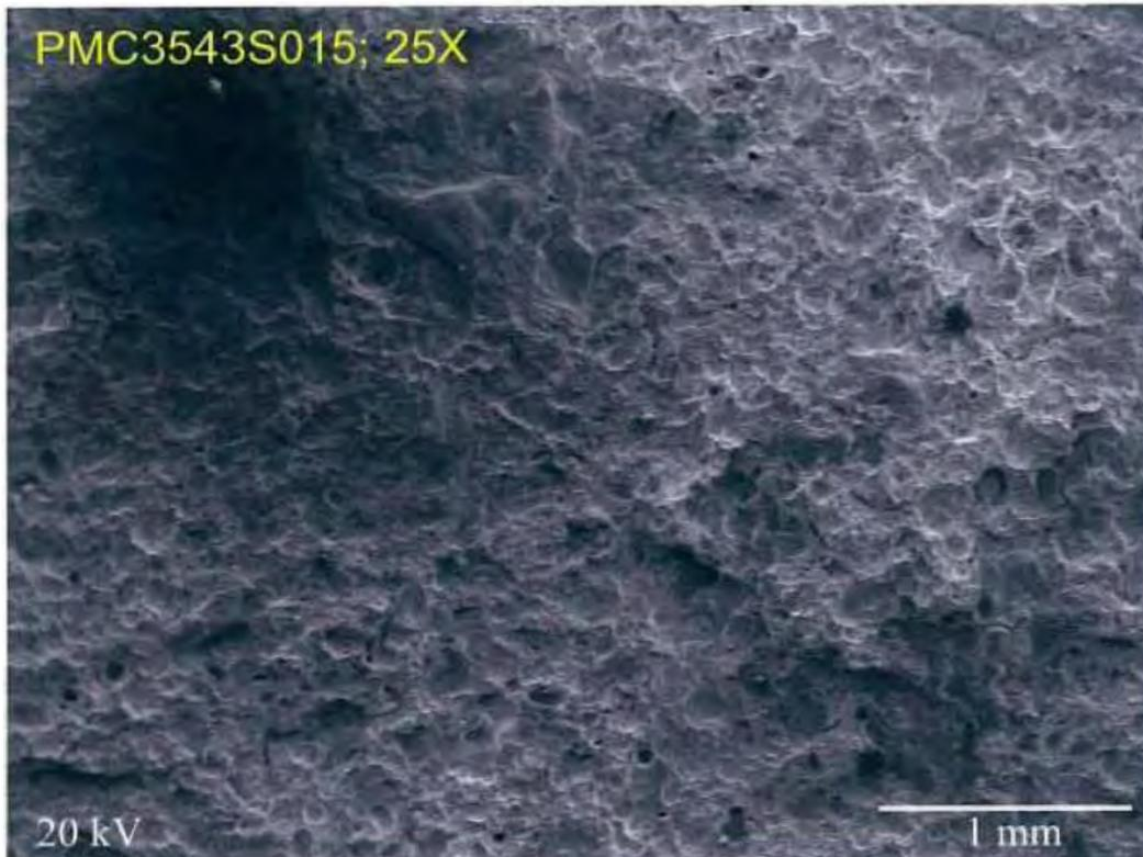
**Fig. 59 S.E.M photo of eye bar fracture surface, 2nd segment in fig. 35 at location 2, Center zone. 25X.**
