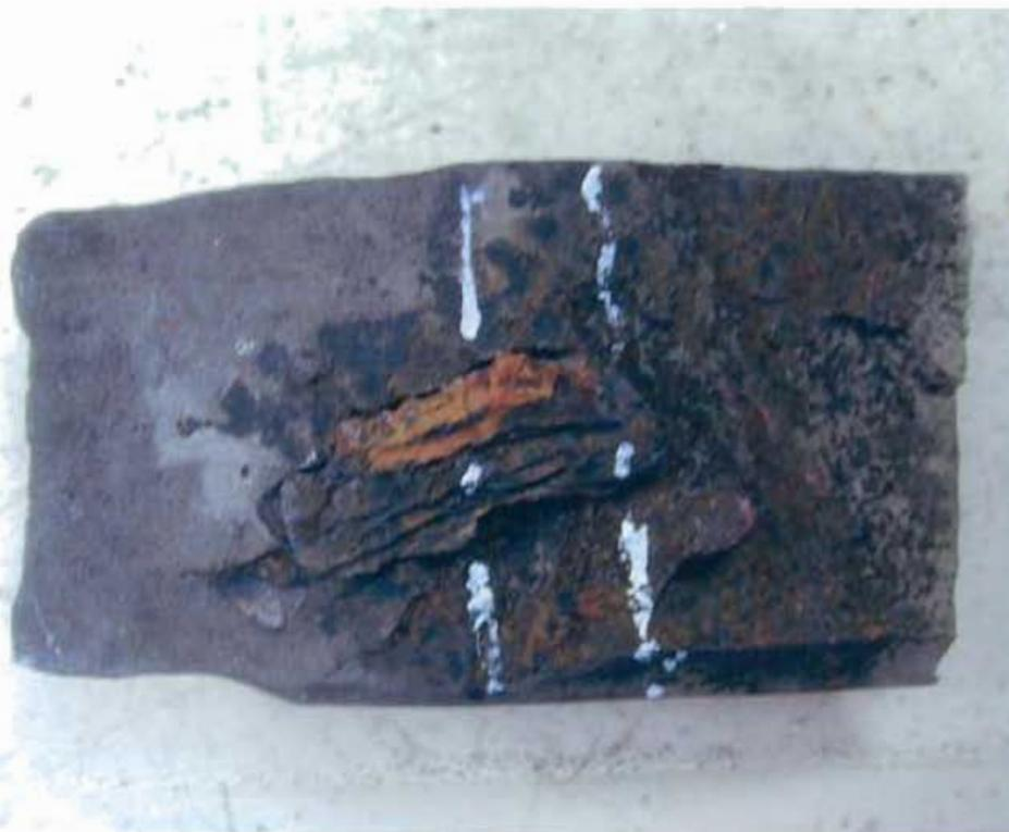
**Fig. 88 Transverse cross-section made of eye bar near the center pin location.**
