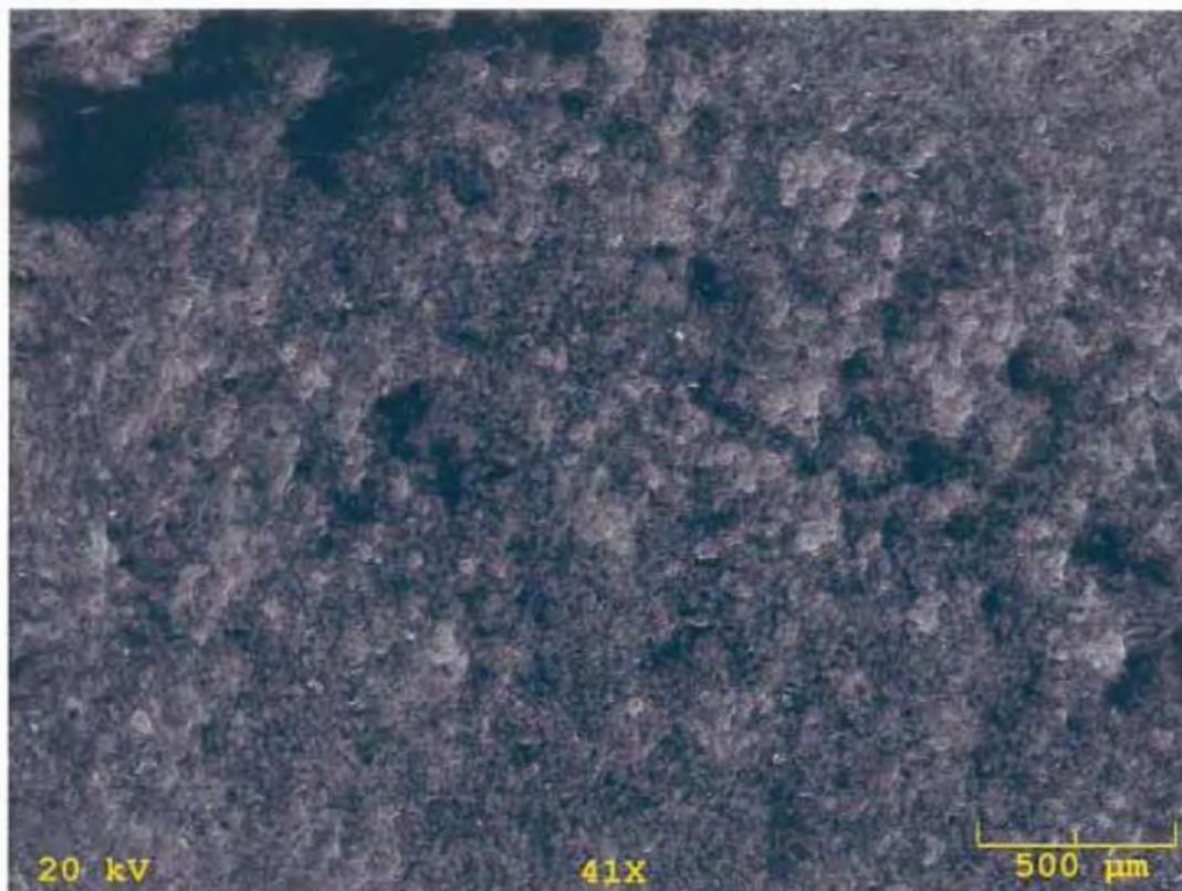
**Fig. 32 S.E.M photo of failed support rod from east span at fracture origin. Zone 2. 41X.**
