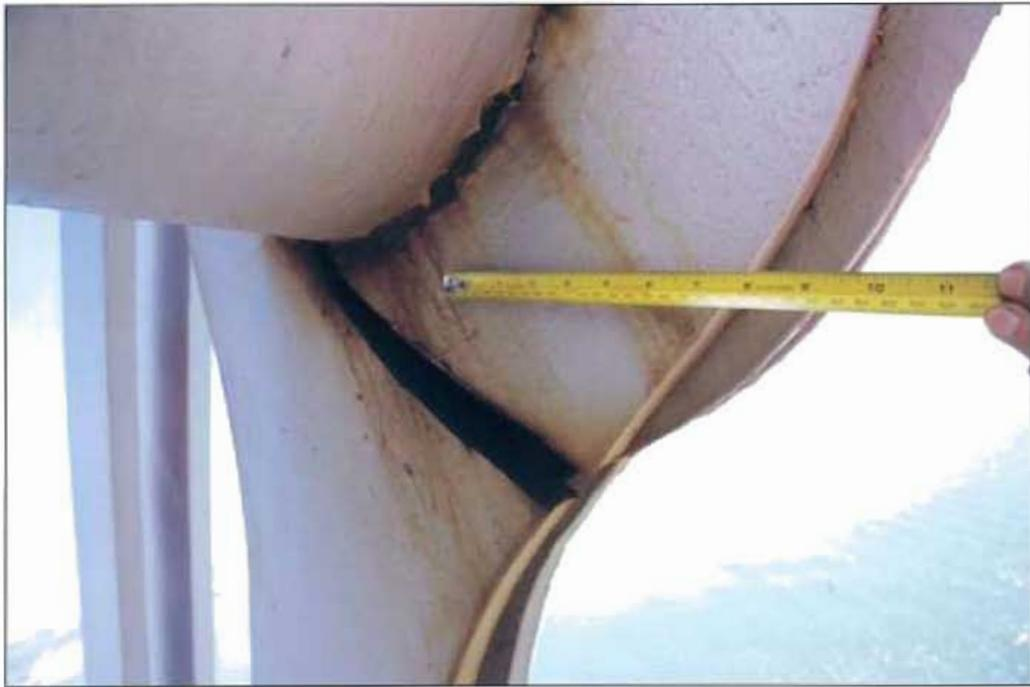
**Fig. 3 Location of cracked eye bar.**
