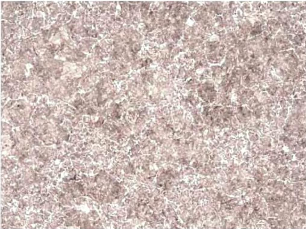
**Fig. 103** Longitudinal microsection of eye bar near the center pin location, in fig. 98, location A, showing core microstructure. 50X.Etched.
