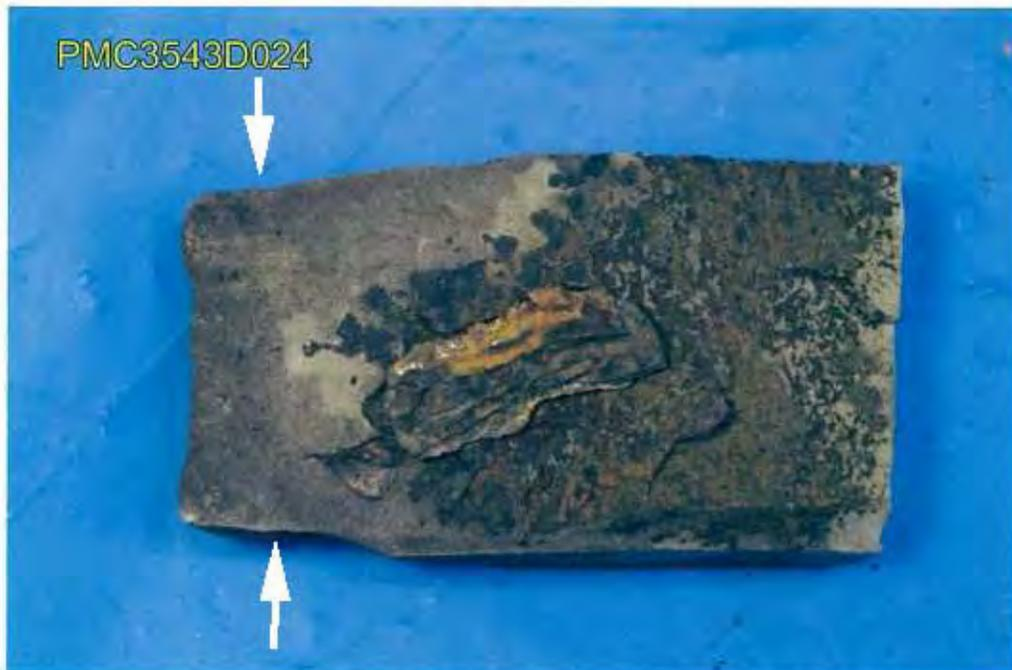
**Fig. 44** Fracture face of eye bar outboard from pin location, after cleaning of oxide layer.
