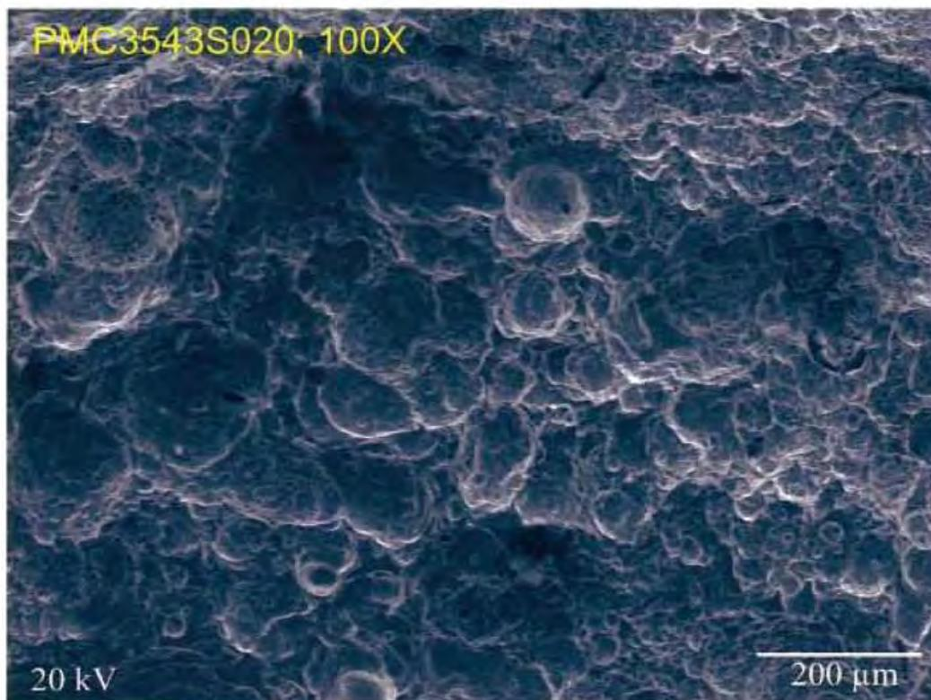
**Fig. 64 S.E.M photo of eye bar fracture surface, 2nd segment in fig. 35 at location 2, left edge. 100X.**
