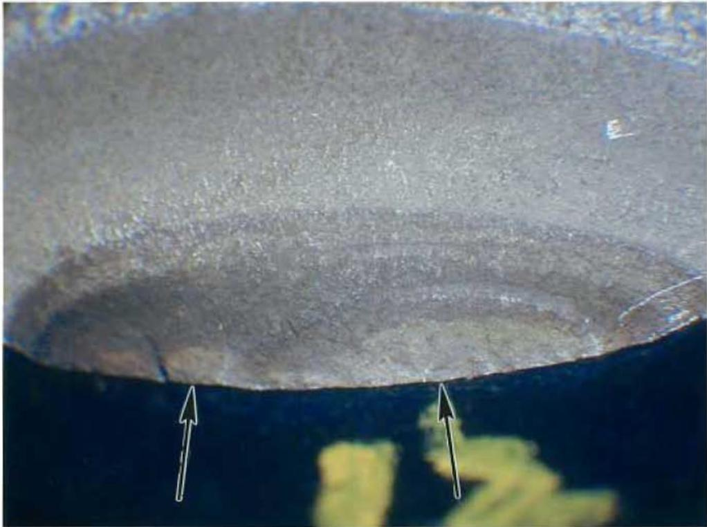
Fig. 18 As received failed support rod from east span. Fracture origin.
