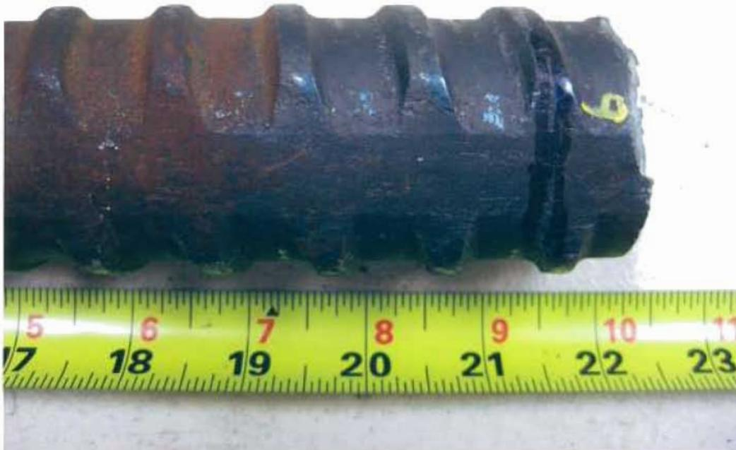
**Fig. 9 As received failed support rod from east span. 9 O'clock position.**
