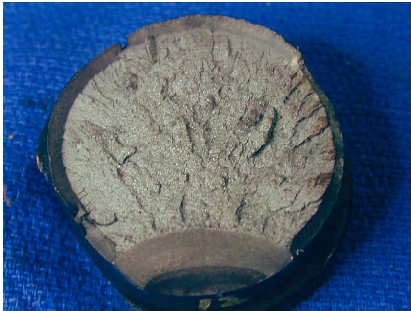
**Figure 12: Fracture surface of failed support rod.**
