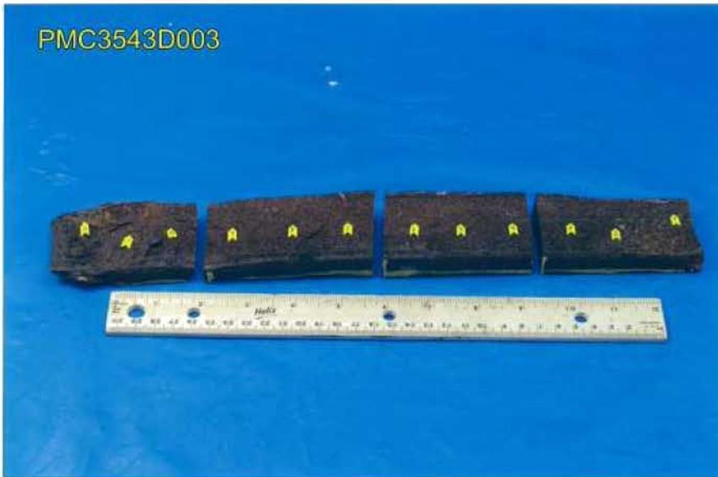
**Fig. 23 Fracture face of eye bar, upper portion. Arrows indicate E.D.S analyses locations.**
