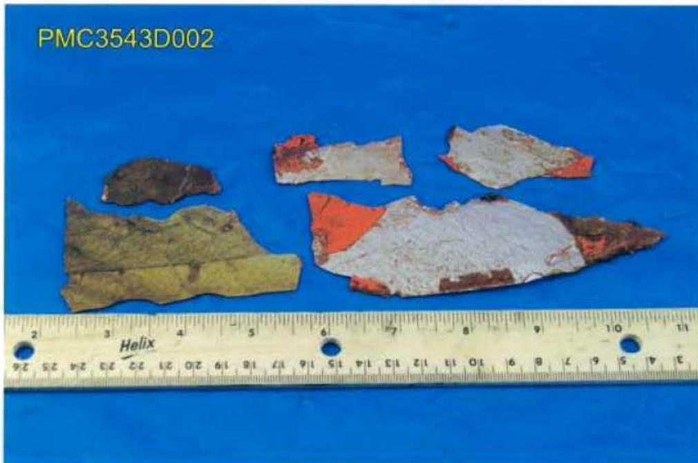
**Fig. 22 Paint chip samples from eye bar.**
