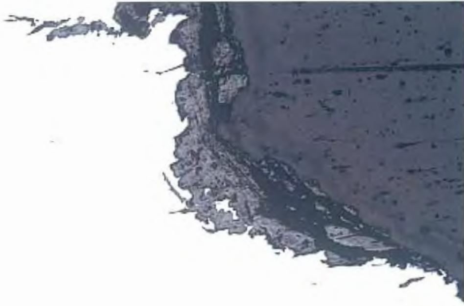
**Fig. 93** Transverse cross-section made of eye bar near the center pin location, showing fracture face and scale. 100X.
