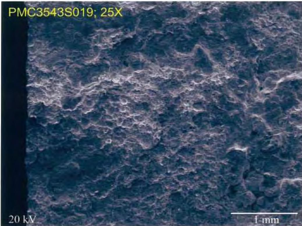
**Fig. 63 S.E.M photo of eye bar fracture surface, 2nd segment in fig. 35 at location 2, left edge. 25X.**
