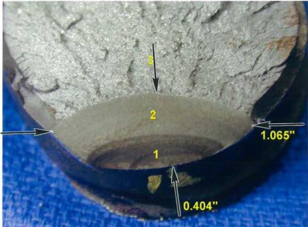
Fig. 17 As received failed support rod from east span. Fracture origin.
