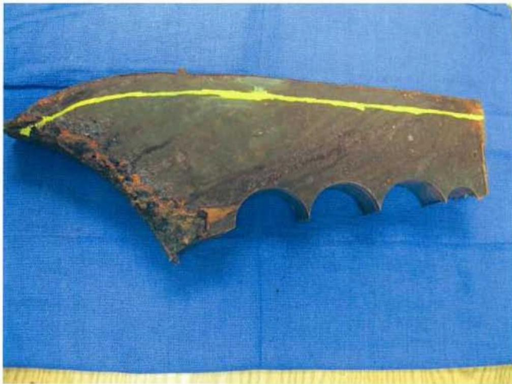
**Fig. 16 Cut location to remove fracture face.**
