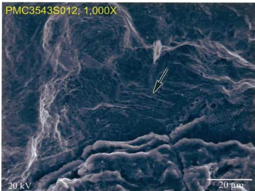
**Fig. 52 S.E.M photo of eye bar fracture surface at fracture origin, in fig. 45. 1000X.**
