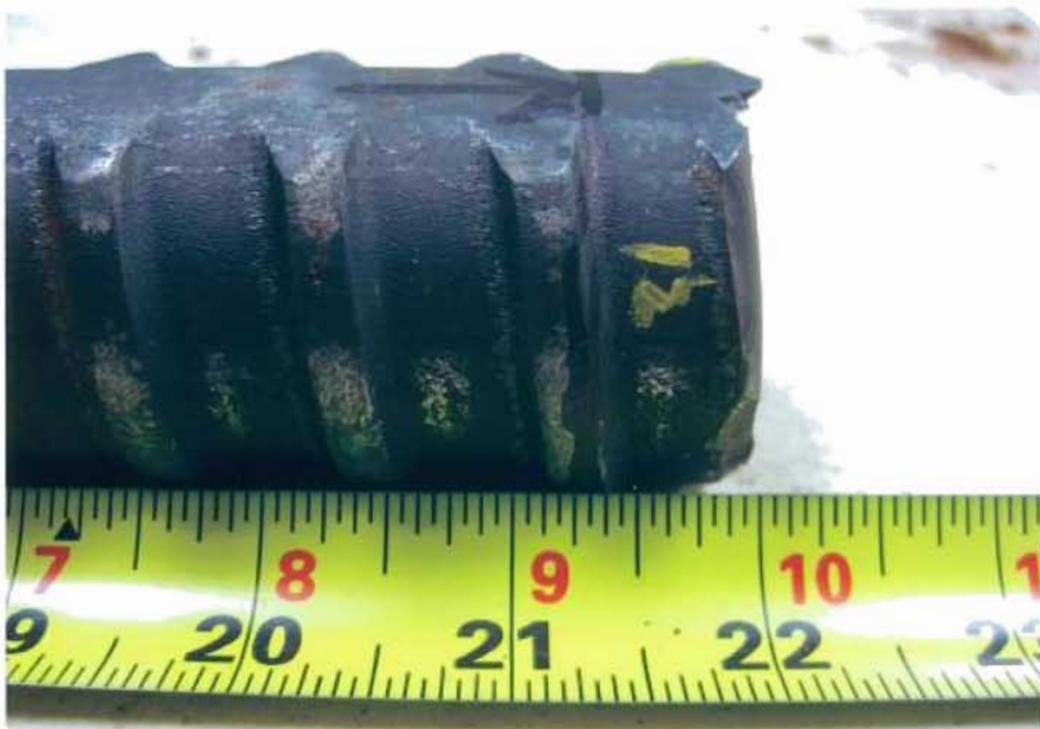
Fig. 3 As received failed support rod from east span. 12 O'clock position, fracture origin.
