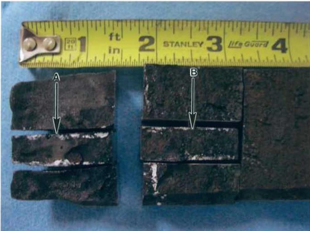
**Fig. 98** Location where longitudinal microsections were made of eye bar near the center pin location.
