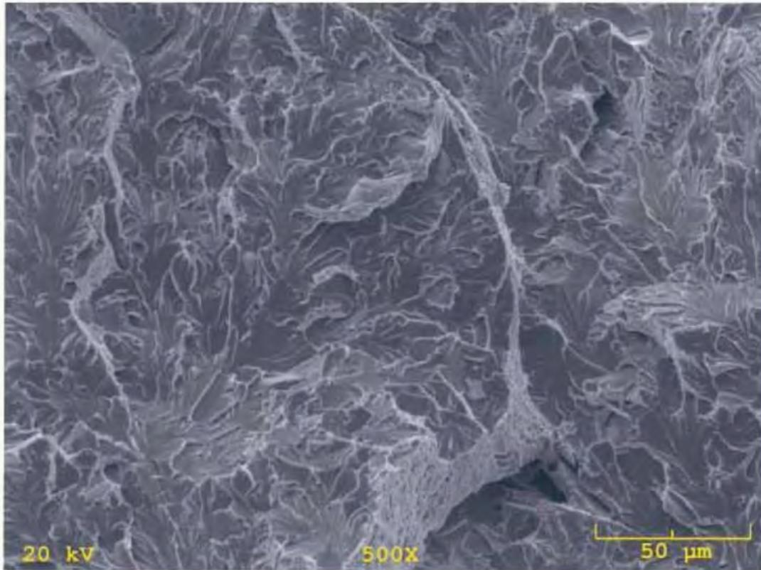
Fig. 41 S.E.M photo of failed support rod from east span 3/4 across on fracture surface. 500X.
