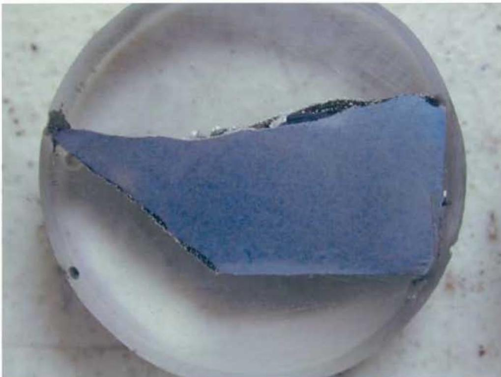
**Fig. 100** Longitudinal microsection of eye bar near the center pin location, in fig. 98, location A.
