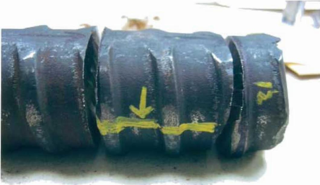
**Fig. 15** As received failed support rod from east span. Location where longitudinal microsection was made.
