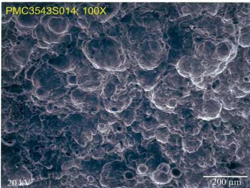
**Fig. 58 S.E.M photo of eye bar fracture surface, 2nd segment in fig. 35 at location 2, right edge. 100X.**
