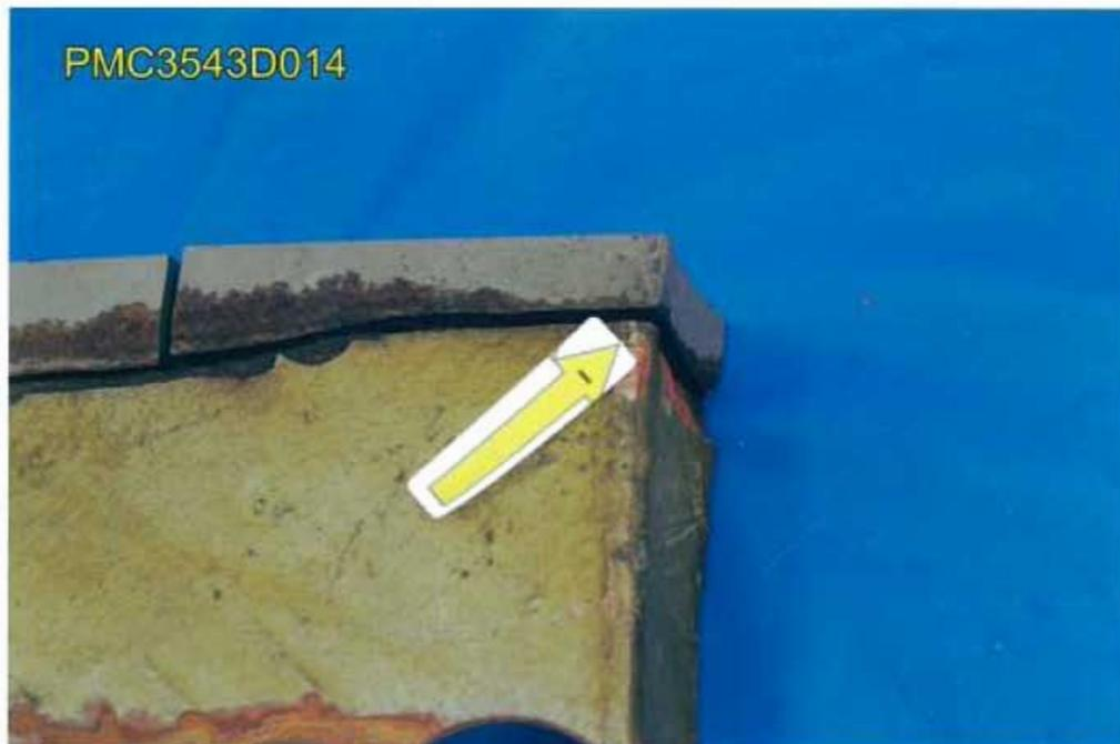
**Fig. 34 Outer edge of fracture. Arrow pointing to fracture origin.**
