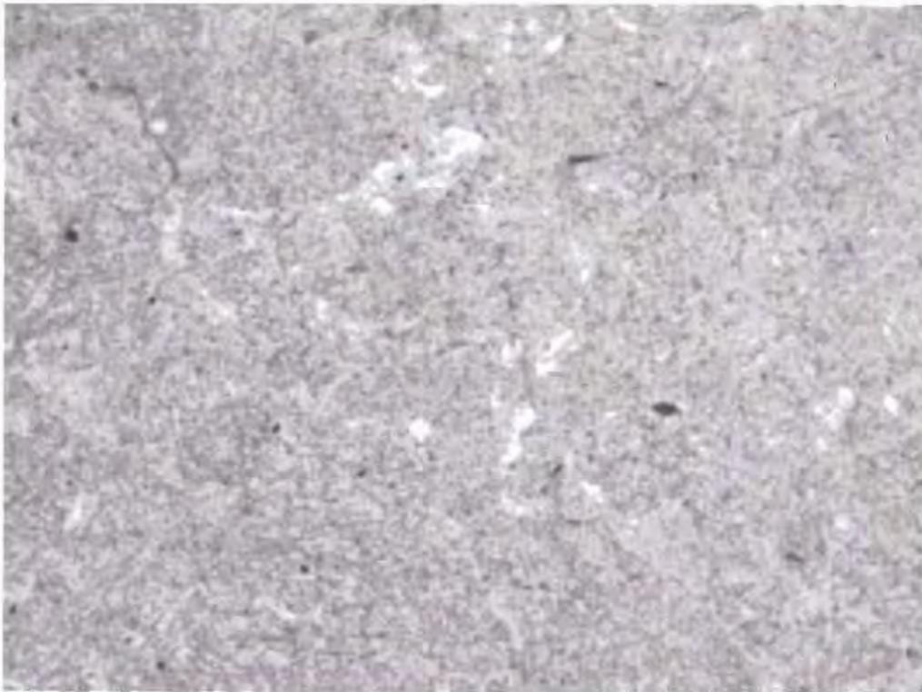
**Fig. 72 Microstructure near top corner sample #1 in fig. 71. 200X Etched.**
