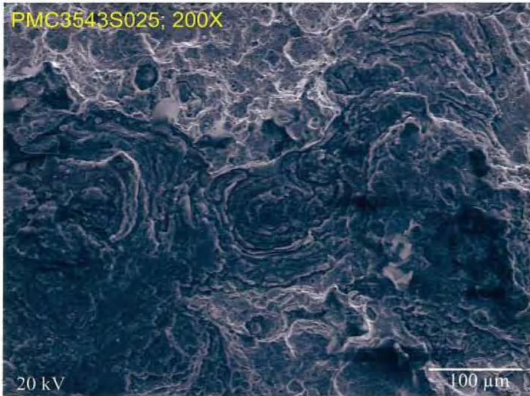
**Fig. 69 S.E.M photo of eye bar fracture surface, 4th segment in fig. 35 at location 4, oxide on Fracture face, area 3. 200X.**
