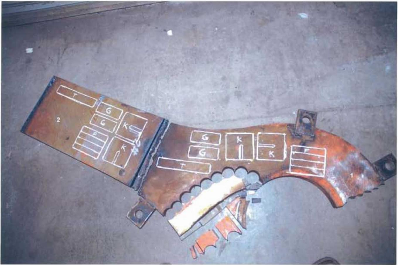
**Fig. 106 Test plan for mechanical properties from eye bar segments 1 and 2**
