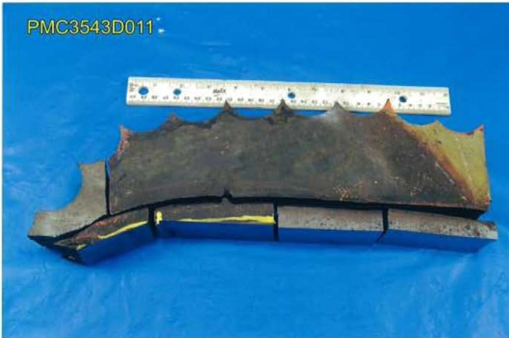
Fig. 31 Overall photo of upper portion of fracture and lower portion of fracture. Opposite side.
