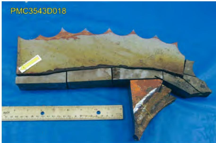
**Figure 7: Upper and lower portion of fractured eye bar. Fracture origin at arrow location.**
