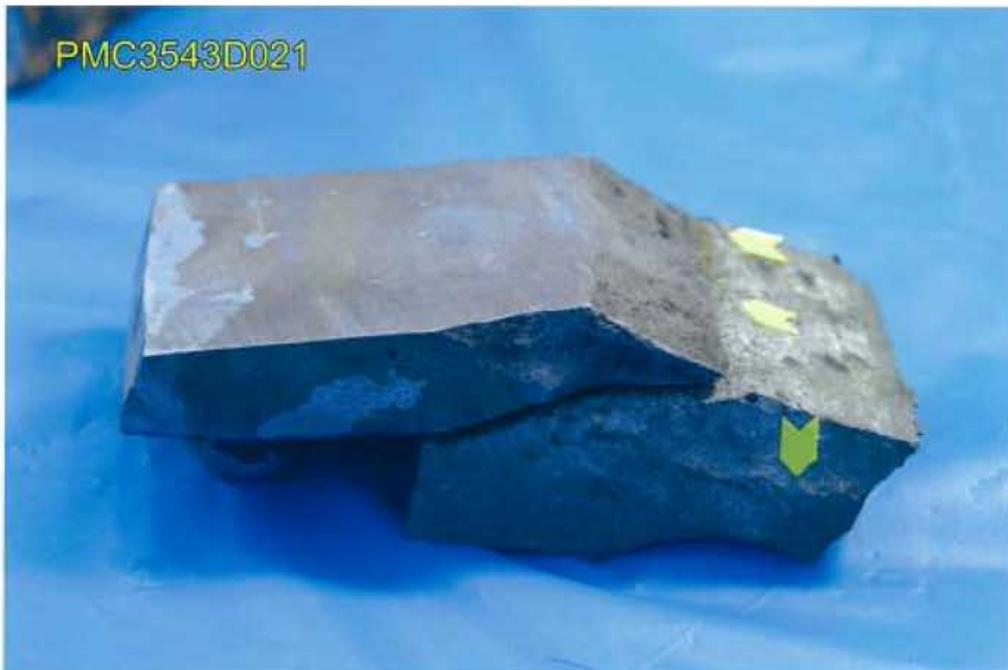
**Fig. 41** Inside diameter surface of eye bar pin location, after cleaning of oxide layer.
