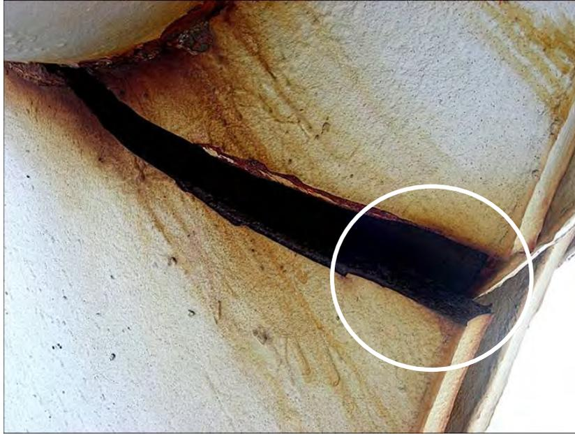
Figure 3: Failure initiation location is circled above and highlighted in following figures.
