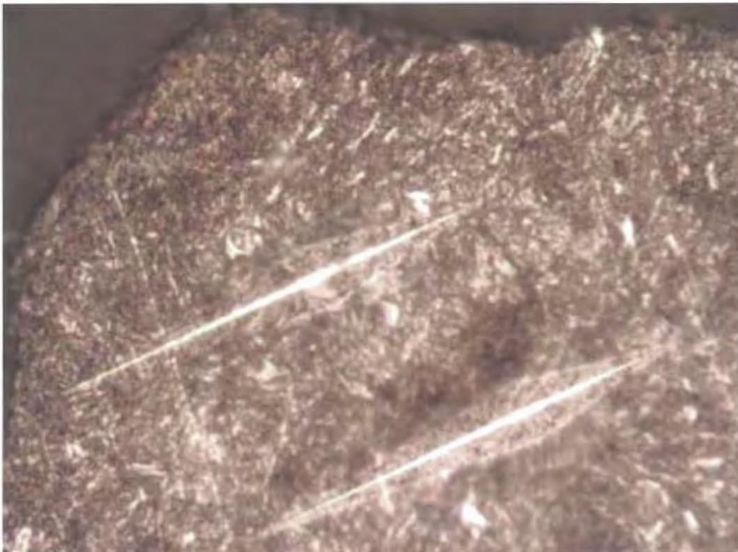
**Fig. 50** Cross-section of failed support rod from east span at fracture origin in fig. 16. 500X. Etched.
