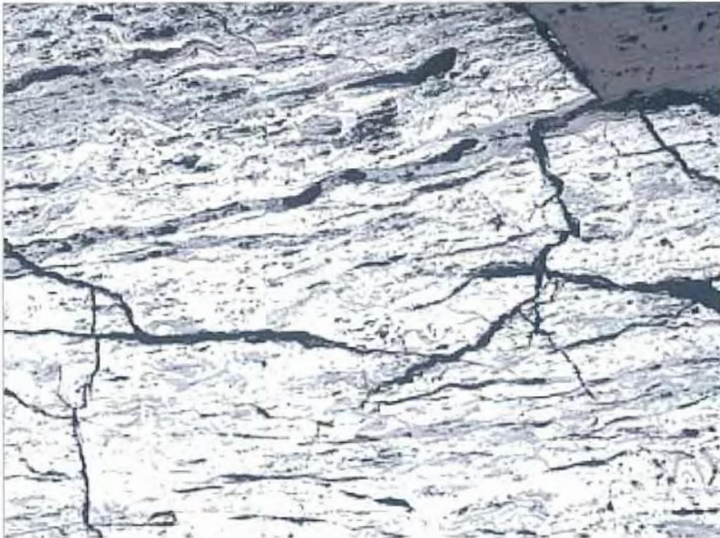
**Fig. 94** Transverse cross-section made of eye bar near the center pin location, showing scale. 100X.
