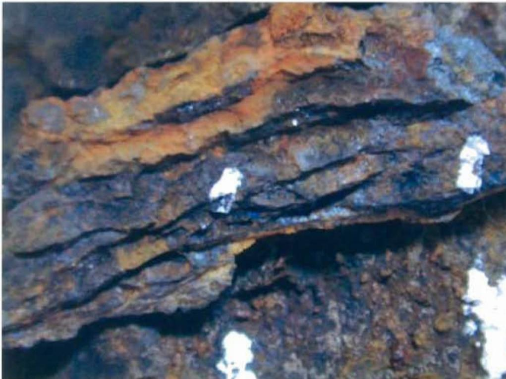
**Fig. 90** Scale on fracture surface of eye bar near the center pin location.
