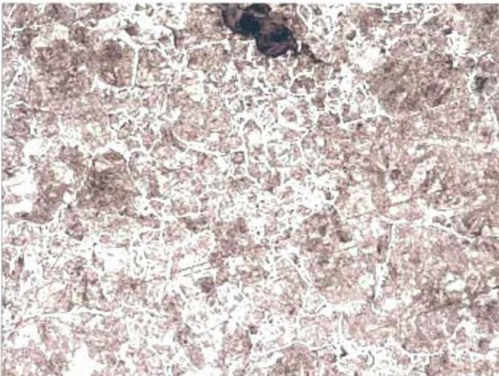
**Fig. 102** Longitudinal microsection of eye bar near the center pin location, in fig. 98, location A, below fracture surface. 200X. Etched.
