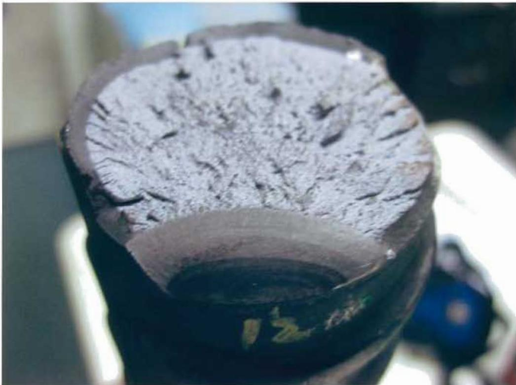
**Fig. 11 As received failed support rod from east span. Fracture sureface.**
