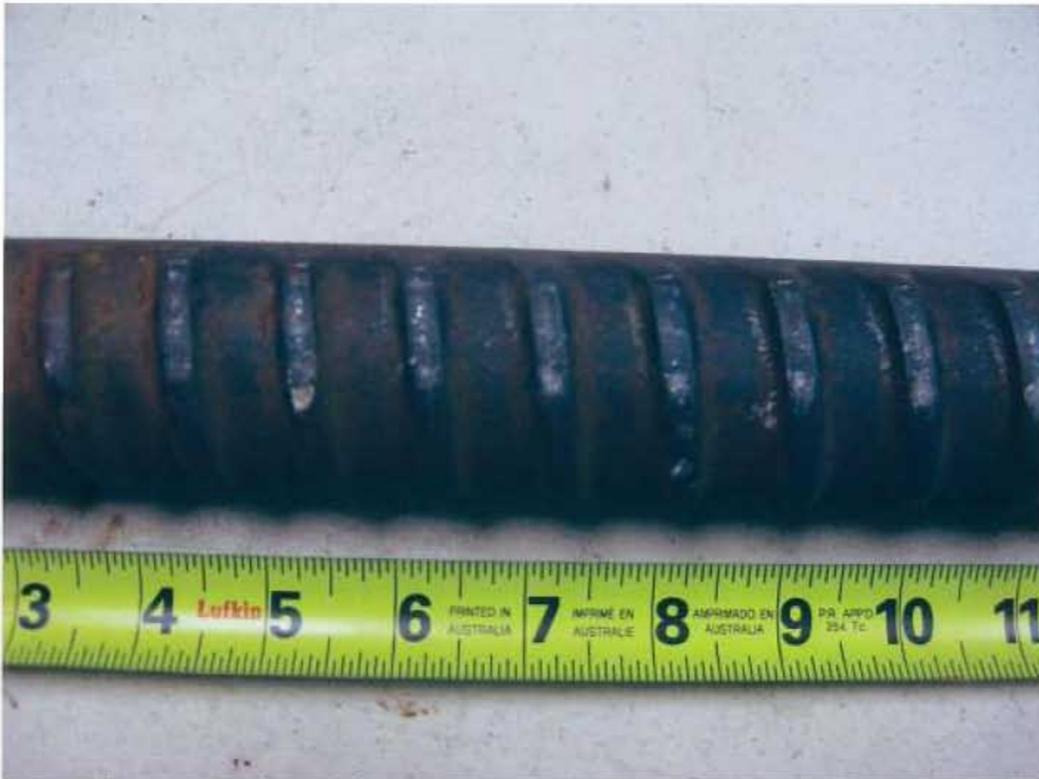
**Fig. 5** As received failed support rod from east span. 12 O'clock position.
