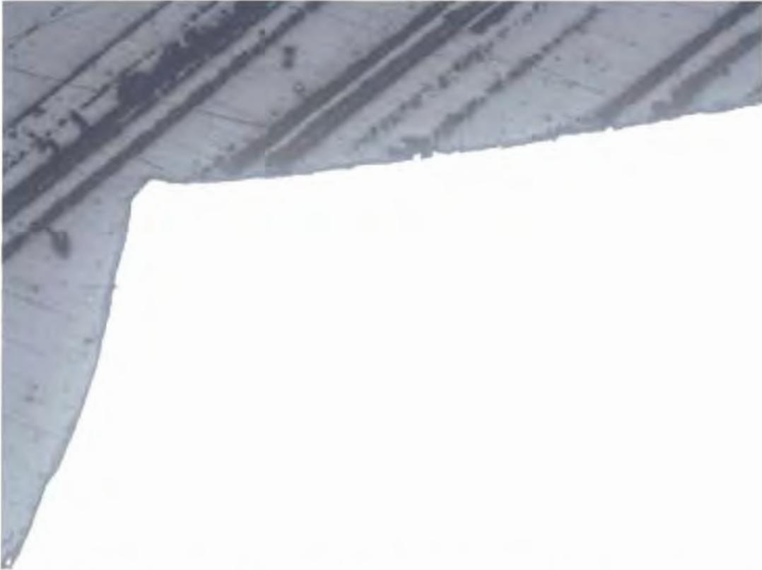
**Fig. 47** Cross-section of failed support rod from east span at fracture origin in fig. 16. 50X.
