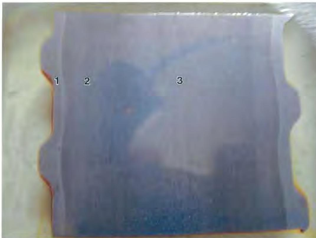
**Fig. 43** Longitudinal cross-section of failed support rod from east span.
