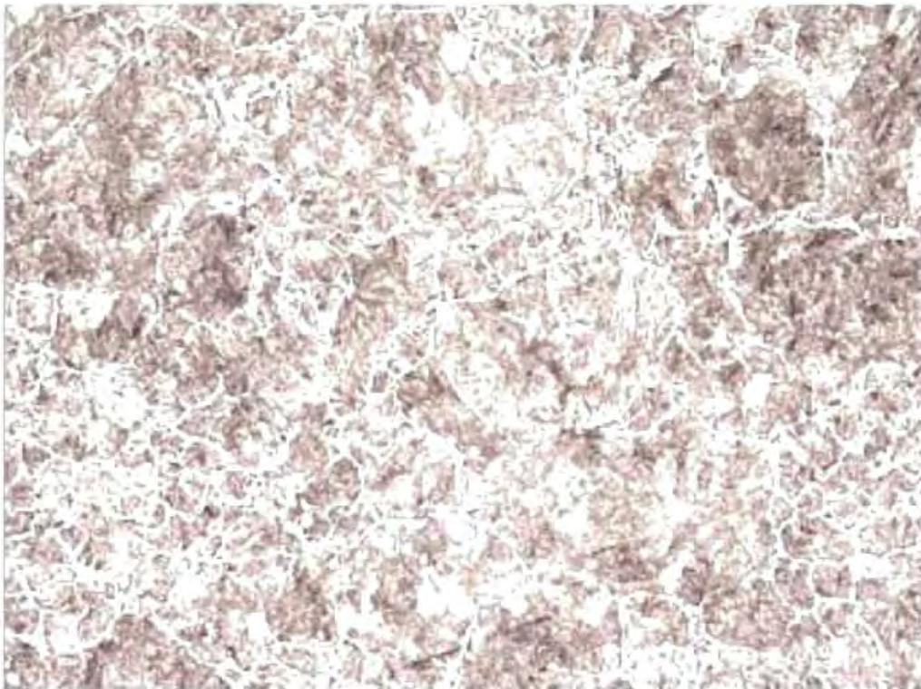
**Fig. 104** Longitudinal microsection of eye bar near the center pin location, in fig. 98, location A, showing core microstructure. 200X.Etched.
