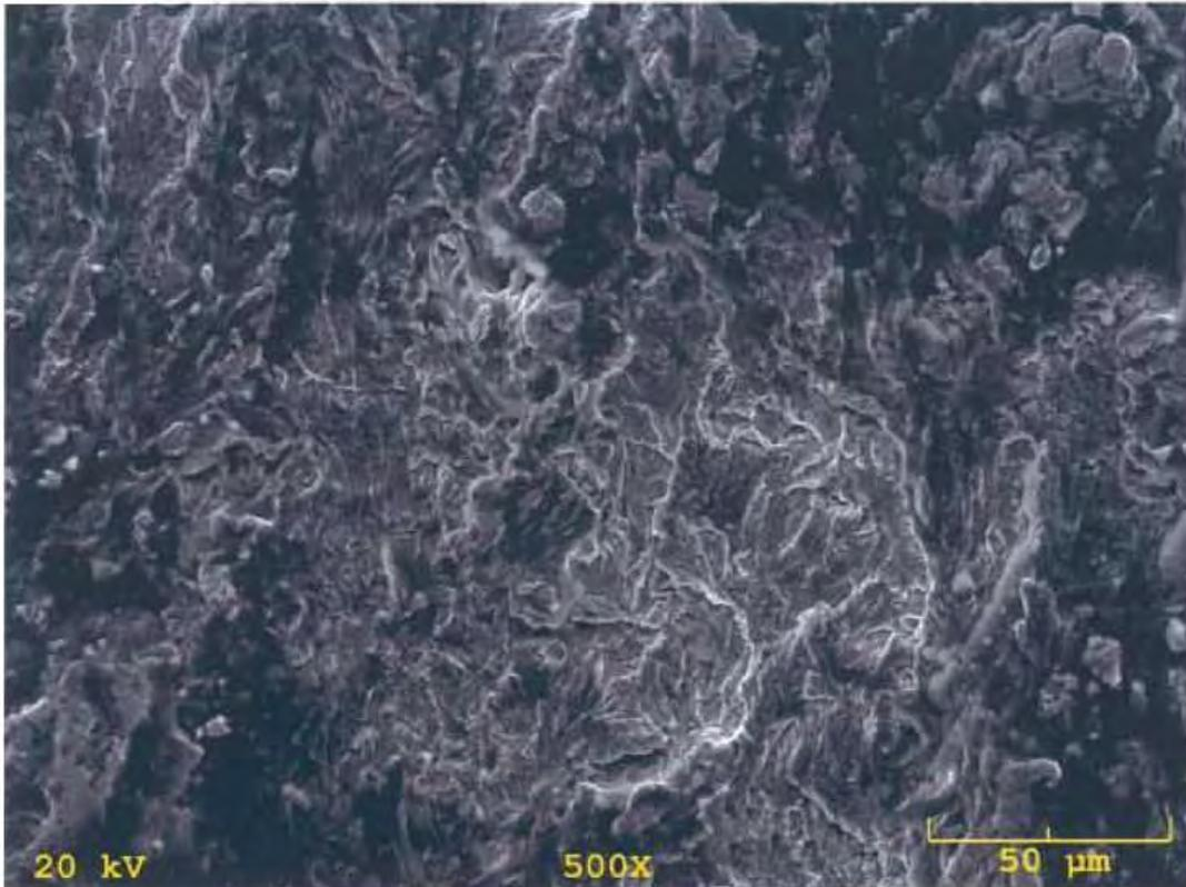
**Fig. 33 S.E.M photo of failed support rod from east span at fracture origin. Zone 2. 500X.**
