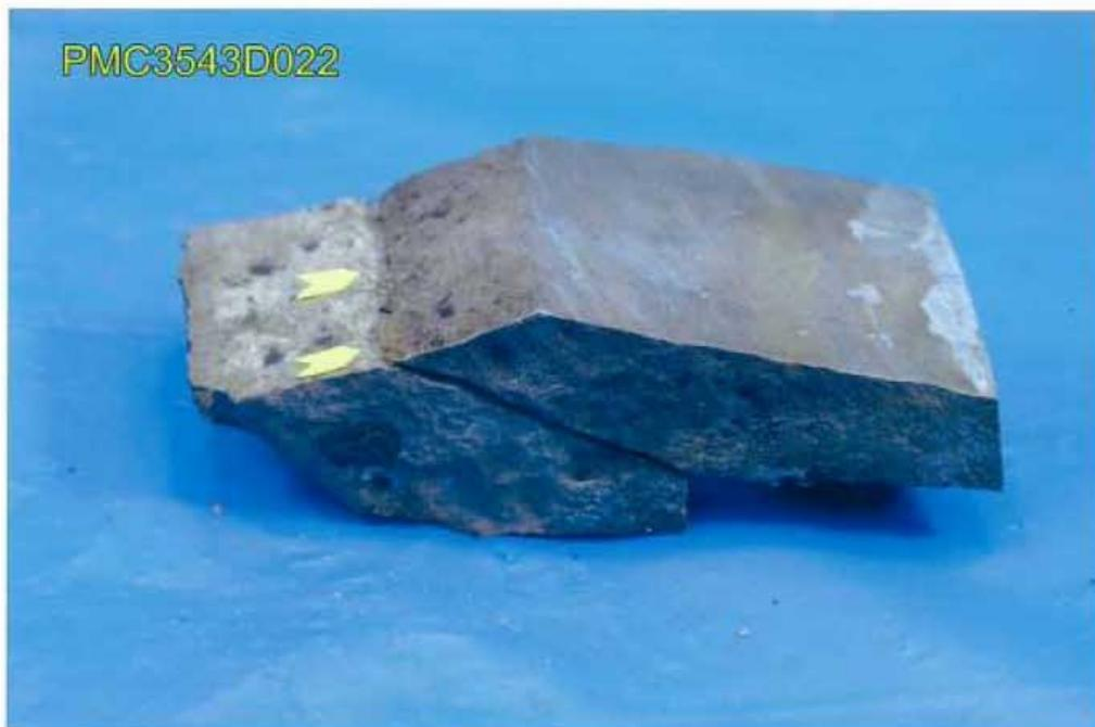
**Fig. 42** Inside diameter surface of eye bar pin location, after cleaning of oxide layer.
