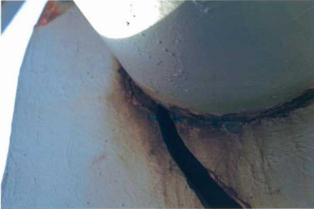
**Fig. 9 Fracture at sleeve location.**
