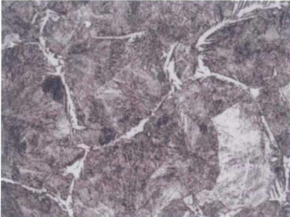
**Fig. 75 Core microstructure of sample # 1 in fig. 71. 500X Etched.**
