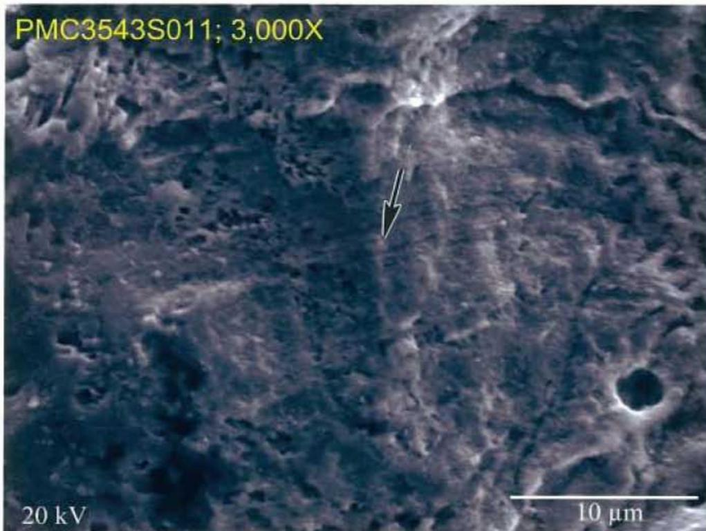
**Fig. 51 S.E.M photo of eye bar fracture surface at fracture origin, in fig. 50. 3,000X**
