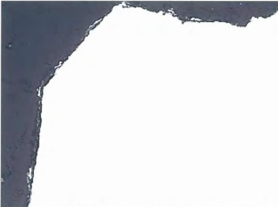
**Fig. 48** Cross-section of failed support rod from east span at fracture origin in fig. 16. 500X.
