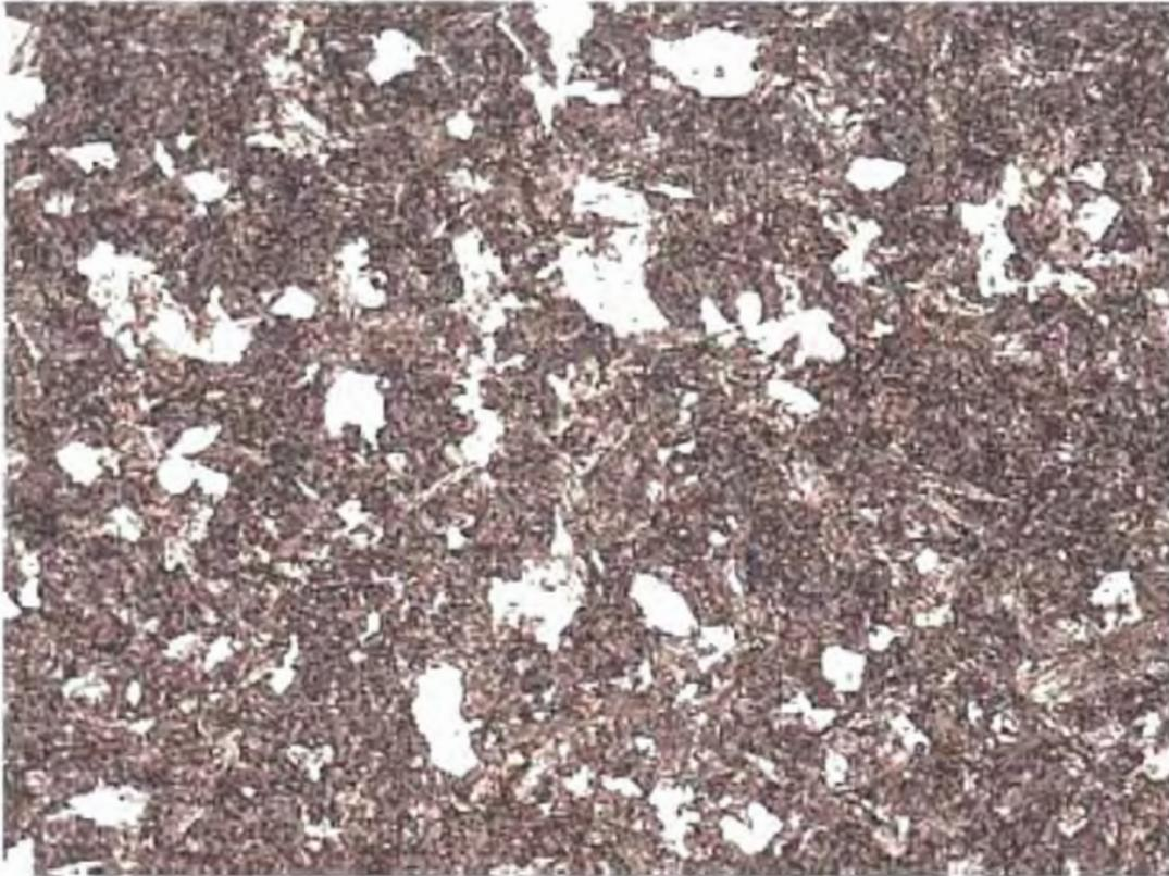
**Fig. 45** Longitudinal cross-section of failed support rod from east span. Microstructure at location 2 in fig. 43. 500X. Etched.
