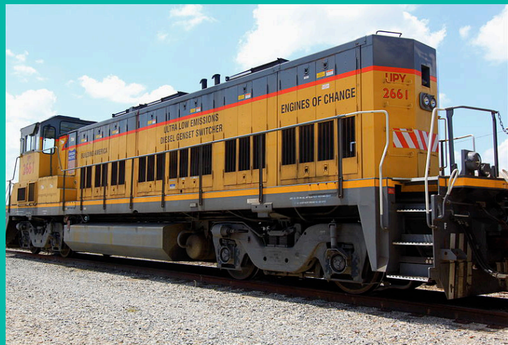
Ultra-low emissions switching locomotive (Source: flickr, Roy Luck, https://commons.wikimedia.org/wiki/File:Union_Pacific_Genset_switcher,_Eureka_Yard.jpg )
