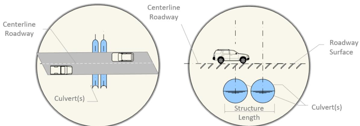
Note: Culvert structure length under 20 feet is classified as a culvert. Over 20 feet is classified as a bridge
