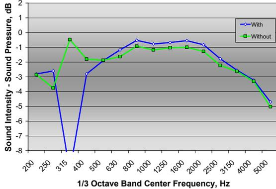
Figure 14: Comparison of 1/3 octave band differences between SI and SPL levels with and without nose cones for a windscreen protected probe measured on PCC pavements on the Mojave Bypass
