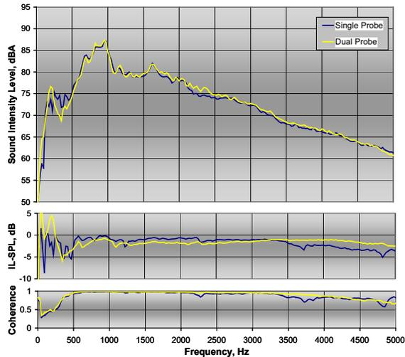
Figure 33: Comparison single and dual probe SI averages of multiple runs on ARFC for the Trailing edge of the tire contact patch
