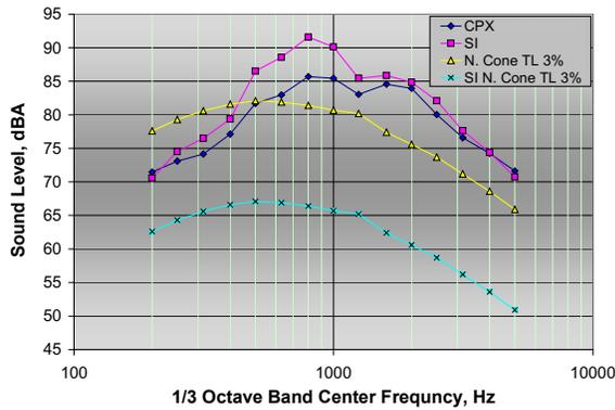
Figure 11: Comparison of the flow induced background noise for SPL and IL using nose cones with a 3% turbulence level relative to CPX & SI tire/pavement noise
