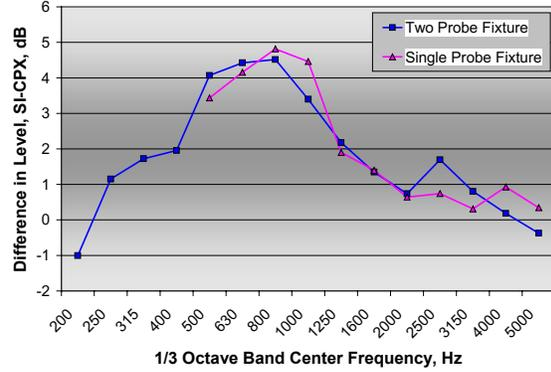
Figure 22: Comparison of averages of differences in 1/3 octave band levels between SI and CPX measurements made with the ADOT CPX trailer using single and dual probe fixtures
