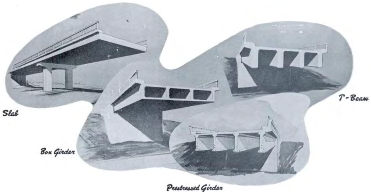
Figure 11: Concrete Bridge Types, Division of Highways Bridge Planning and Design Manual, September 1958.
