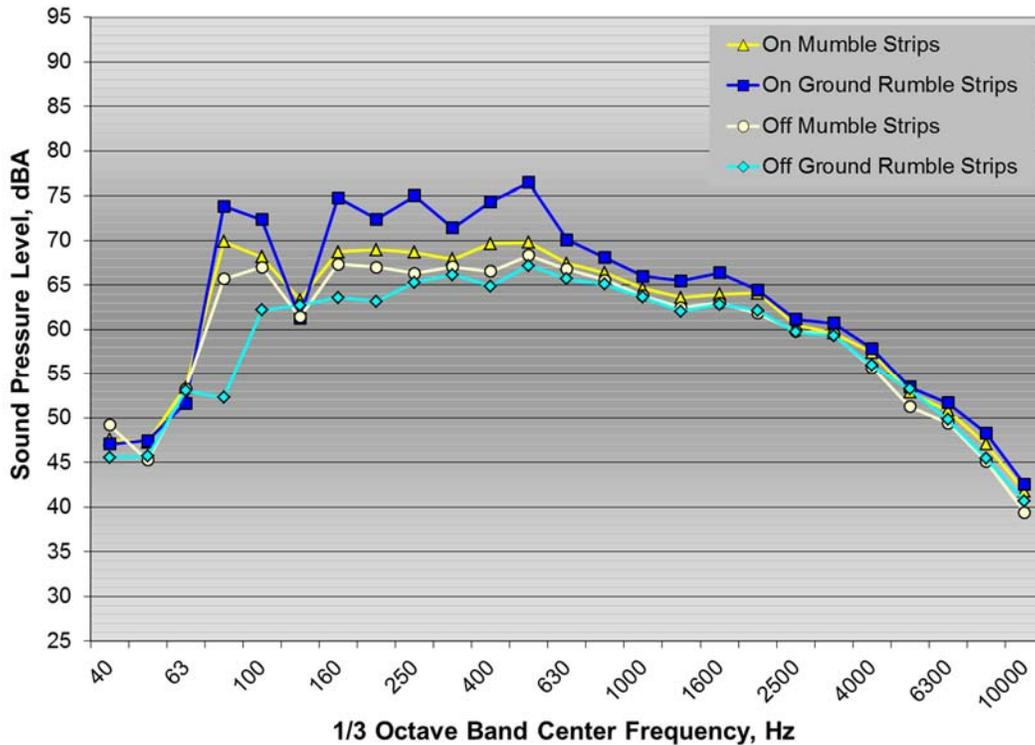
Figure 39: 1/3 octave band interior noise spectra for 4-yard dump truck test vehicle on and off mumble strips and ground rumble strips
