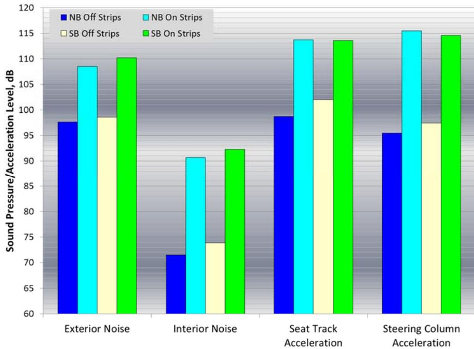
**Figure A7: Overall noise and acceleration levels for Malibu test vehicle traveling at 60 mph both on and off mumble strips and both northbound and southbound**
