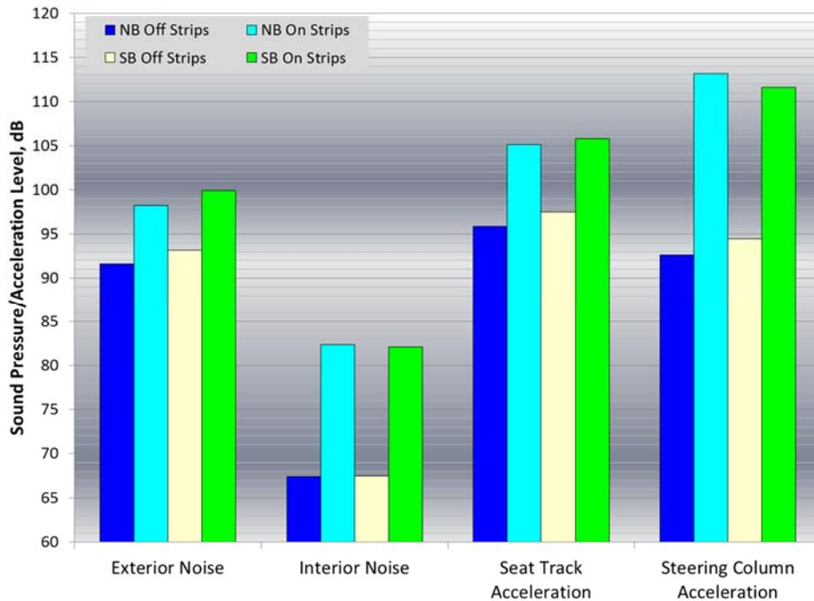
**Figure A9: Overall noise and acceleration levels for Malibu test vehicle traveling at 40 mph both on and off mumble strips and both northbound and southbound**
