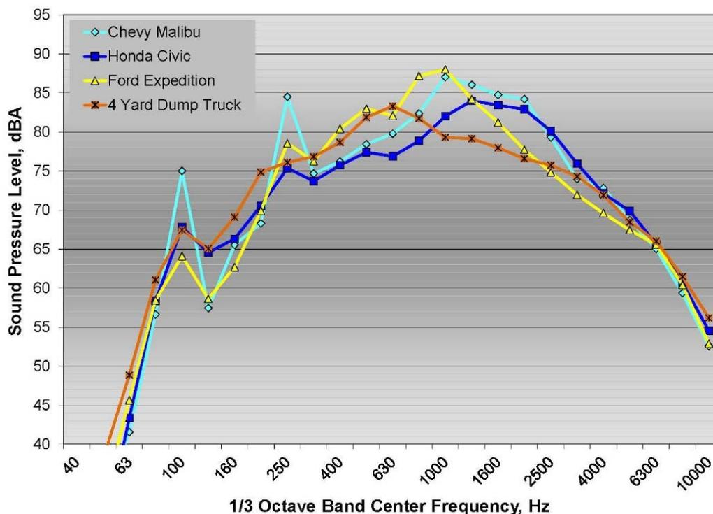
Figure 30: 1/3 octave band pass-by spectra on dots for four test vehicles
