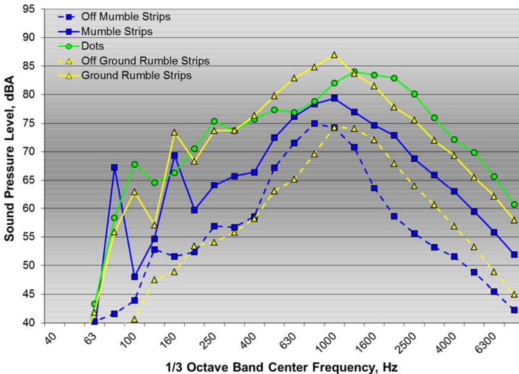
Figure 24: 1/3 octave band pass-by spectra for Civic test vehicle on (solid lines) and off (dashed lines) mumble strips, dots, and ground rumble strips
