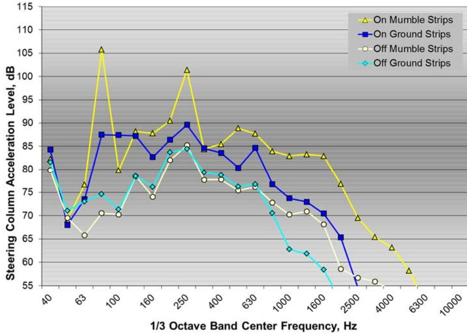
Figure A18:  $\frac{1}{3}$  octave band steering column acceleration spectra for Expedition test vehicle on and off mumble strips and ground rumble strips at 60 mph
