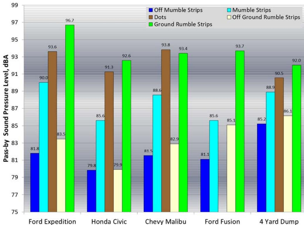
**Figure 22: Overall A-weighted pass-by sound pressure levels for all four test vehicles on three types of warning devices**
