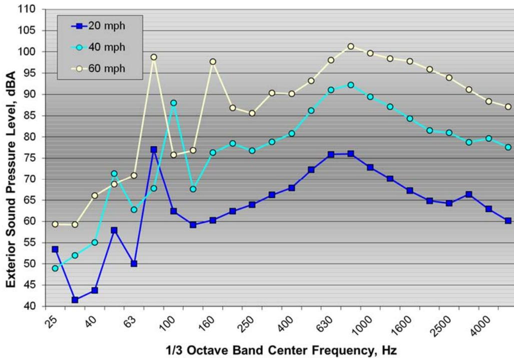
Figure 49: 1/3 octave band on-board exterior noise spectra on mumble strips for the Malibu test vehicle at 20, 40, and 60 mph
