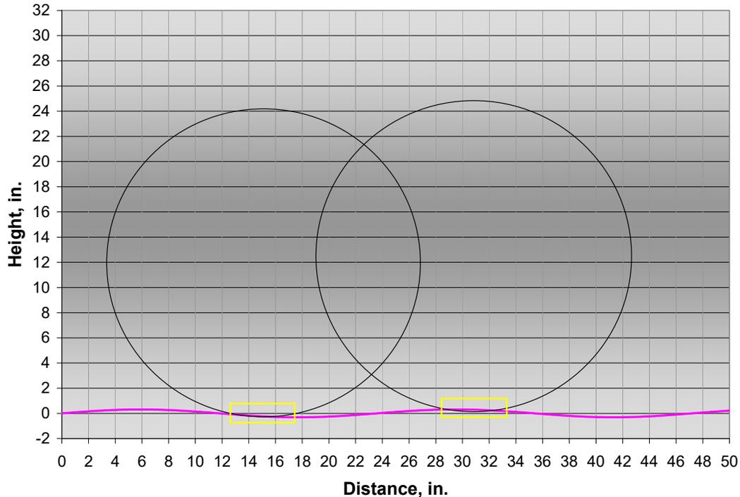
**Figure 4: Relative geometries of typical passenger car tire, tire contact patch length, and exaggerated rumble strip profiles of  $\lambda=23.6$  inches**
