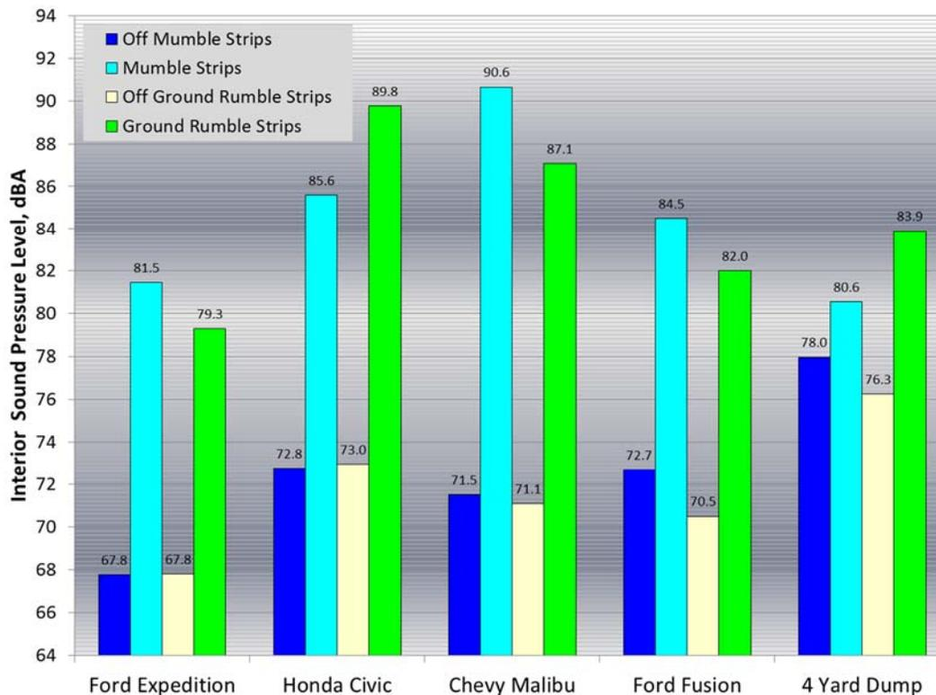
**Figure 34: Overall A-weighted interior sound pressure levels for all four test vehicles on and off mumble and ground rumble strips**
