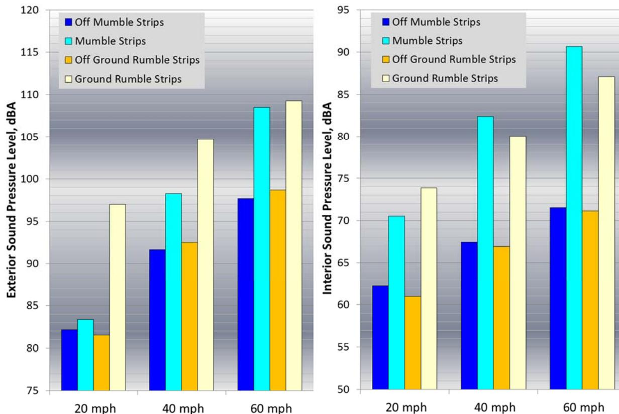
**Figure 48: Overall A-weighted on-board exterior (left) and interior (right) sound pressure levels for Malibu test vehicle on and off mumble strips and ground rumble strips at 20, 40, and 60 mph**
