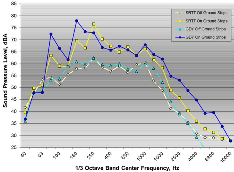
Figure A26: 1/3 octave band interior noise spectra for Ford Fusion test vehicle on and off ground rumble strips with SRTT and Goodyear test tires
