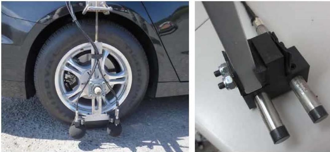
**Figure 67: Modified OBSI fixture for rumble strip and mumble strip measurements installed (left) and with added probe holder isolation (right)**
