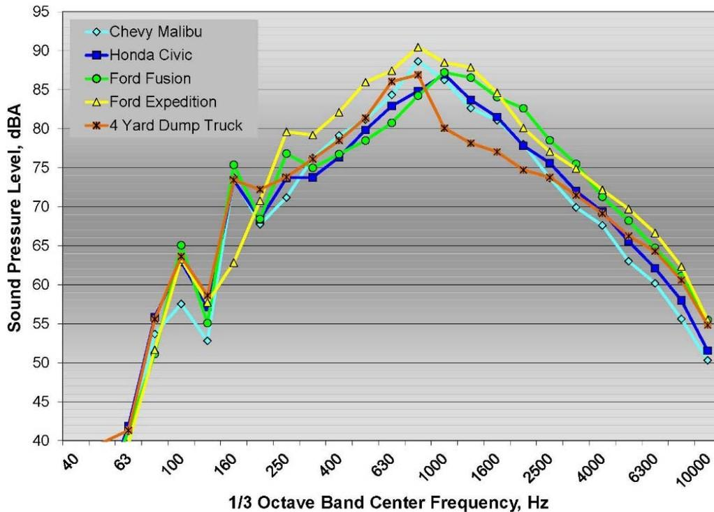
**Figure 29: 1/3 octave band pass-by spectra on ground rumble strips for all five test vehicles**
