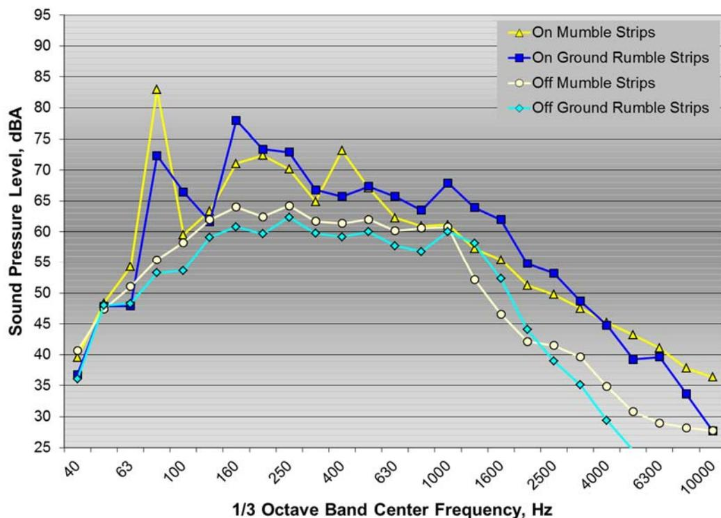
Figure 37: 1/3 octave band interior noise spectra for Fusion test vehicle on and off mumble strips and ground rumble strips
