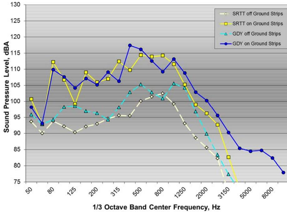
Figure A28: 1/3 octave band seat track acceleration spectra for Ford Fusion test vehicle on and off ground rumble strips with SRTT and Goodyear test tires
