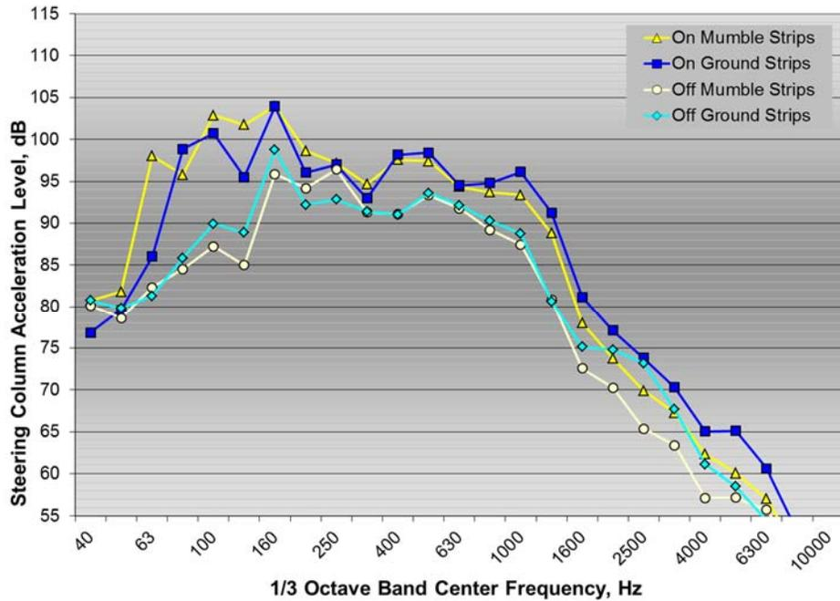
Figure A20: 1/3 octave band steering column acceleration spectra for 4-yard dump truck test vehicle on and off mumble strips and ground rumble strips at 60 mph
