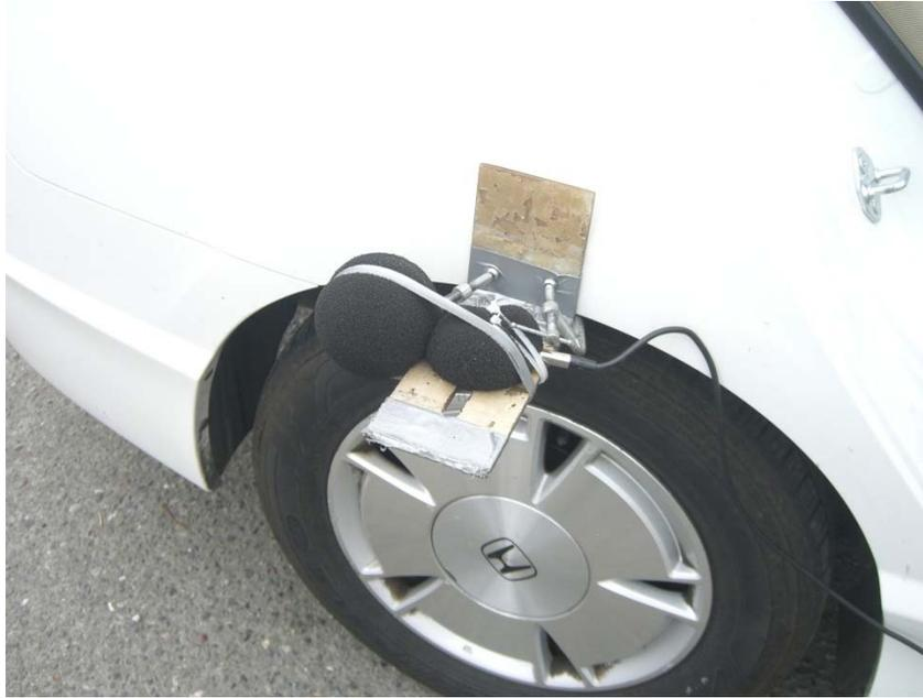
**Figure 14: Photograph of on-board microphone mounted above the wheel opening at the right rear tire of the Civic test vehicle**
