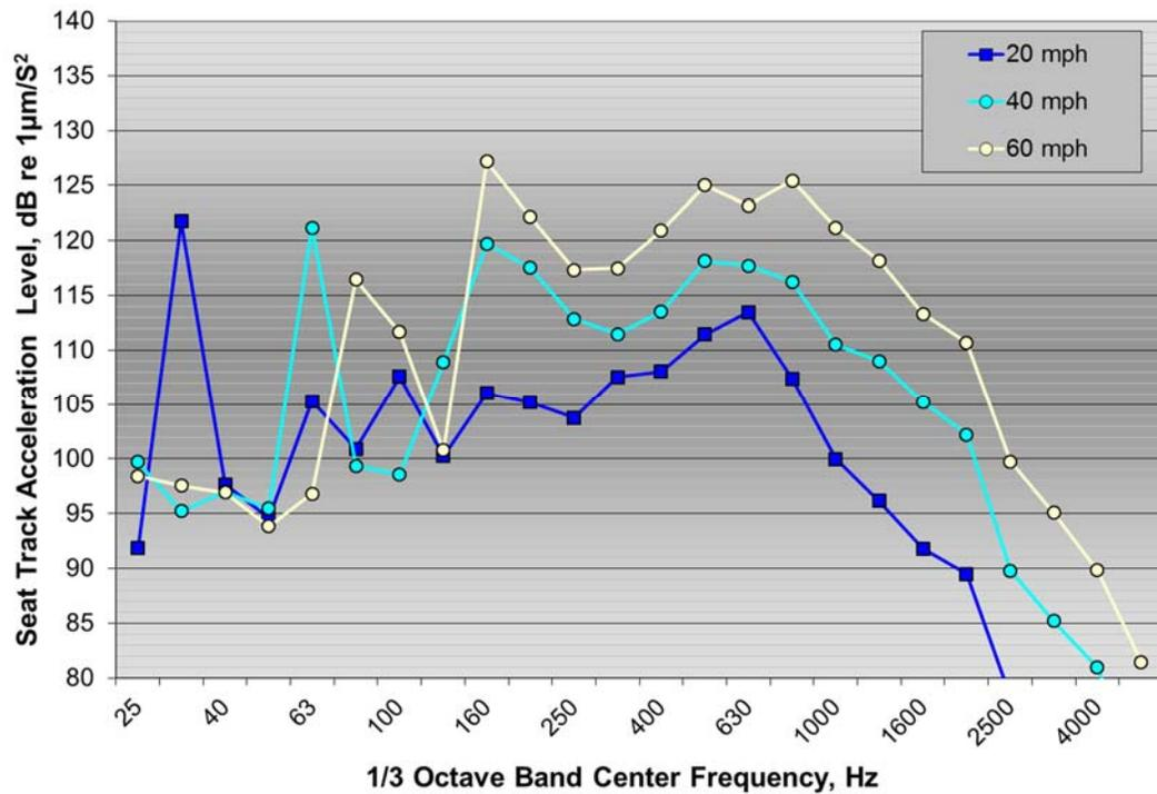
Figure 56: 1/3 octave band seat track acceleration level on ground rumble strips for the Malibu test vehicle at 20, 40, and 60 mph
