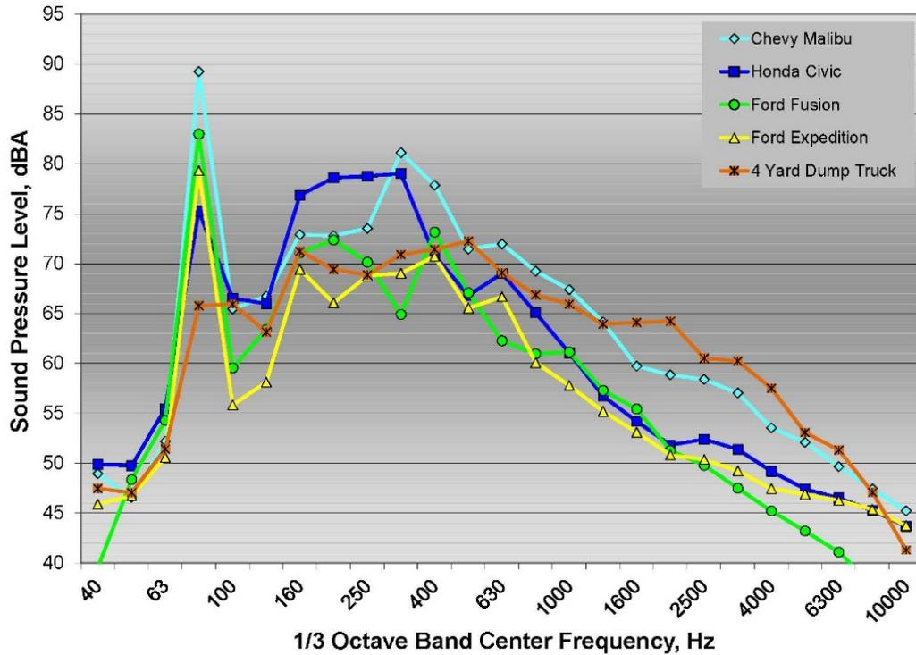
Figure 40: 1/3 octave band interior noise spectra for all five test vehicles on mumble strips
