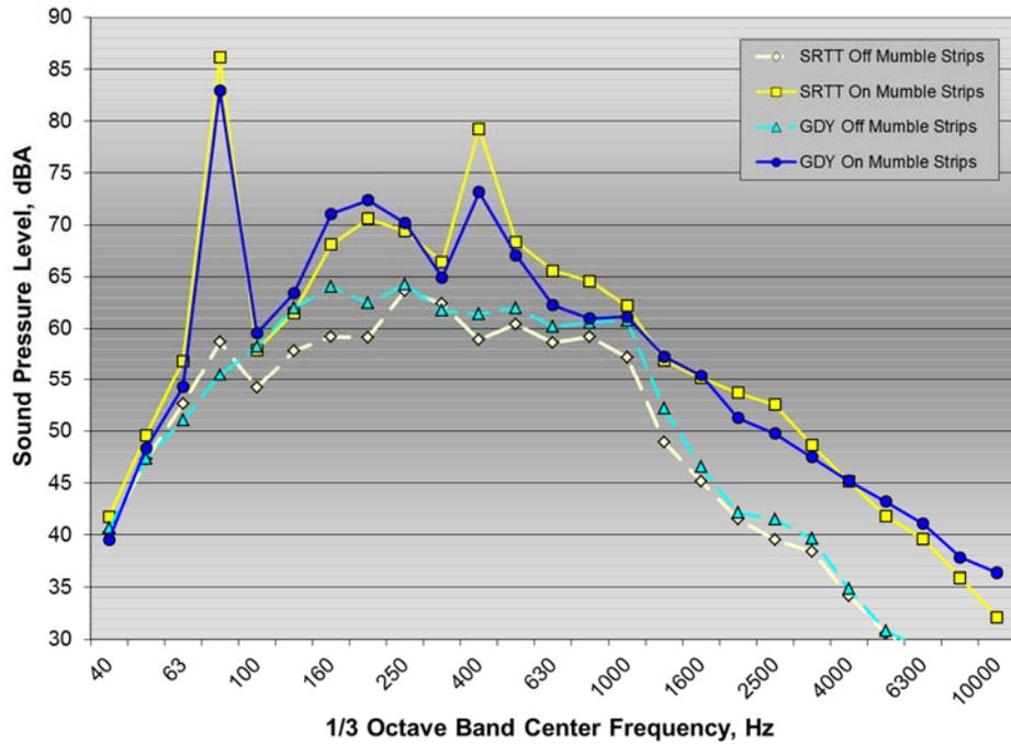
Figure A25: 1/3 octave band interior noise spectra for Ford Fusion test vehicle on and off mumble strips with SRTT and Goodyear test tires
