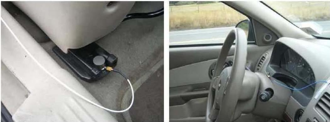
**Figure 16: Photographs of accelerometers mounted on the seat track (left) and the steering column (right) on the Malibu test vehicle**
