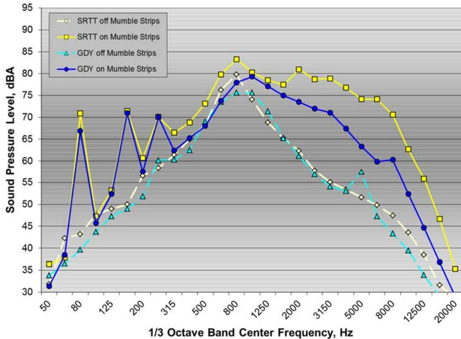
Figure A21: 1/3 octave band pass-by noise spectra for Ford Fusion test vehicle on and off mumble strips with SRTT and Goodyear test tires
