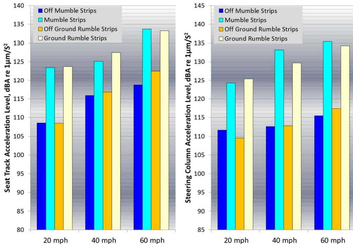
**Figure 53: Overall seat track (left) and steering column acceleration levels for Malibu test vehicle on and off mumble strips and ground rumble strips at 20, 40, and 60 mph**
