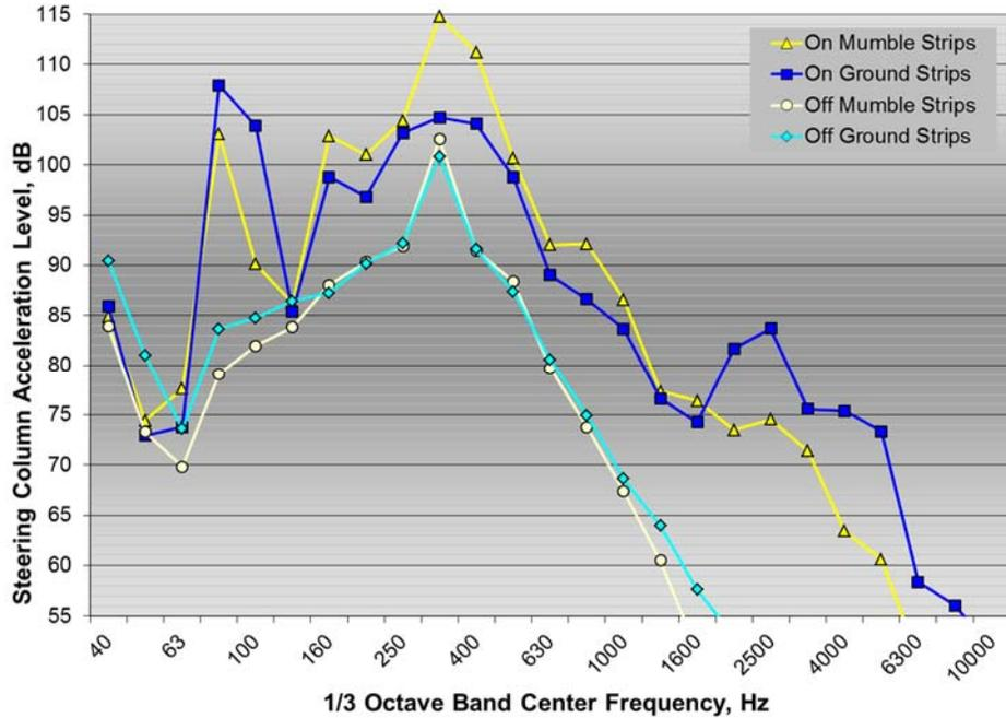
Figure A16: 1/3 octave band steering column acceleration spectra for Civic test vehicle on and off mumble strips and ground rumble strips at 60 mph
