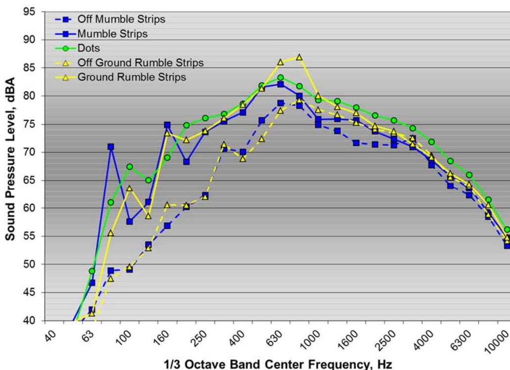
Figure 27:  $\frac{1}{3}$  octave band pass-by spectra for 4-yard dump truck test vehicle on (solid lines) and off (dashed lines) mumble strips, dots, and ground rumble strips
