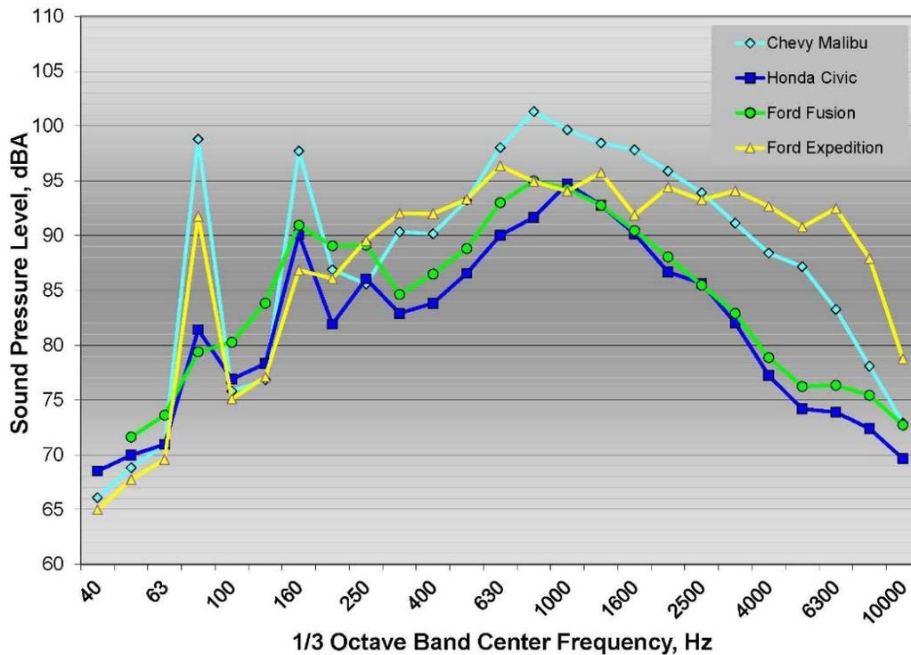
Figure 32: 1/3 octave band on-board exterior spectra on mumble strips for four test vehicles
