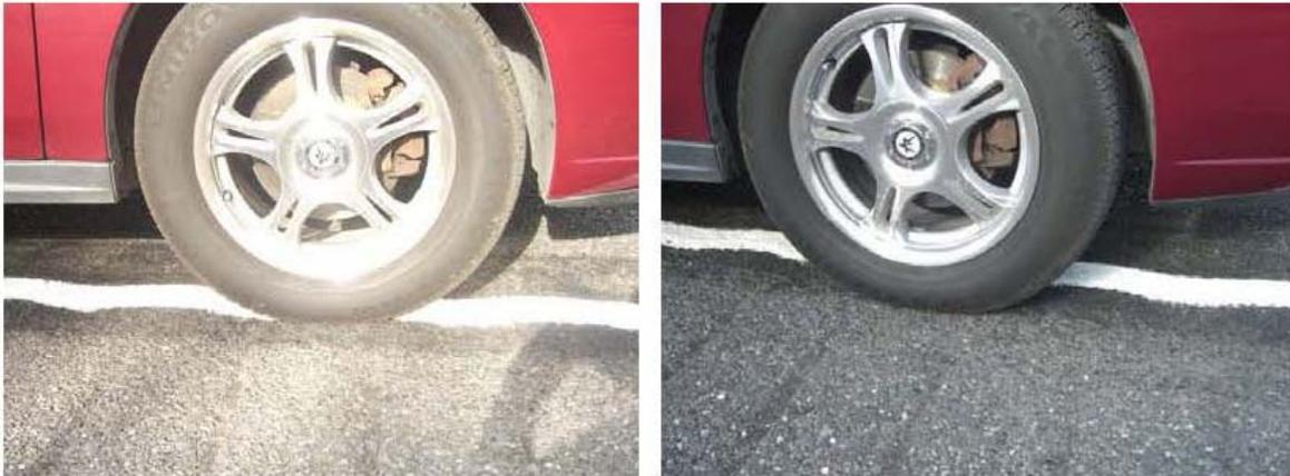
**Figure 9: Photographs of the test tire on crest of the mumble strip (left) and in the valley of the mumble strip (right)**
