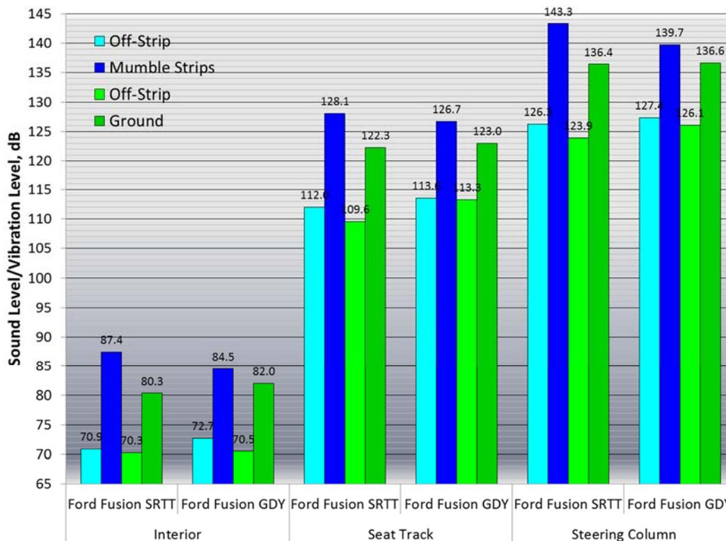
Figure 62: Overall A-weighted interior sound pressure and unweighted vibration levels for GDY tires and SRTT
