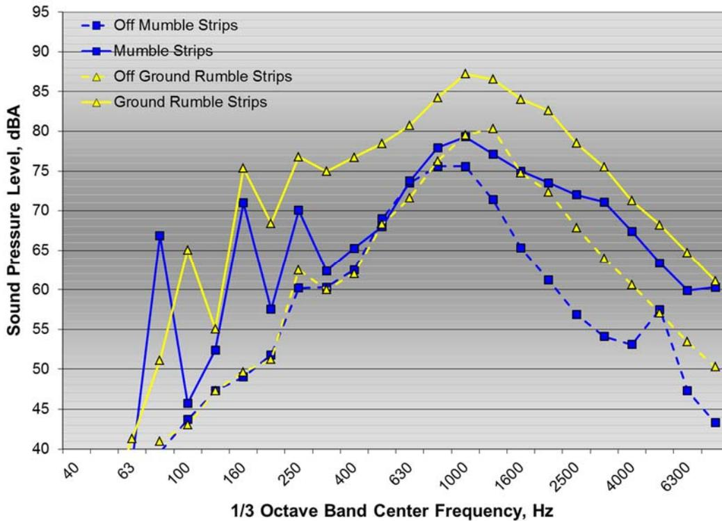
Figure 25: 1/3 octave band pass-by spectra for Ford Fusion test vehicle on (solid lines) and off (dashed lines) mumble strips and ground rumble strips
