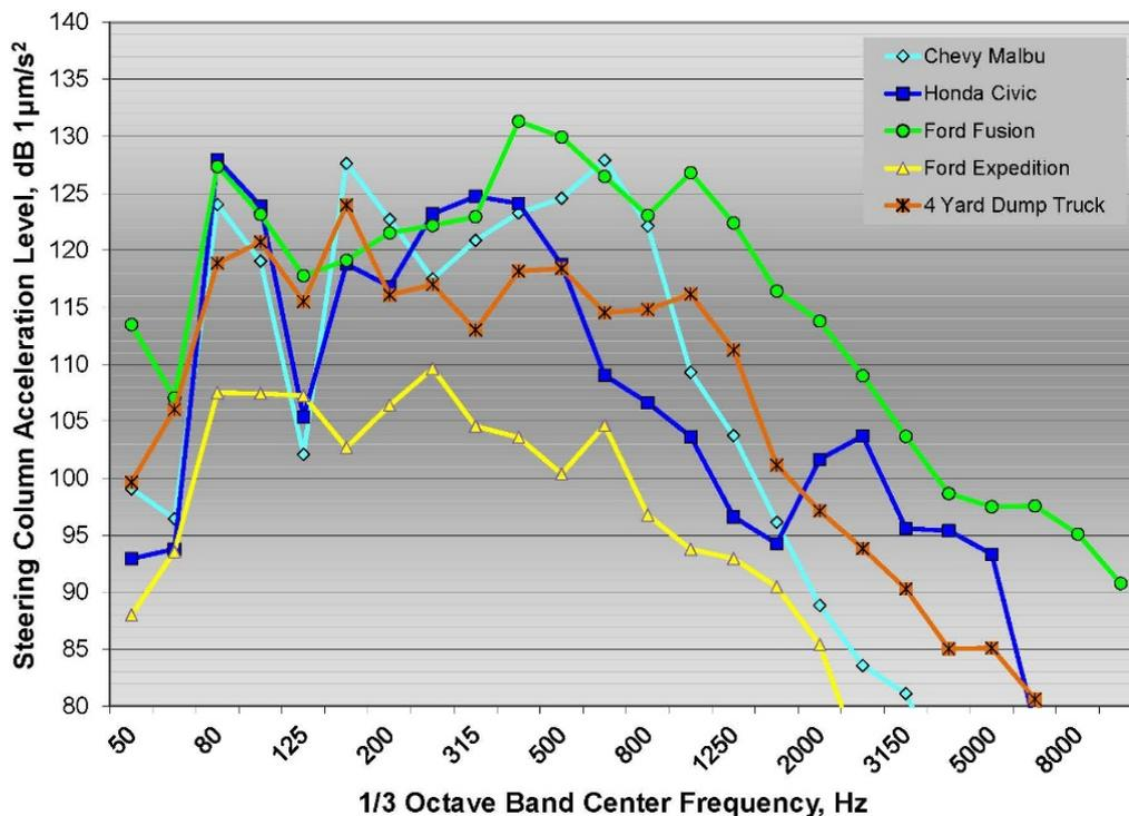
**Figure 47: 1/3 octave band steering column acceleration spectra for all five test vehicles on ground rumble strips**
