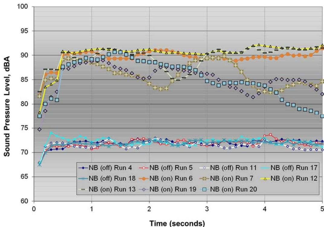
Figure 20: Interior noise measurement runs on and off the mumble strips by the Malibu test vehicle
