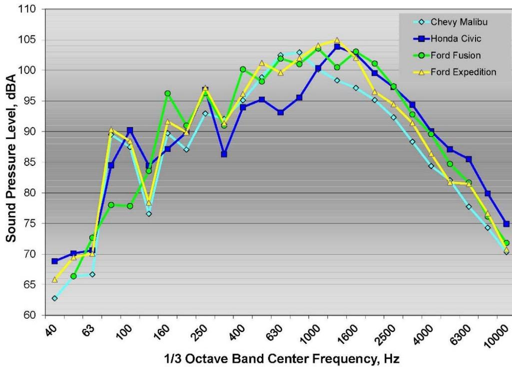
Figure 33: 1/3 octave band on-board exterior spectra on ground rumble strips for four test vehicles
