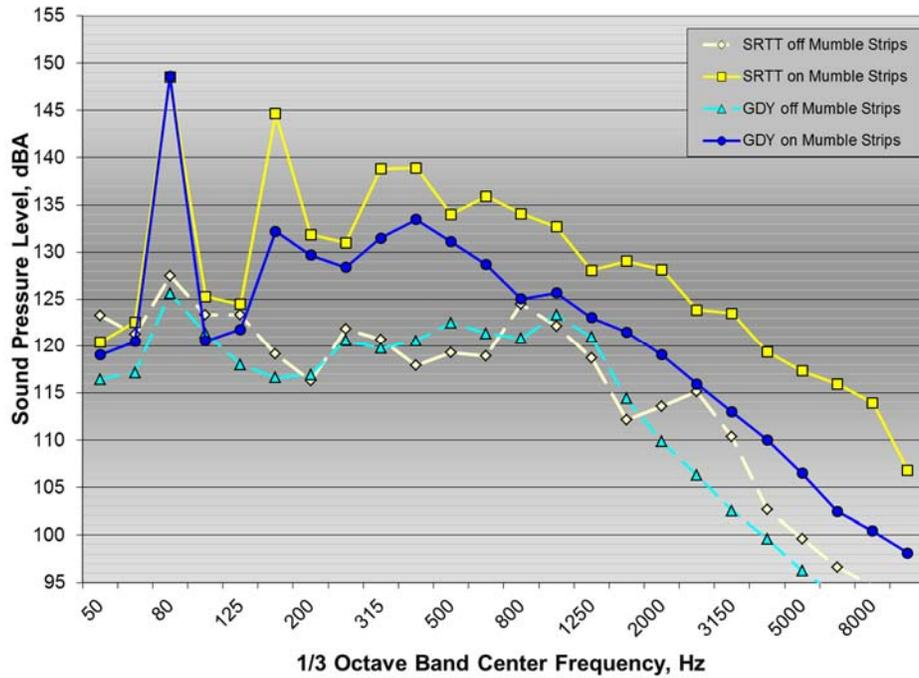
Figure A31: 1/3 octave band front fender acceleration spectra for Ford Fusion test vehicle on and off mumble strips with SRTT and Goodyear test tires
