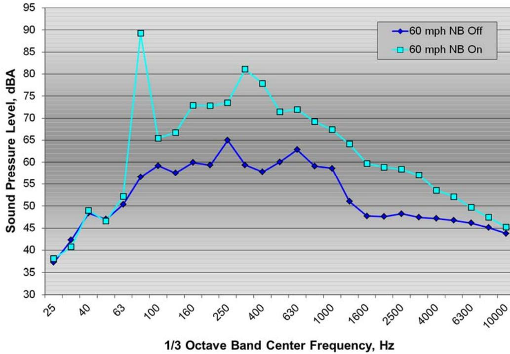
Figure 21: Interior noise 1/3 octave band spectra for the Malibu test vehicle traveling on and off the mumble strips
