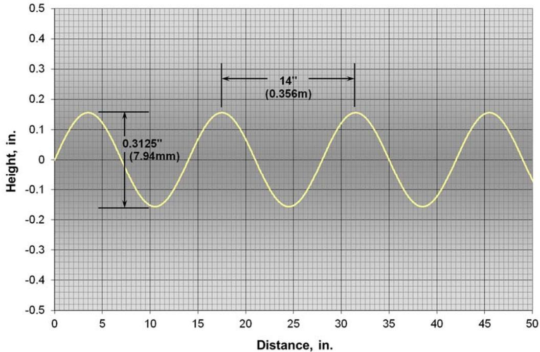
Figure 1: Recommended sinusoidal profile for mumble strips
