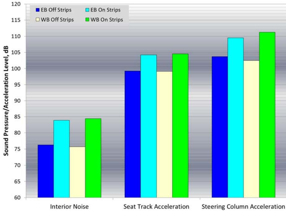
**Figure A6: Overall noise and acceleration levels for 4-yard dump truck test vehicle traveling at 60 mph both on and off ground rumble strips and both eastbound and westbound**
