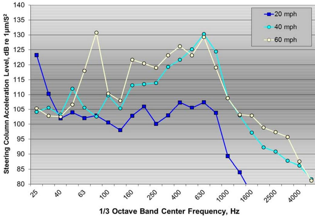
Figure 55: 1/3 octave band steering column acceleration level on mumble strips for the Malibu test vehicle at 20, 40, and 60 mph
