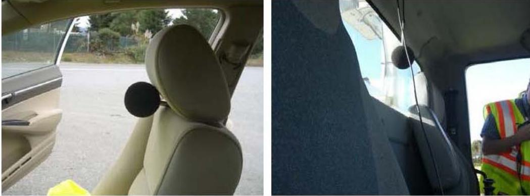
**Figure 15: Photographs of the interior noise microphone mounted in the Malibu test vehicle and in the 4-yard dump truck**
