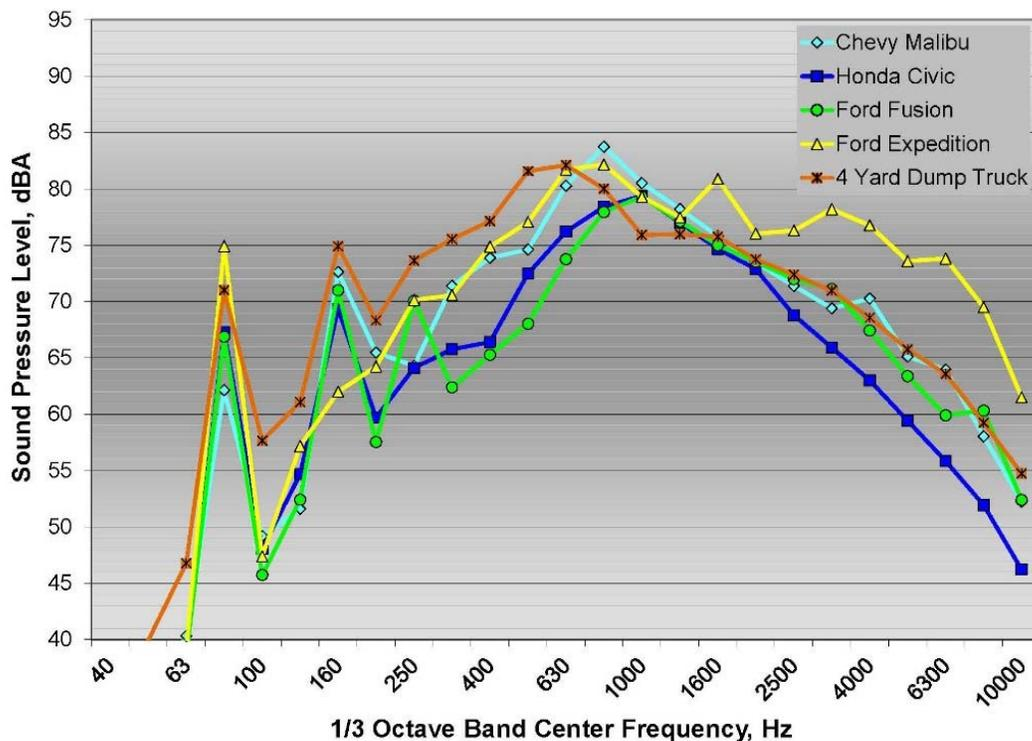
Figure 28: 1/3 octave band pass-by spectra on mumble strips for all five test vehicles
