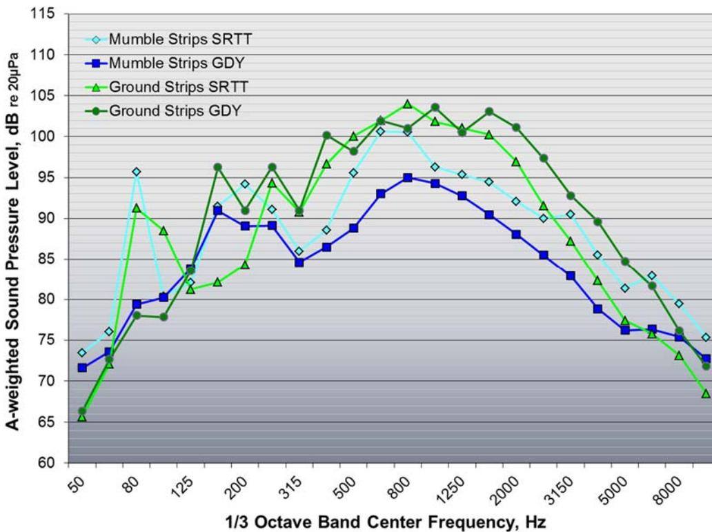
Figure 61: 1/3 octave band exterior sound pressure levels measured with GDY tires and SRTT
