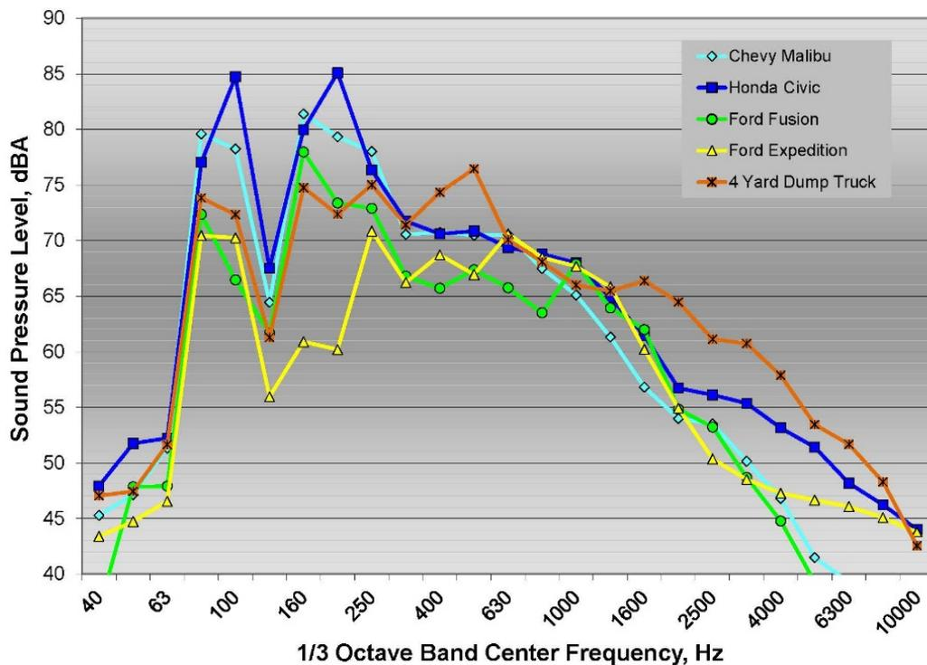
Figure 41: 1/3 octave band interior noise spectra for all five test vehicles on ground rumble strips
