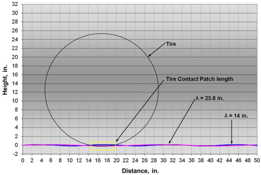
Figure 3: Relative geometries of rumble strip profiles, typical passenger car tire, and tire contact patch length
