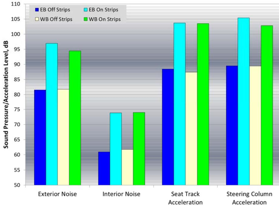
Figure A12: Overall noise and acceleration levels for Malibu test vehicle traveling at 20 mph both on and off ground rumble strips and both eastbound and westbound
