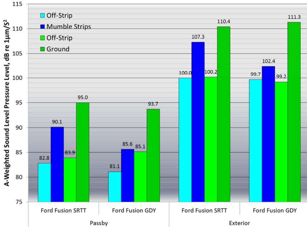
Figure 59: Overall A-weighted pass-by and exterior sound pressure levels for GDY tires and SRTT
