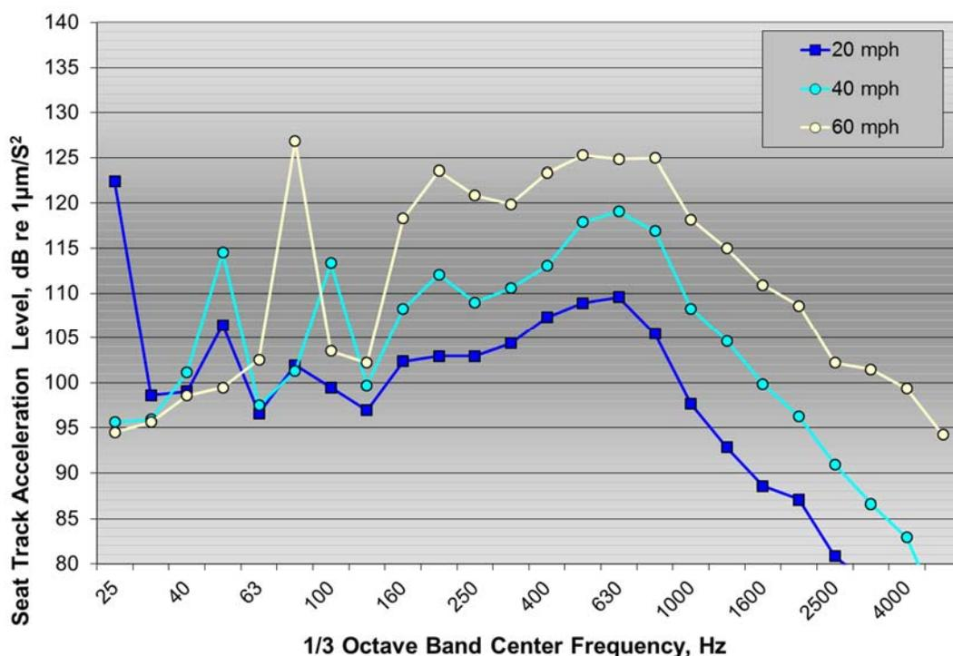
Figure 54: 1/3 octave band seat track acceleration level on mumble strips for the Malibu test vehicle at 20, 40, and 60 mph
