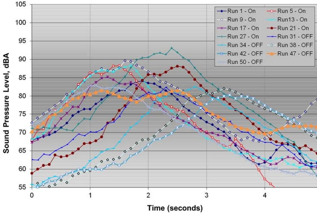
Figure 18: Pass-by time histories for travel on and off the mumble strips by the Malibu test vehicle
