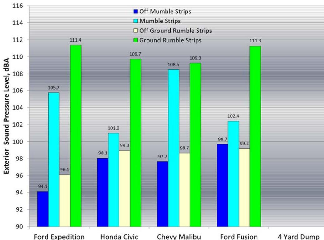
**Figure 31: Overall A-weighted on-board exterior sound pressure levels for four test vehicles on mumble and ground rumble strips**
