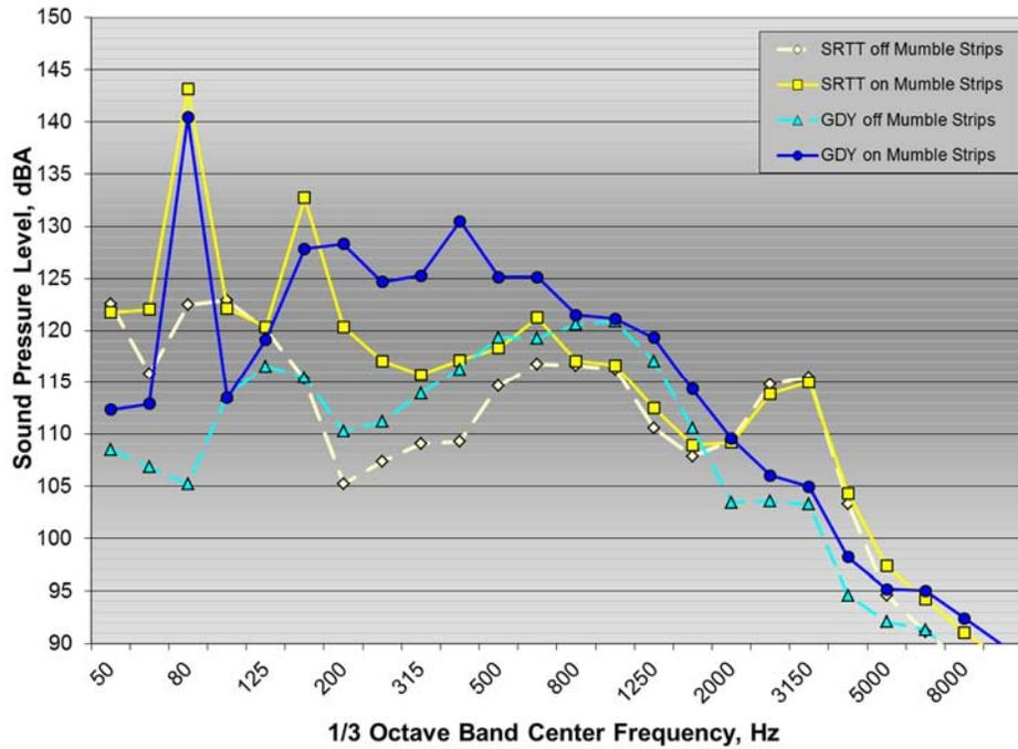
Figure A35: 1/3 octave band rear door acceleration spectra for Ford Fusion test vehicle on and off mumble strips with SRTT and Goodyear test tires
