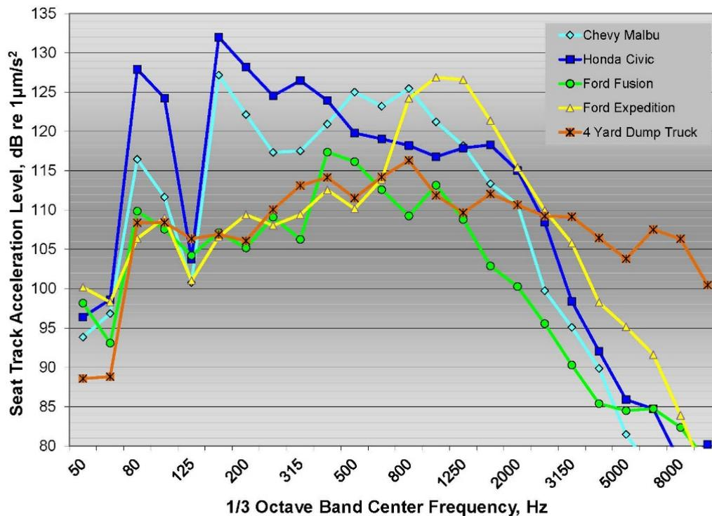
**Figure 44:** 1/3 octave band seat track acceleration spectra for all five test vehicles on ground rumble strips
