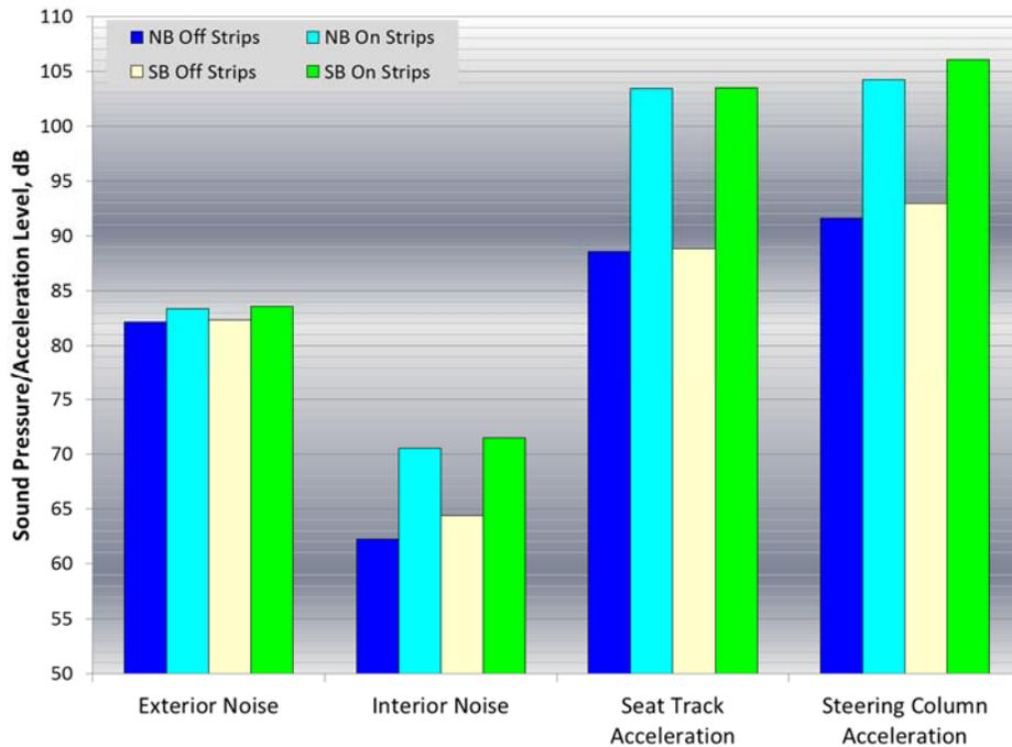
**Figure A11: Overall noise and acceleration levels for Malibu test vehicle traveling at 20 mph both on and off mumble strips and both northbound and southbound**
