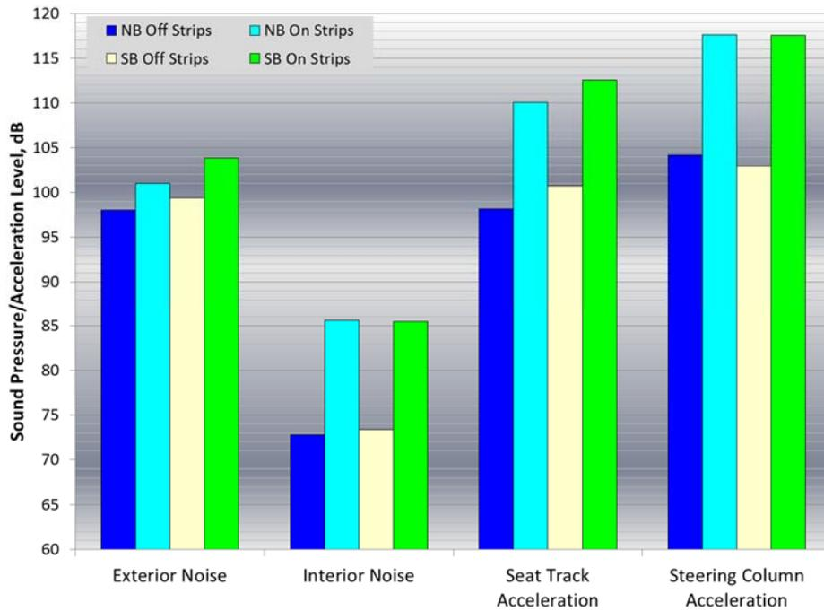
**Figure A3: Overall noise and acceleration levels for Civic test vehicle traveling at 60 mph both on and off mumble strips and both northbound and southbound**
