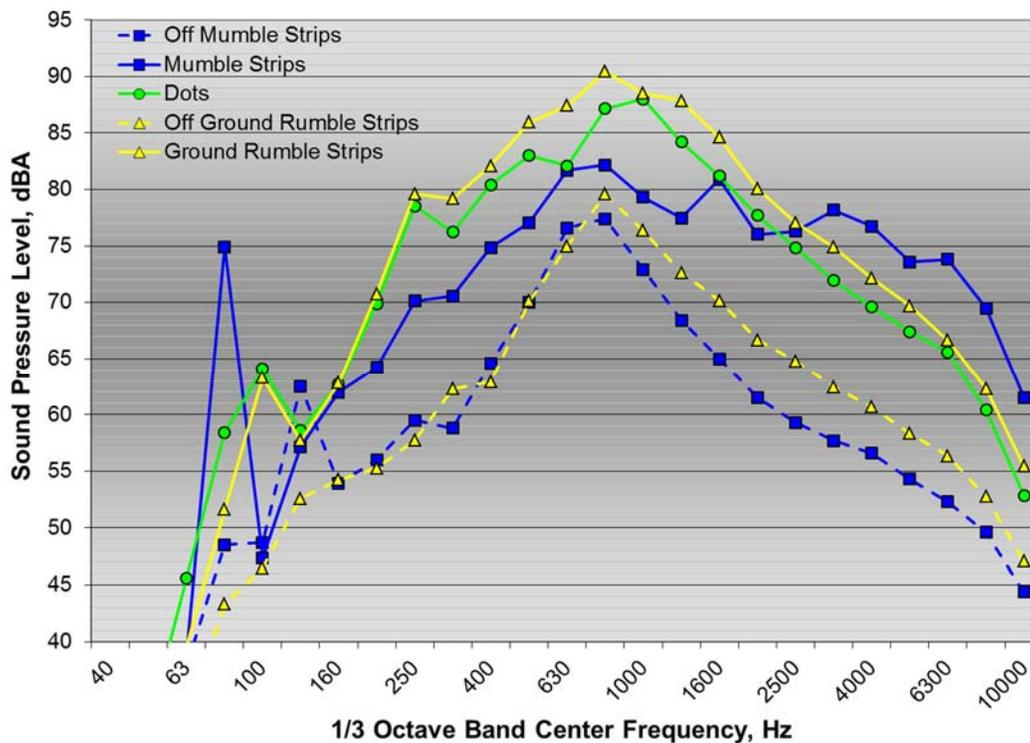
Figure 26: 1/3 octave band pass-by spectra for Expedition test vehicle on (solid lines) and off (dashed lines) mumble strips, dots, and ground rumble strips
