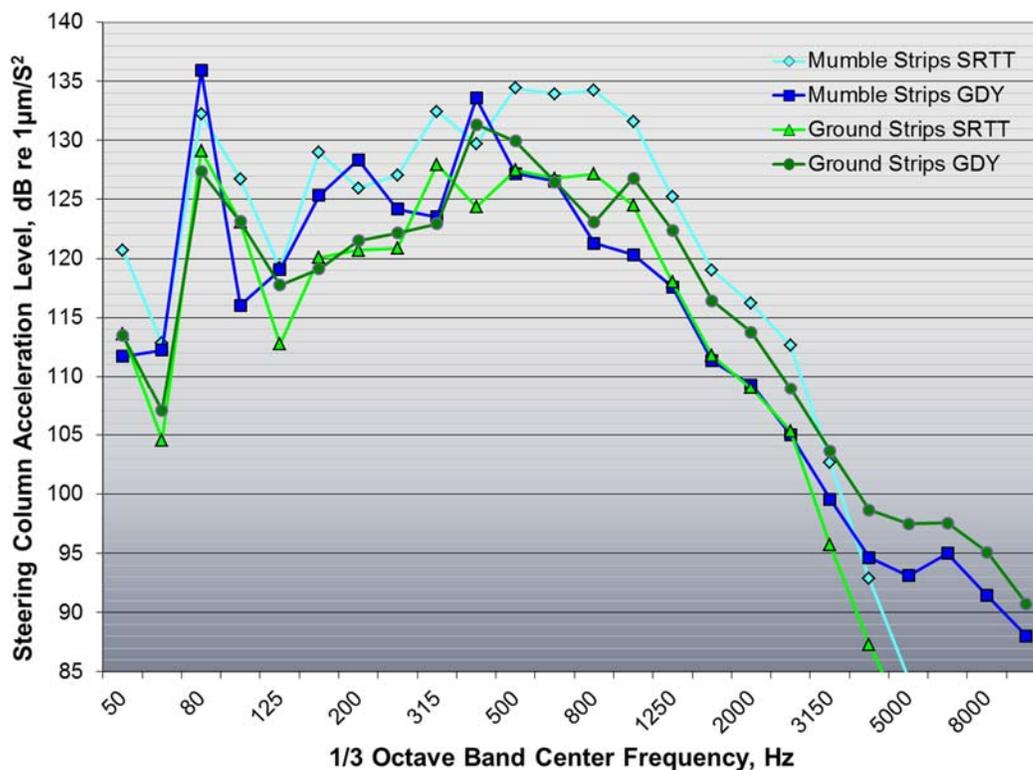
Figure 65: 1/3 octave band steering column acceleration levels measured with GDY tires and SRTT
