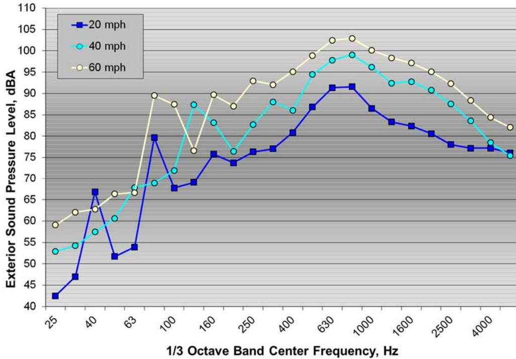
Figure 51: 1/3 octave band on-board exterior noise spectra on ground rumble strips for the Malibu test vehicle at 20, 40, and 60 mph
