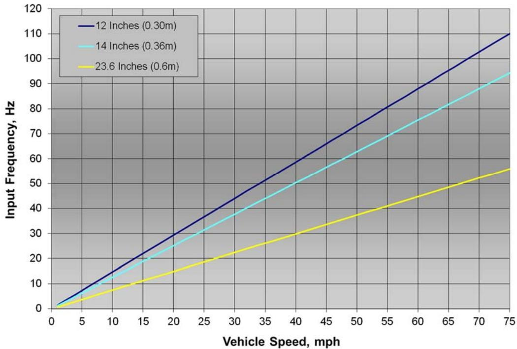
Figure 6: Forcing function frequency as a function of vehicle speed for different λ values
