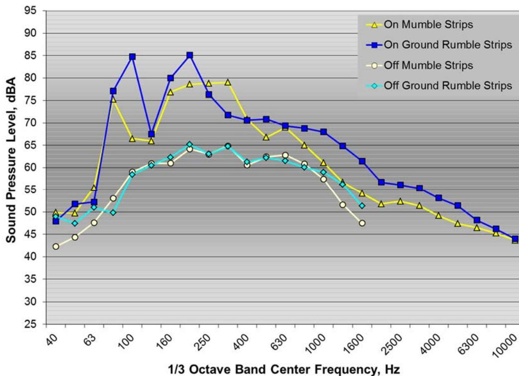
Figure 36: 1/3 octave band interior noise spectra for Civic test vehicle on and off mumble strips and ground rumble strips
