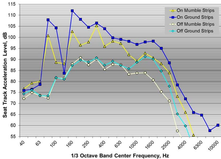
Figure A15:  $\frac{1}{3}$  octave band seat track acceleration spectra for Civic test vehicle on and off mumble strips and ground rumble strips at 60 mph
