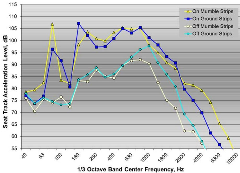
Figure A13: 1/3 octave band seat track acceleration spectra for Malibu test vehicle on and off mumble strips and ground rumble strips at 60 mph
