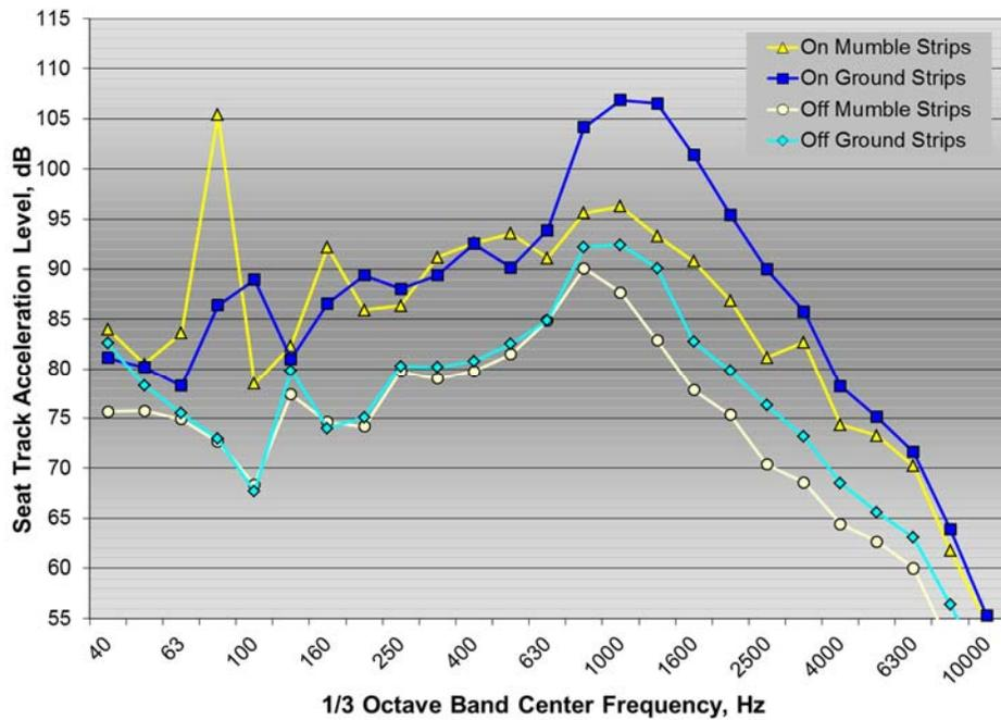
Figure A17: 1/3 octave band seat track acceleration spectra for Expedition test vehicle on and off mumble strips and ground rumble strips at 60 mph
