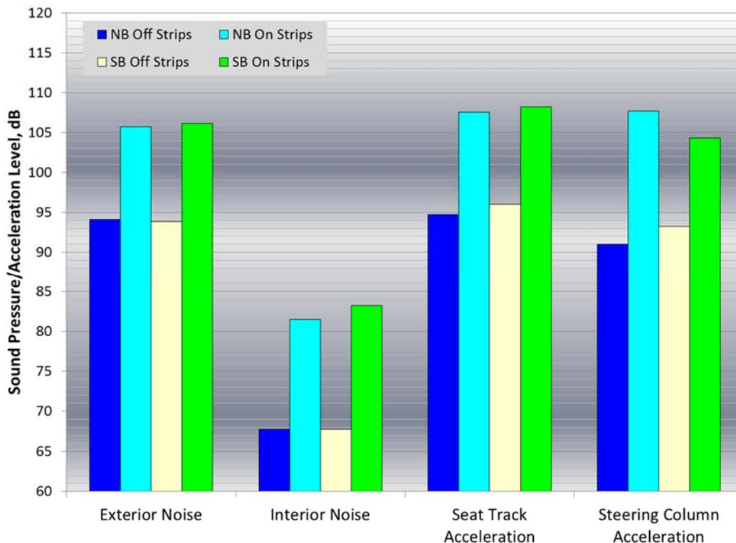
**Figure A1: Overall noise and acceleration levels for Expedition test vehicle traveling at 60 mph both on and off mumble strips and both northbound and southbound**
