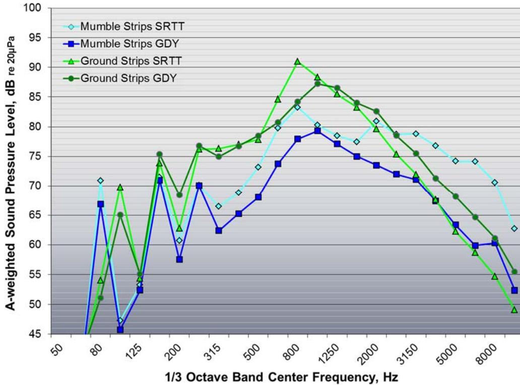
Figure 60: 1/3 octave band pass-by sound pressure levels measured with GDY tires and SRTT
