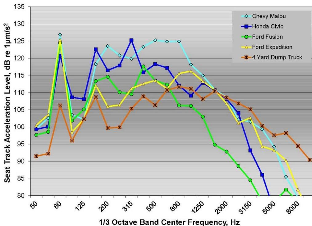
**Figure 43:** 1/3 octave band seat track acceleration spectra for all five test vehicles on mumble strips
