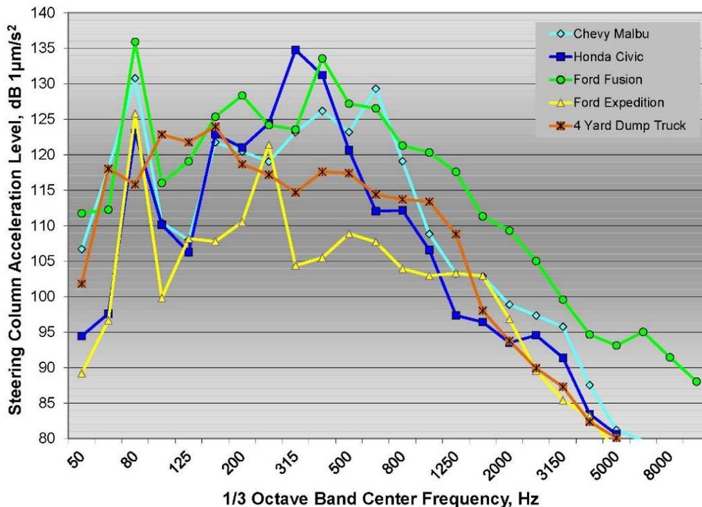
**Figure 46: 1/3 octave band steering column acceleration spectra for all four test vehicles on mumble strips**
