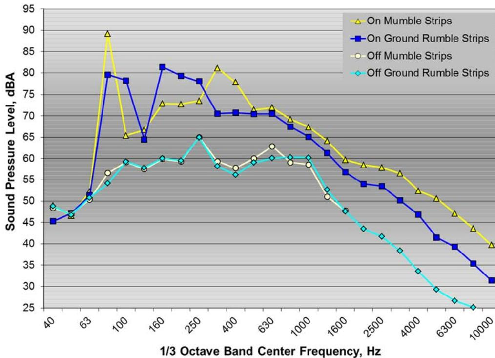
Figure 35:  $\frac{1}{3}$  octave band interior noise spectra for Malibu test vehicle on and off mumble strips and ground rumble strips
