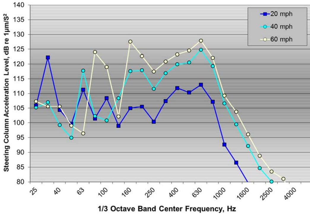
Figure 57: 1/3 octave band steering column acceleration level on ground rumble strips for the Malibu test vehicle at 20, 40, and 60 mph
