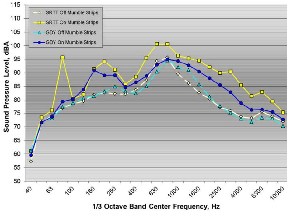
Figure A23: 1/3 octave band exterior noise spectra for Ford Fusion test vehicle on and off mumble strips with SRTT and Goodyear test tires
