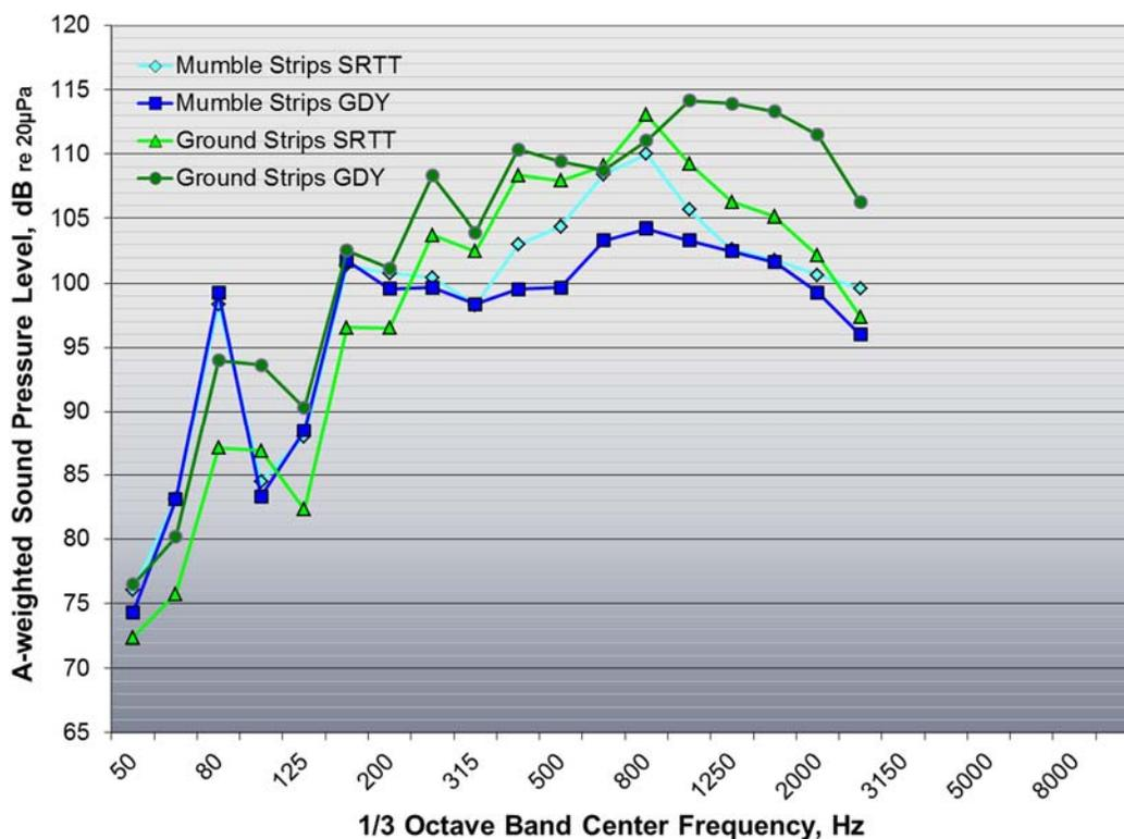
Figure 68:  $\frac{1}{3}$  octave band sound pressure levels measured by the OBSI probes for the GDY tires and SRTT
