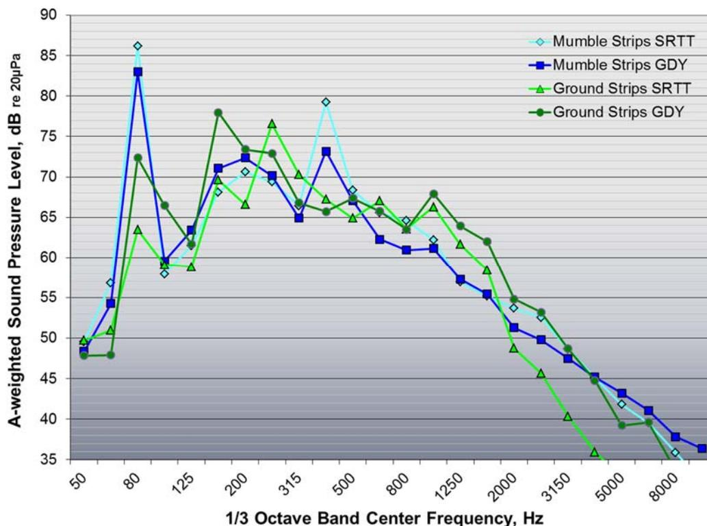
**Figure 63:** 1/3 octave band interior sound pressure levels measured with GDY tires and SRTT
