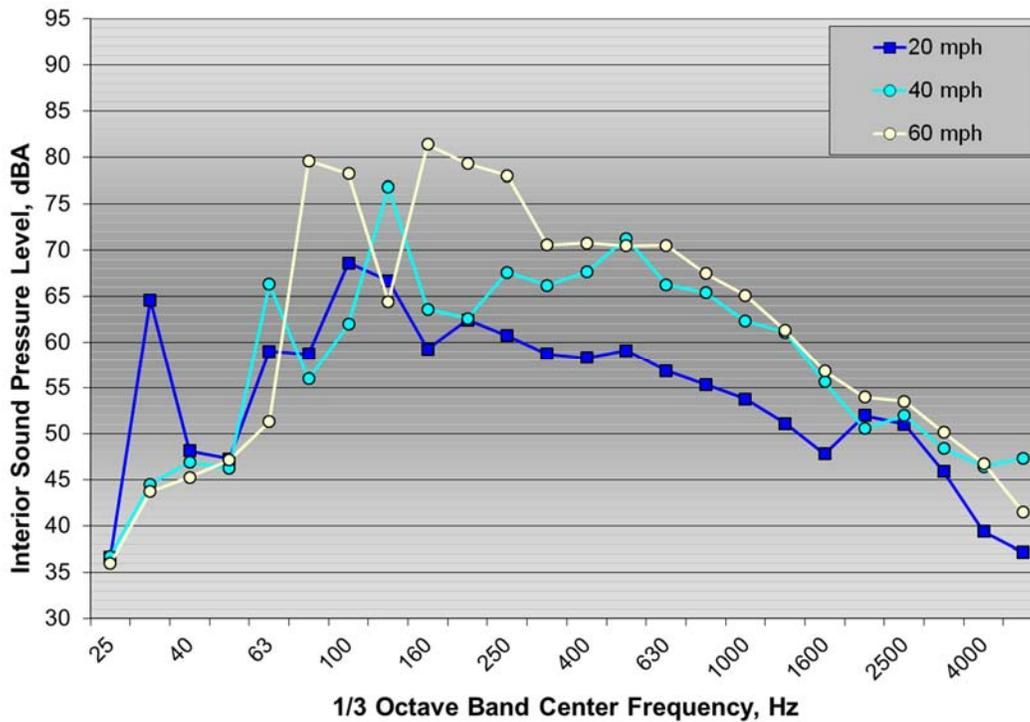
Figure 52: 1/3 octave band interior noise spectra on ground rumble strips for the Malibu test vehicle at 20, 40, and 60 mph
