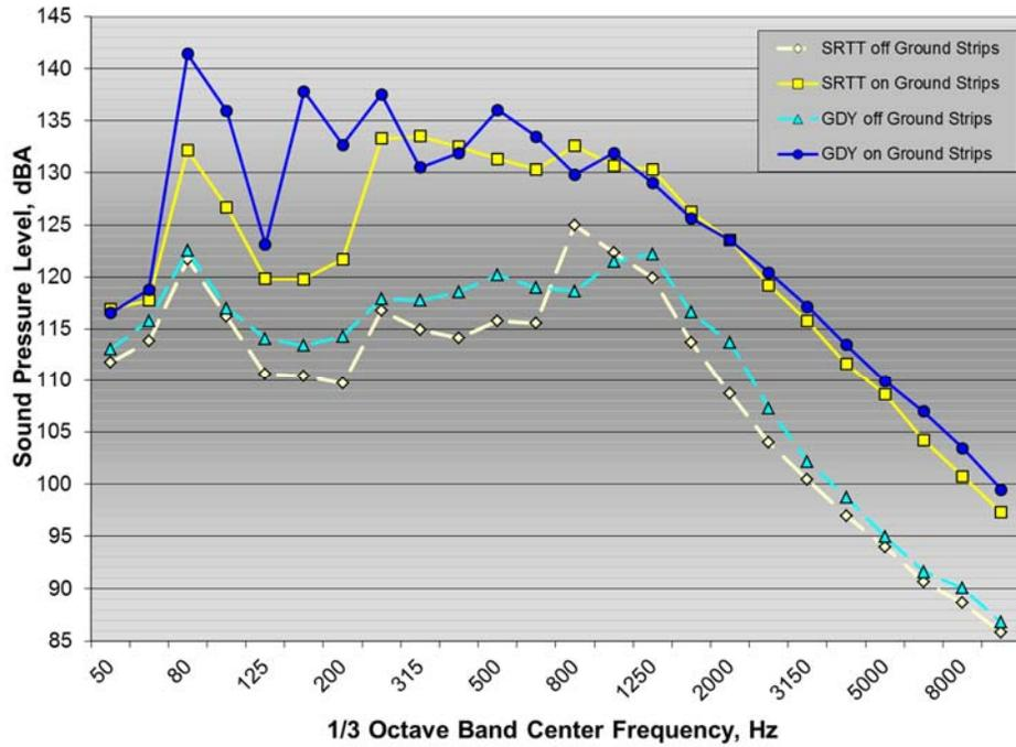
**Figure A32:** 1/3 octave band front fender acceleration spectra for Ford Fusion test vehicle on and off ground rumble strips with SRTT and Goodyear test tires
