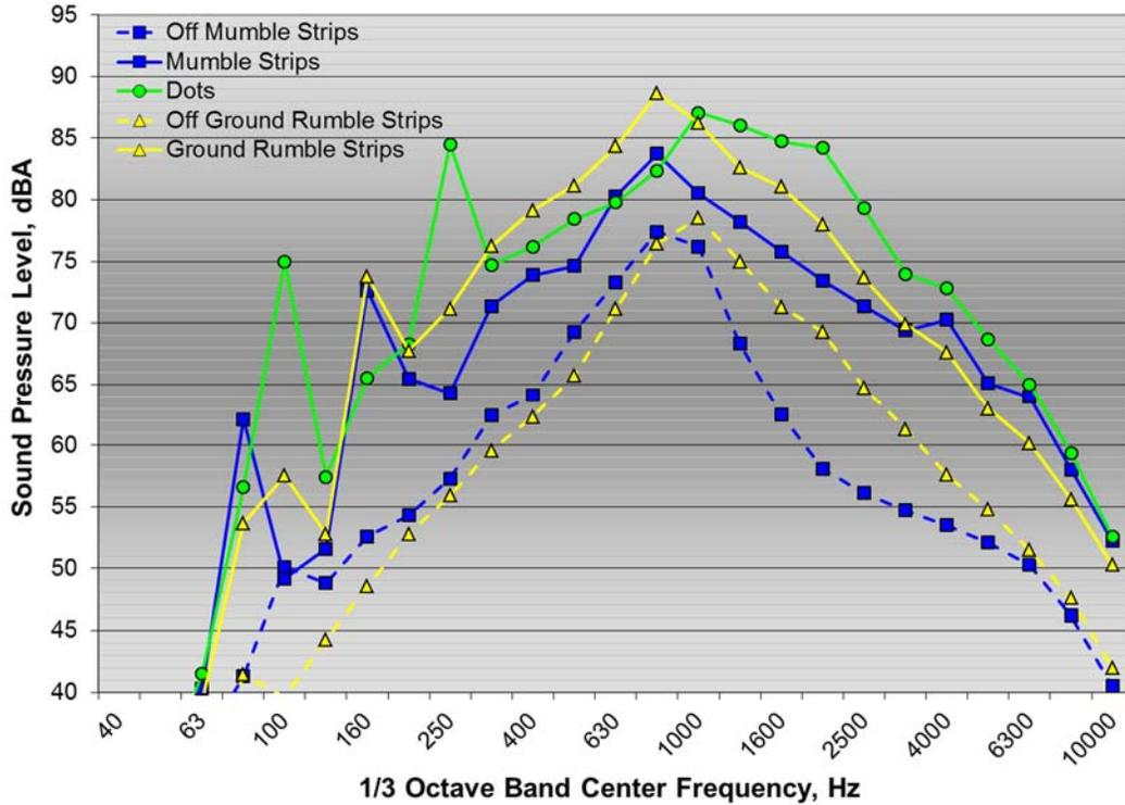
Figure 23: 1/3 octave band pass-by spectra for Malibu test vehicle on (solid lines) and off (dashed lines) mumble strips, dots, and ground rumble strips
