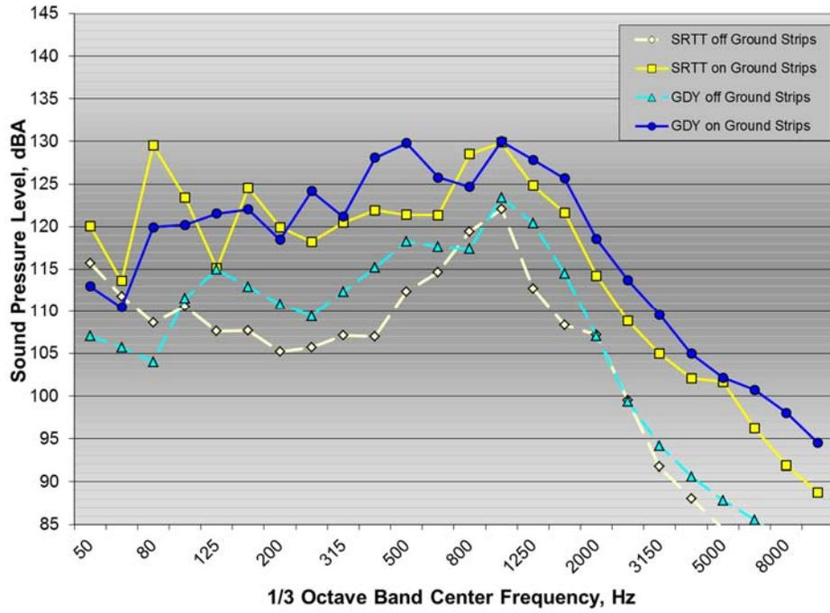
**Figure A36: 1/3 octave band rear door acceleration spectra for Ford Fusion test vehicle on and off ground rumble strips with SRTT and Goodyear test tires**
