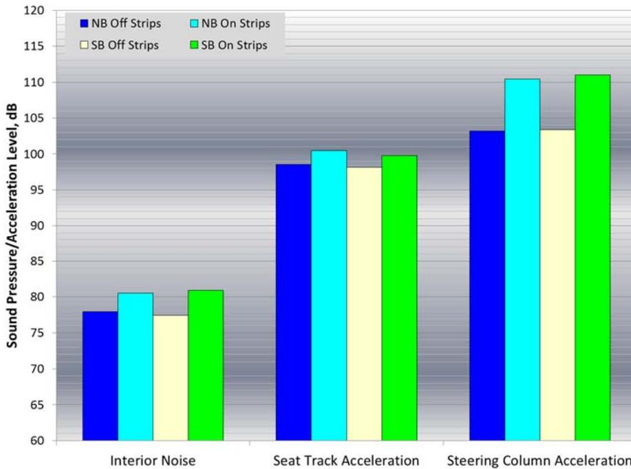
**Figure A5: Overall noise and acceleration levels for 4-yard dump truck test vehicle traveling at 60 mph both on and off mumble strips and both northbound and southbound**
