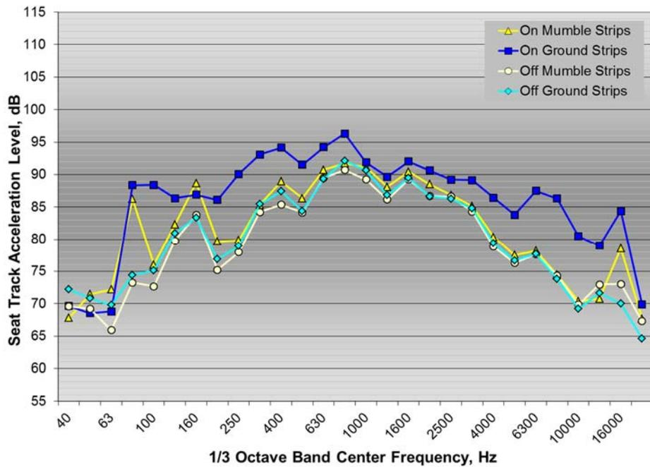
Figure A19:  $\frac{1}{3}$  octave band seat track acceleration spectra for 4-yard dump truck test vehicle on and off mumble strips and ground rumble strips at 60 mph
