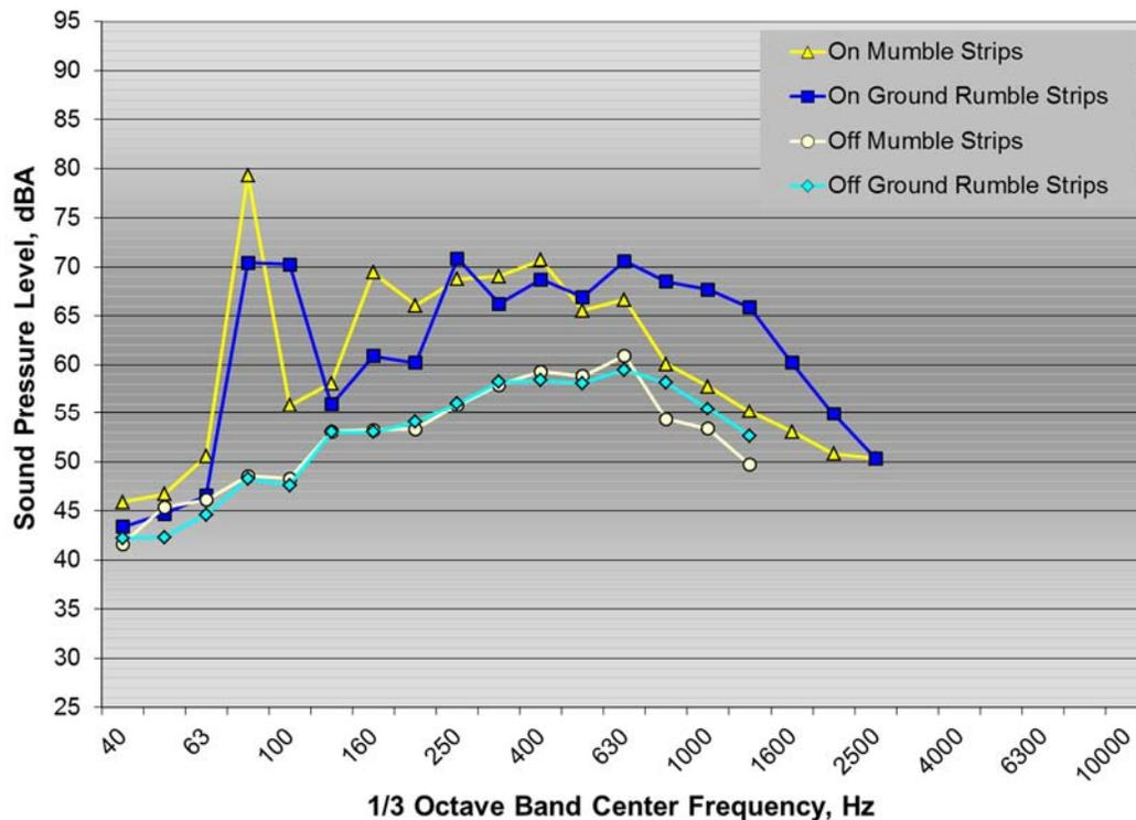
**Figure 38: 1/3 octave band interior noise spectra for Expedition test vehicle on and off mumble strips and ground rumble strips**
