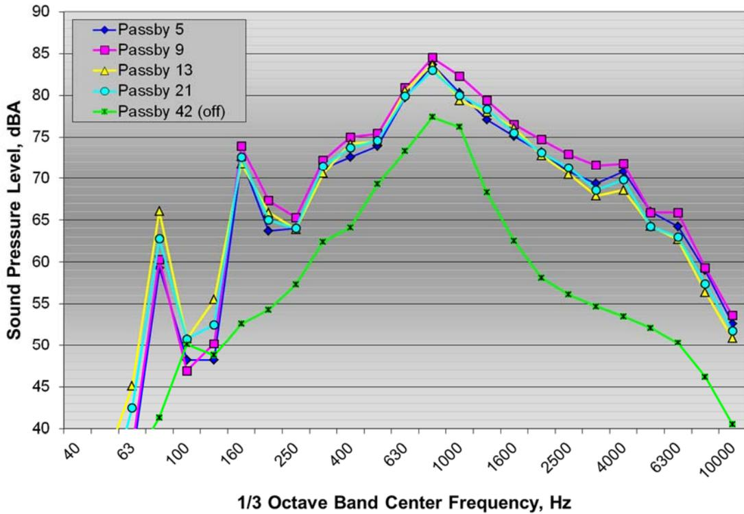
Figure 19: Spectra at maximum overall A-weighted sound level for multiple pass-bys on the mumble strips and one pass-by off the strips by the Malibu test vehicle
