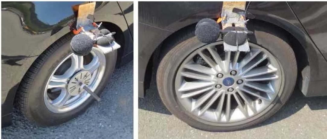
**Figure 58: SRTT (left) and GDY test tire (right)**
