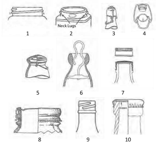
1. External thread; 2. Lug seal; 3, 4, 5. Light-ening stopper; 6. Hutchinson Stopper; 7. External thread w/ screw cap; 8. Seal and band; 9. Continuous thread; 10. Crown Cap
