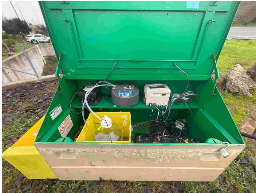
Figure 4-2. Example of typical Caltrans automated sampling equipment
