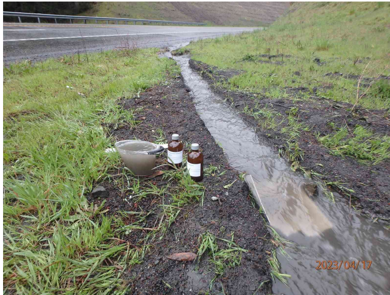
Figure 4-14. Edge-of-pavement stormwater influent to bioswale at Station 1-344 (Circle Point Curve) Channel installed to facilitate sampling. Inflow is sampled from the Teflon sheeting to the right of the bottles.
