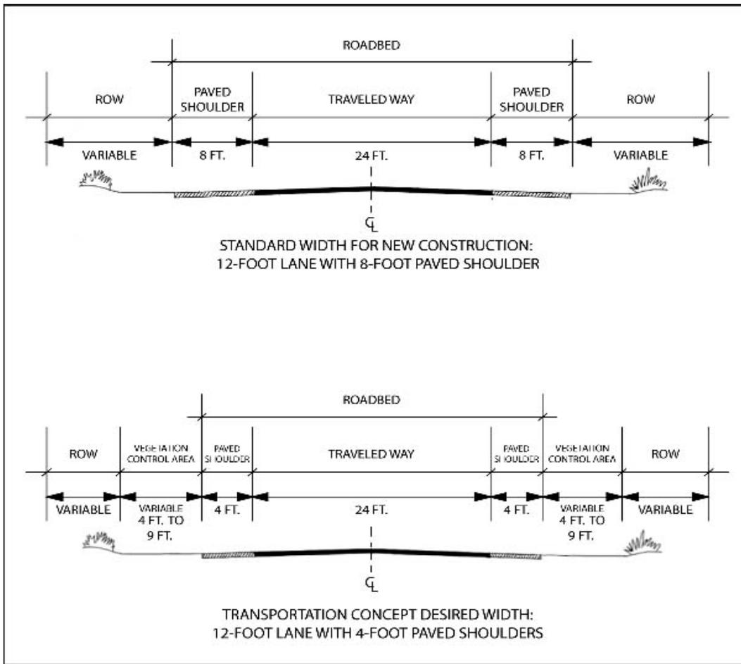
*Figure 5: Comparison of typical cross sections on a standard width for new construction on a rural two-lane highway and the Transportation Concept desired width for Highway 1. The main difference is the width of the paved shoulder (8 feet vs. 4 feet); the desired width also accommodates roadside features for the unpaved shoulder within the vegetation control area.*
