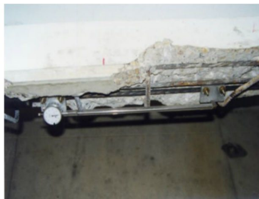
Figure 7-9. ABITB Stressing Gauge (NCHRP20-07(307), 2012)
