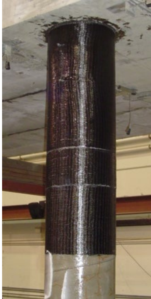
Figure 7-20. Partial CFRP Wrap of a Column
