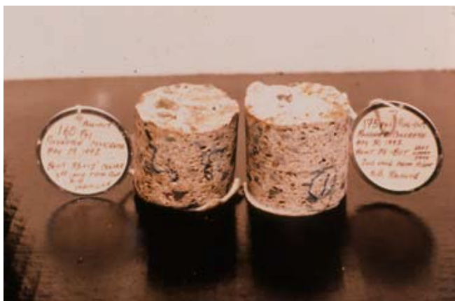
Figure 5-67. Pull-out Test Cores
