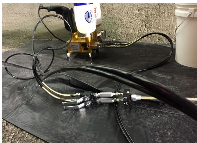
Figure 5-29. Epoxy Injection Pump and Injection Gun
