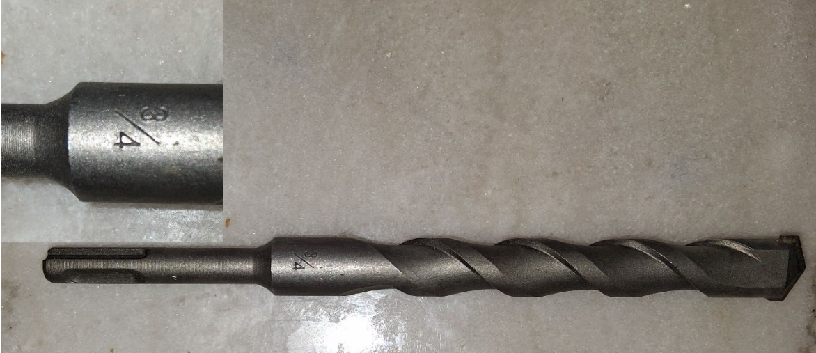
Figure 4-29. Drill Diameter Size Marking on The Shank of Drill Bit
