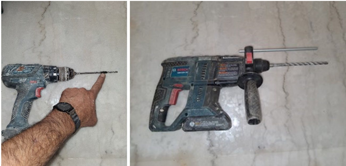
Figure 4-28. Use of Tape Around Drill Bit or Drill Stop to Achieve the Desired Hole Depth
