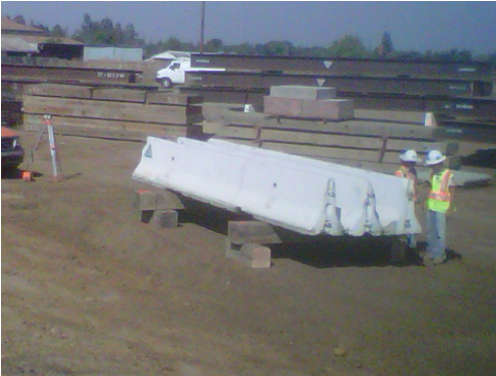
Figure 8-16. Simple Static Soil Load Test Using K-Rail.
