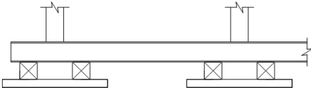
Figure 7-16. Concrete Pads with Cap Beam.
