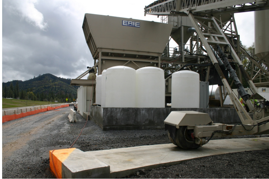
Figure 4-3a. Aggregate Storage Bins.
