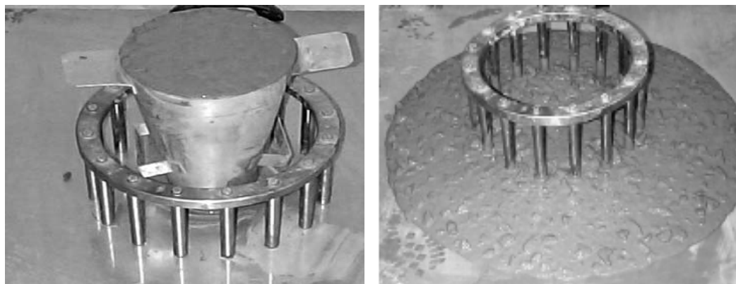
Figure 9-9. J-Ring Test (Ref. ASTM C1621).
