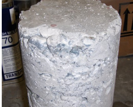
(a) Cylinder Cast with Rock Pockets.
