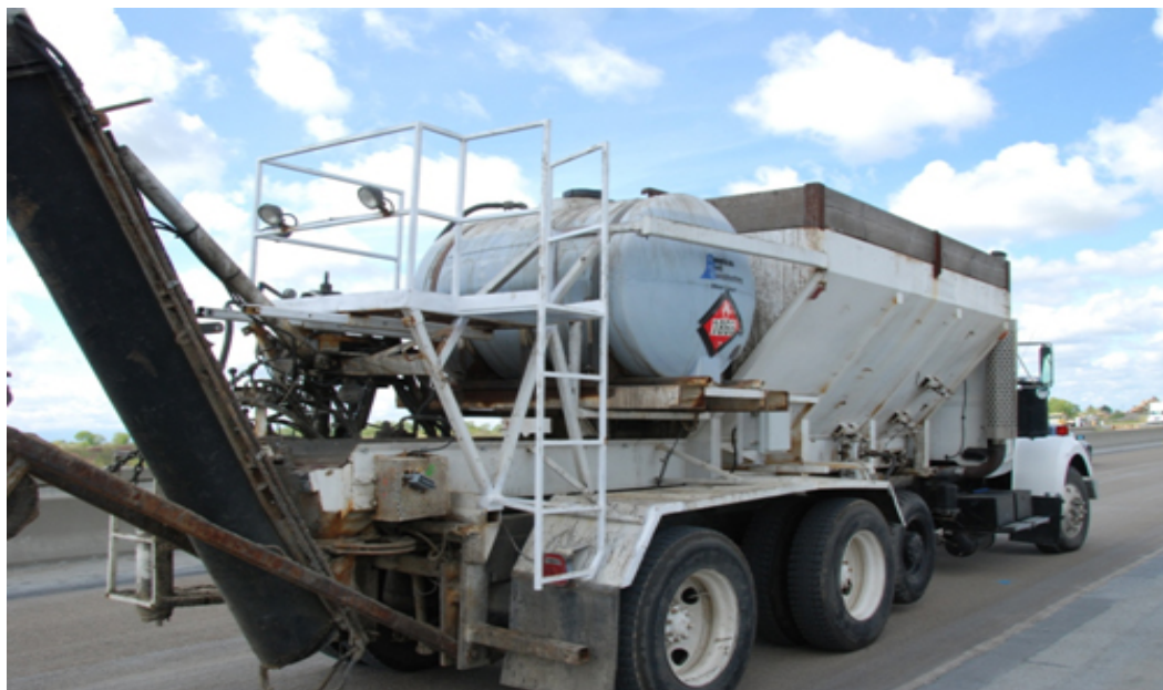
Figure 6-16. Volumetric Operation (Note HAZMAT Placard ID # 1866).
