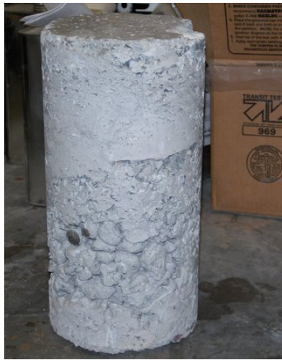
(c) Cylinder Poorly Cast.
