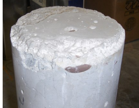
(b) Cylinder Not Filled Properly.
