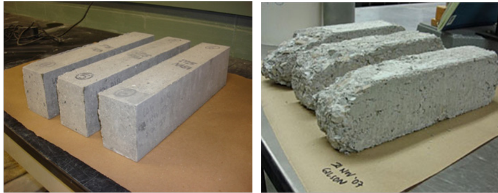
Figure 1-6. Freeze-Thaw Damage, Before and After Photos 3 .
