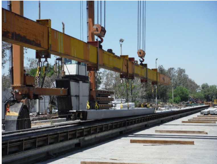
Figure 8-1. PC PS Concrete Pile Fabrication
