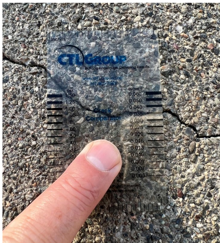
Figure 7-37. Crack Width Measurement with a Crack Comparator
