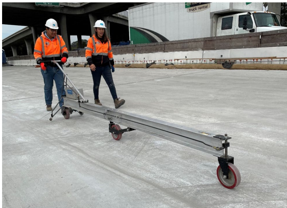
Figure 7-35. Smoothness Testing per California Test 547
