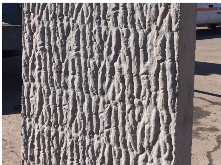
Figure 5-36. Test Panel for Fractured Granite Texture
