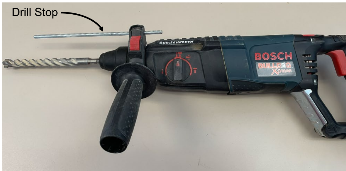
Figure 4-25. Drill with Drill Stop Attachment
