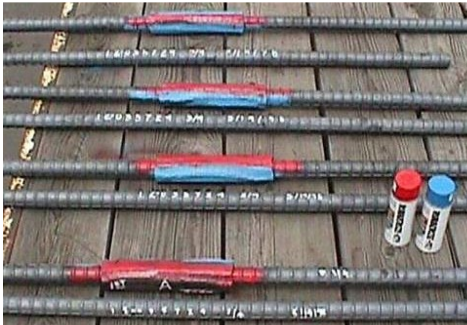
Figure 4-18. Tamper Proof Marking on Production Sample Splices
