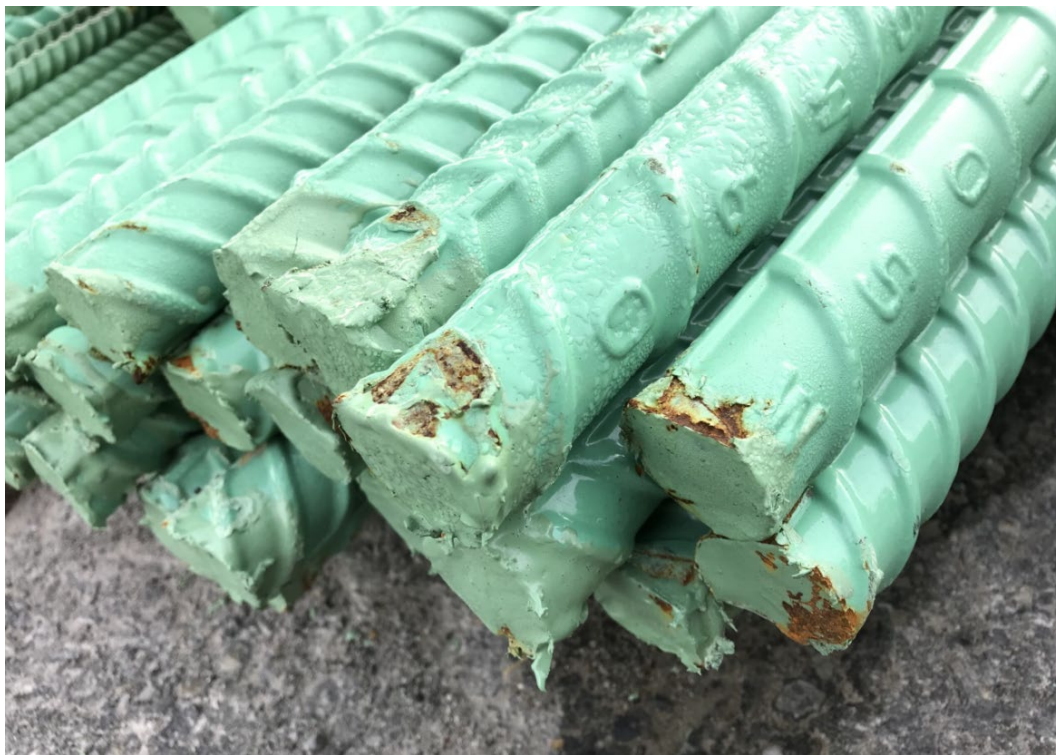
Figure 4-11. Damaged Epoxy Coating
