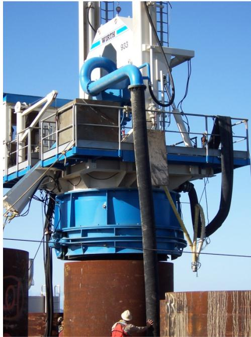
**Figure 6-12. Reverse Circulation Drilling Equipment.**
