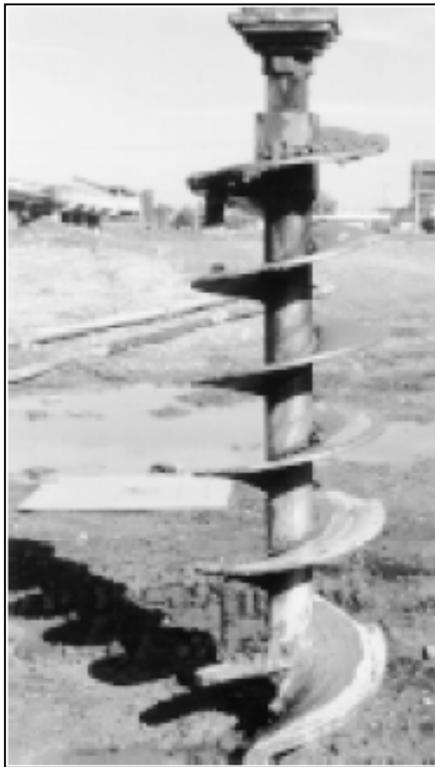
Figure 6-1. Short Flight Auger.
