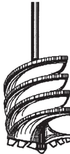
Figure 6-4. Double Flight Auger.
