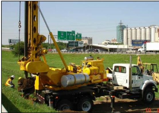
Figure 6-15. Truck Mounted Drill Rig.
