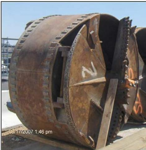
Figure 6-6. Drilling Bucket.
