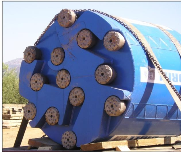
Figure 6-9. Down-Hole Hammer.
