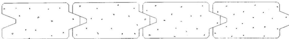
Figure 12-4. Concrete Sheet Piling.
