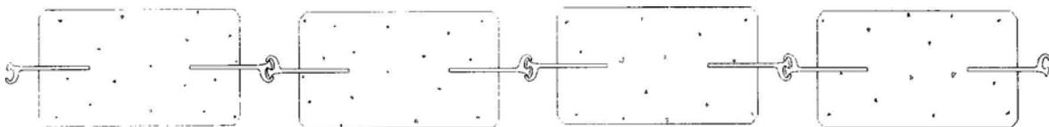
Figure 12-5. Concrete Sheet Piling with Steel Interlocks.
