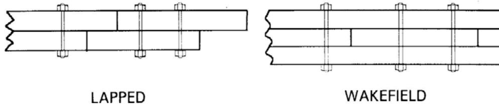
Figure 12-2. Lapped and Wakefield Sheet Piling.
