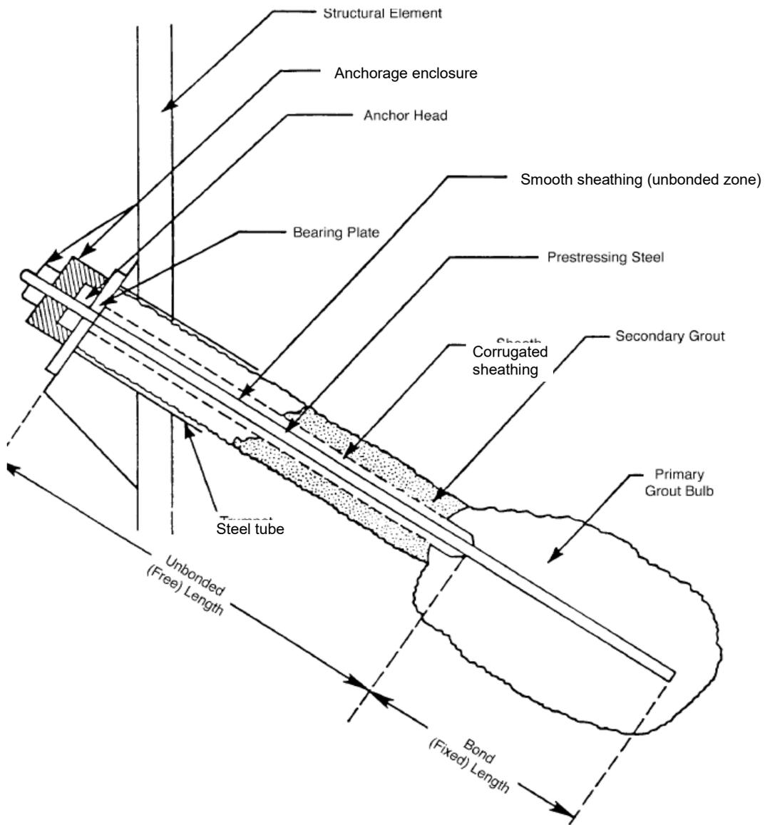
Figure 11-1. Sub Horizontal Ground Anchor Schematic.
