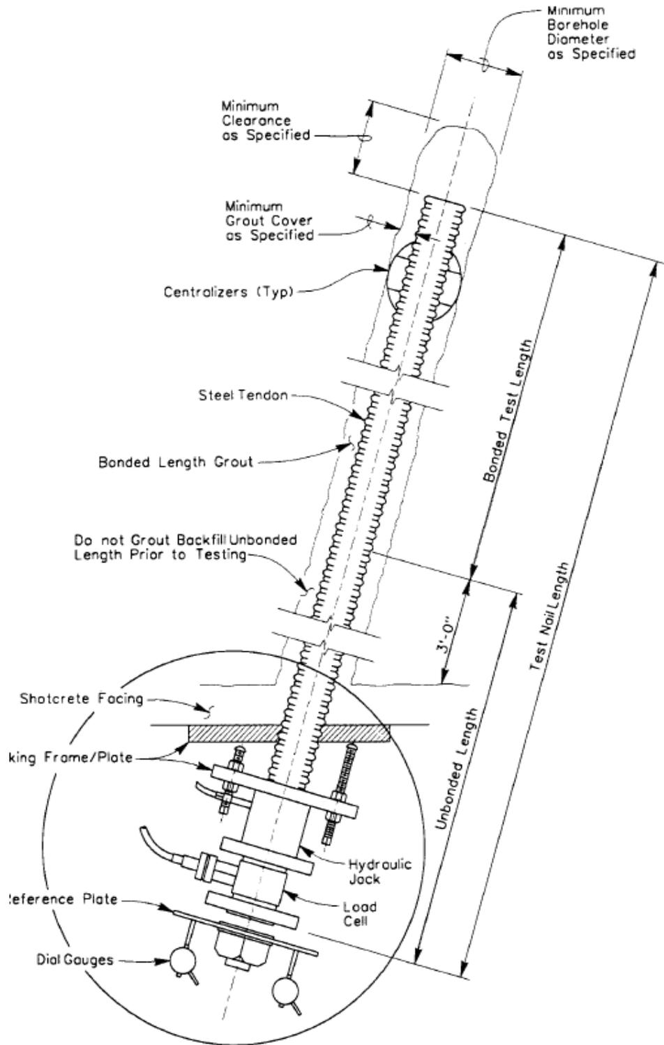
Figure 11-5. Verification/Test Nail Detail.
