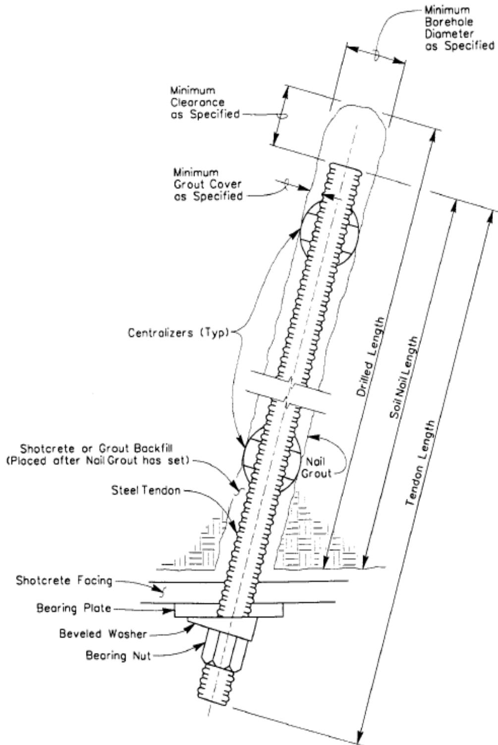
Figure 11-4. Soil Nail Detail.
