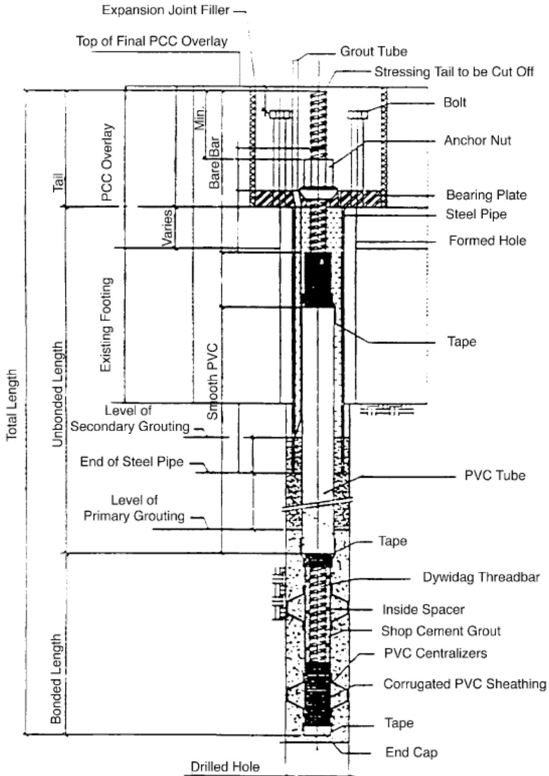
Figure 11-2. Vertical Ground Anchor Schematic.
