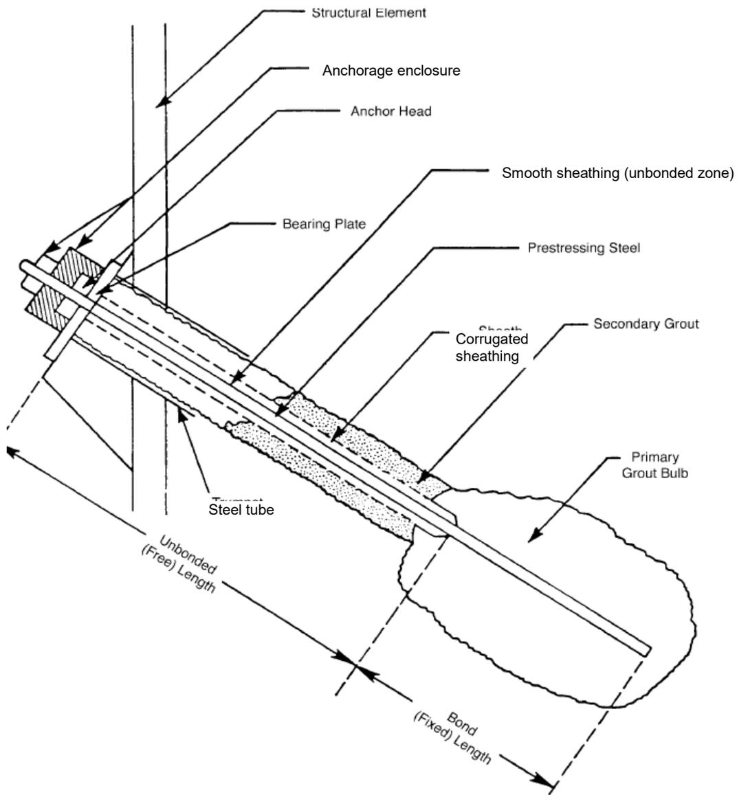
Figure 11-1. Sub Horizontal Ground Anchor Schematic.
