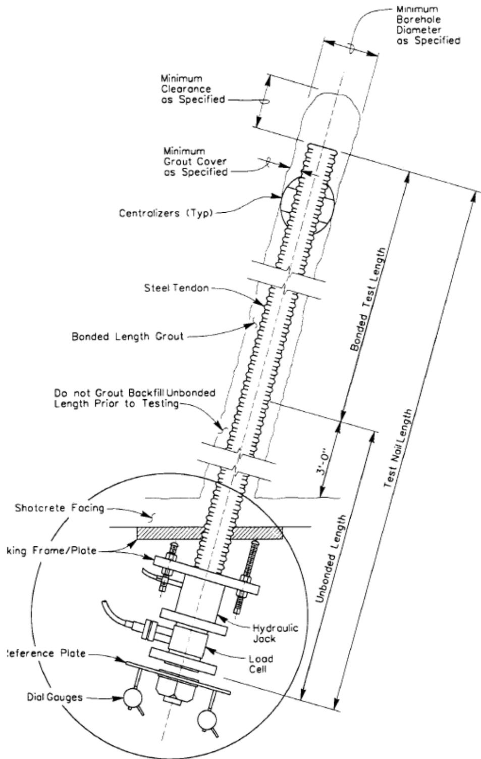
Figure 11-5. Verification/Test Nail Detail.
