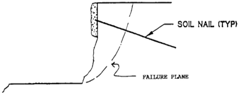
Figure 11-3. Soil Nail Schematic.
