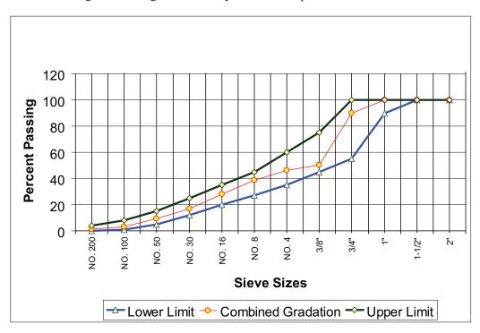
The resulting combined gradation analysis would be plotted out as shown:
