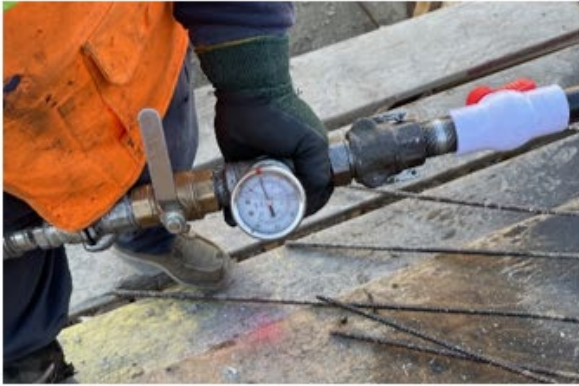
Air pressure test. Contractor marked dial with red at the target starting pressure.
