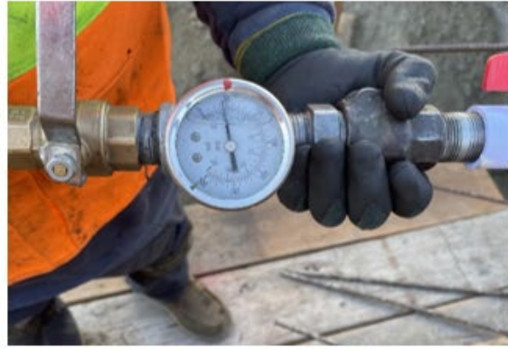
Air pressure test. Contractor marked dial with red at the target starting pressure.
