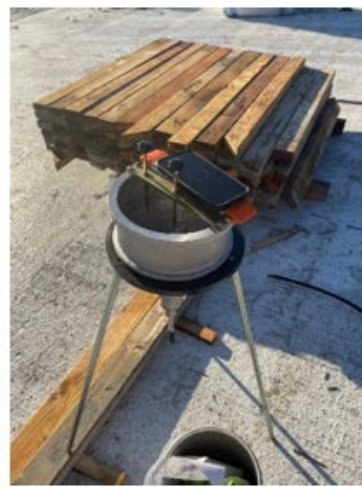
Grouting operation and apparatus for CT 541.
