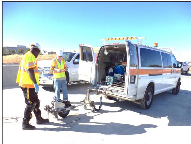
Figure 6.1-2. Coefficient of Friction Testing per *California Test 342*.
