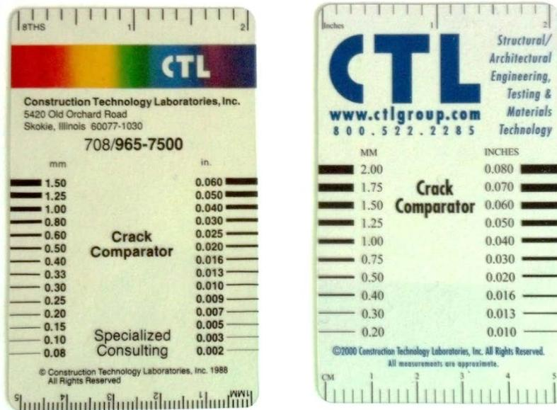
Figure 6.1-3. Crack Comparator Makes Checking Crack Width Easier.
