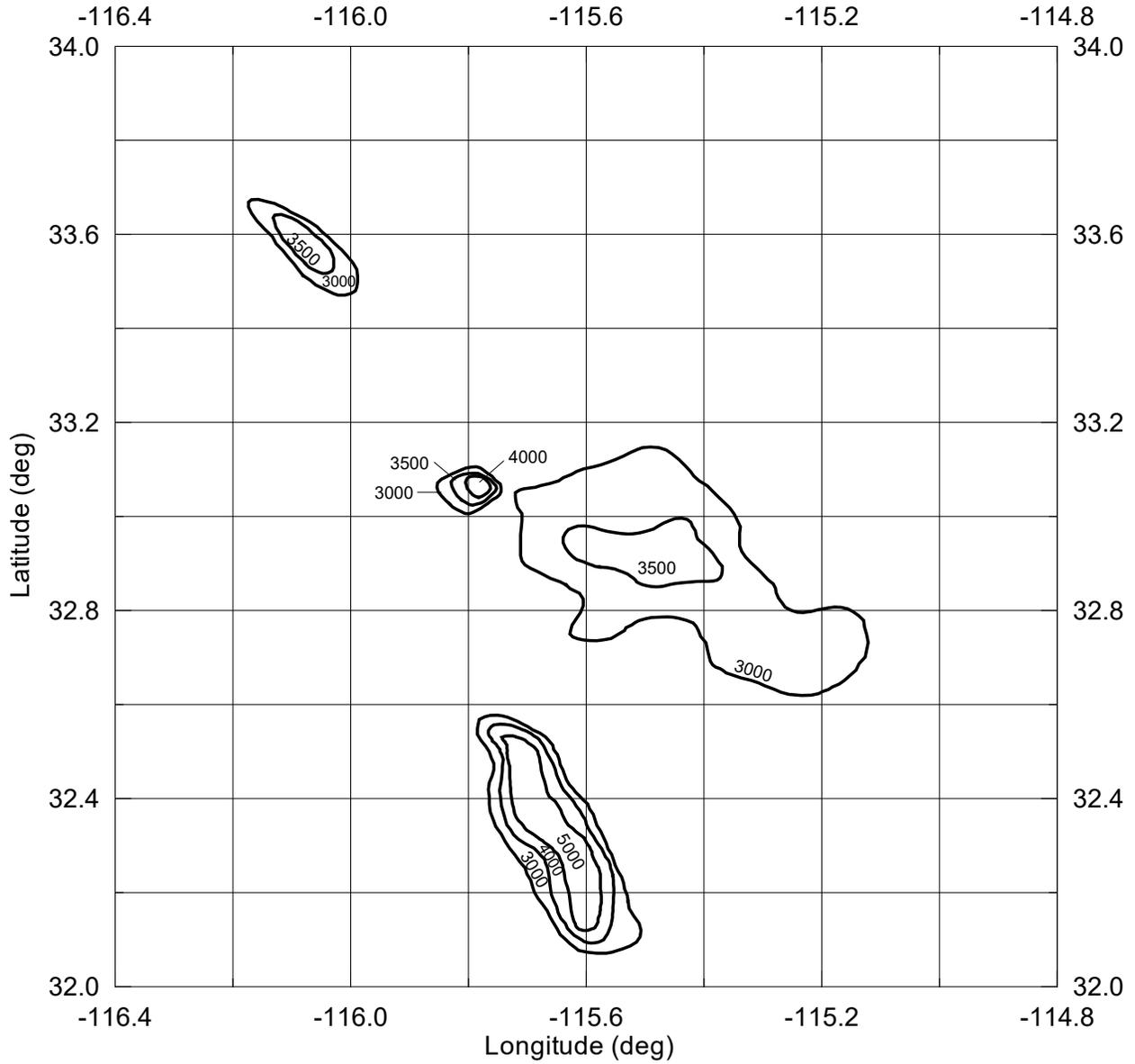
**Figure B.8** Contours of depth (meters) to shear wave velocity 2.5 km/s ( $Z_{2.5}$ ) in the Salton Basin (Imperial Valley)
