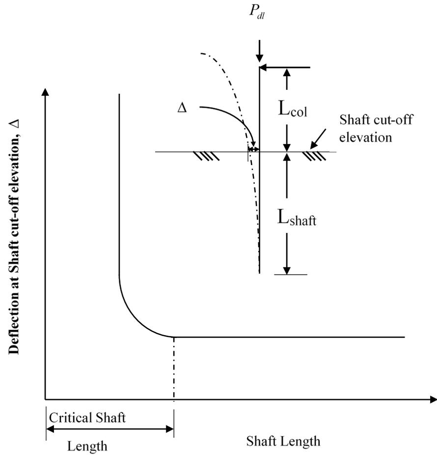
Figure C6.2.6-1 Lateral Stability Analysis of Shafts
