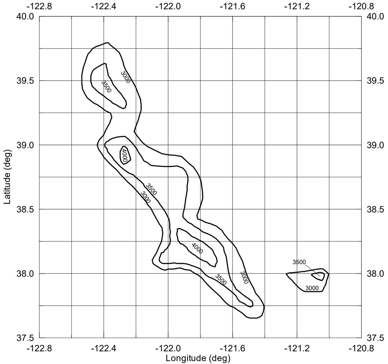
**Figure B.9** Contours of depth (meters) to shear wave velocity 2.5 km/s ( $Z_{2.5}$ ) in Northern California
