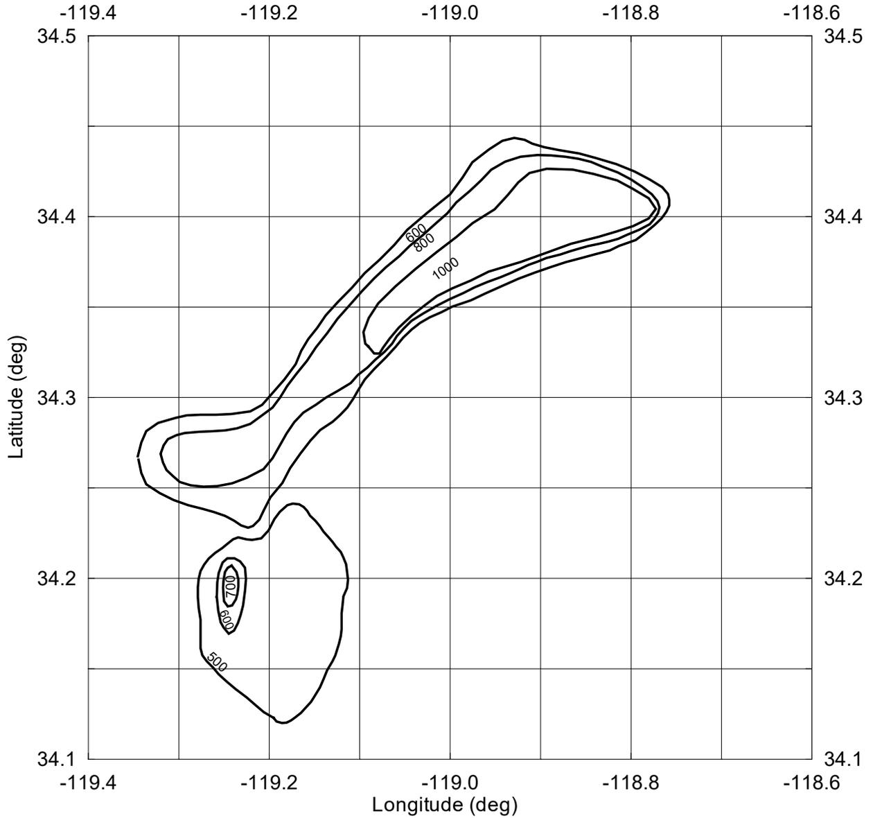
**Figure B.5** Contours of depth (meters) to shear wave velocity 1 km/s ( $Z_{1.0}$ ) in the Ventura Basin
