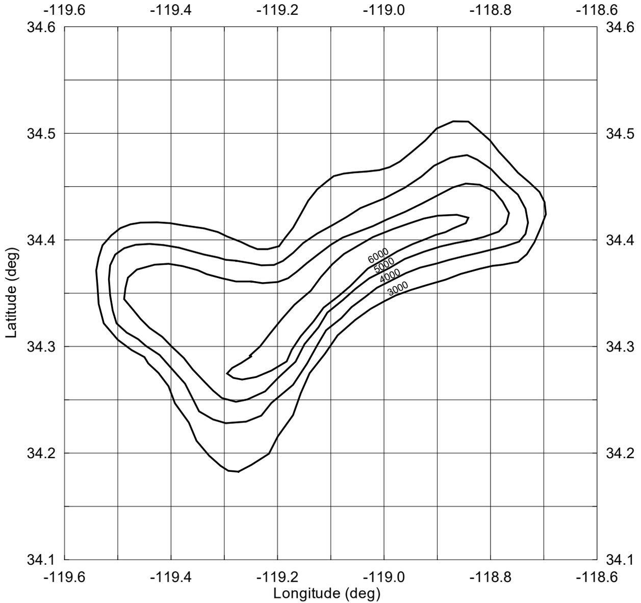
**Figure B.6** Contours of depth (meters) to shear wave velocity 2.5 km/s ( $Z_{2.5}$ ) in the Ventura Basin
