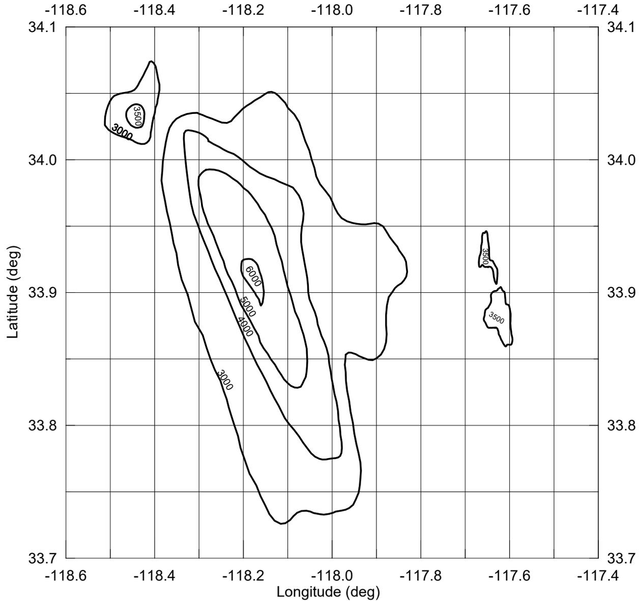
**Figure B.4** Contours of depth (meters) to shear wave velocity 2.5 km/s ( $Z_{2.5}$ ) in the Los Angeles Basin
