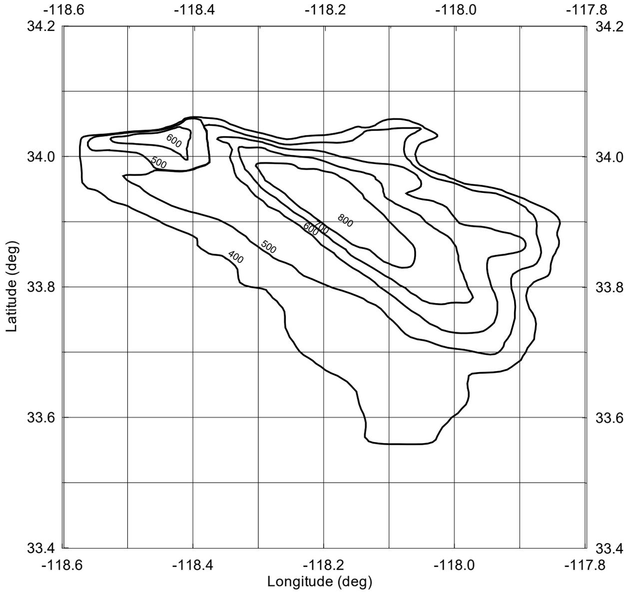
**Figure B.3** Contours of depth (meters) to shear wave velocity 1 km/s ( $Z_{1.0}$ ) in the Los Angeles Basin
