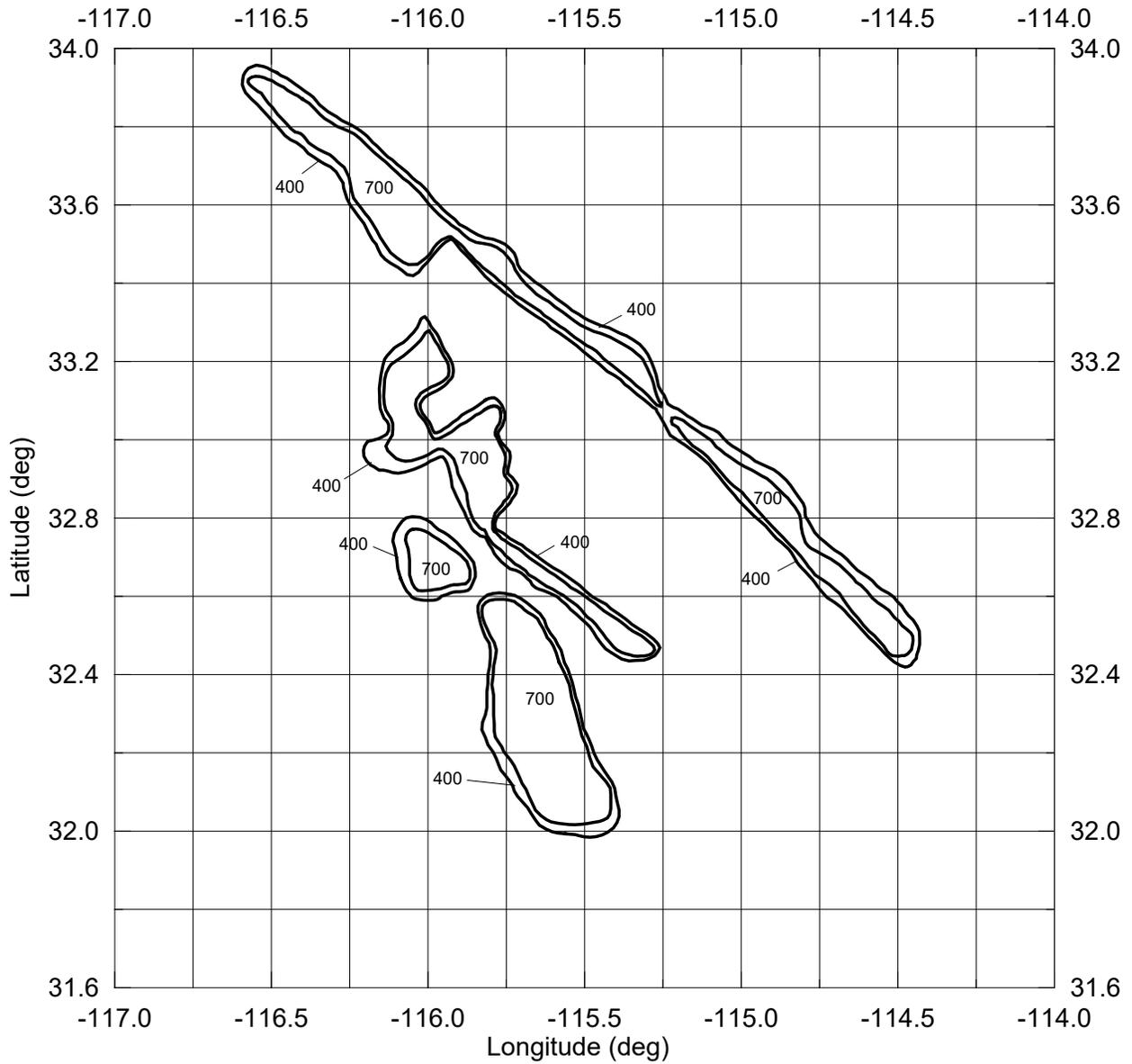
**Figure B.7** Contours of depth (meters) to shear wave velocity 1 km/s ( $Z_{1.0}$ ) in the Salton Basin (Imperial Valley)
