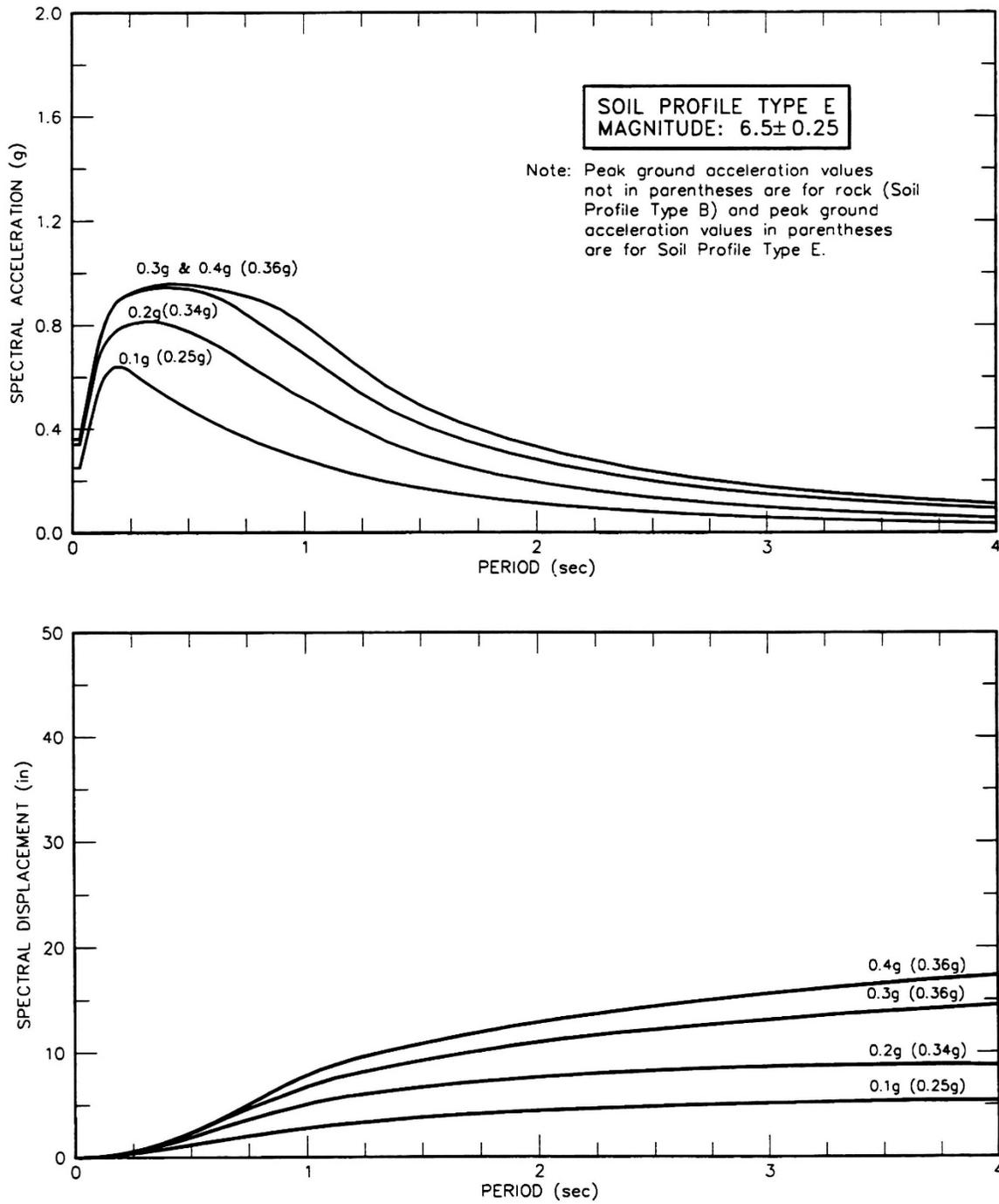
**Figure B.11** Spectral Acceleration and Displacement for Soil Profile E ( $M = 6.5 \pm 0.25$ )
