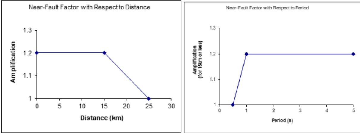
**Figure B.1** Near-Fault adjustment factor as a function of distance and spectral period. The distance measure is based on the closest distance to any point on the fault plane
