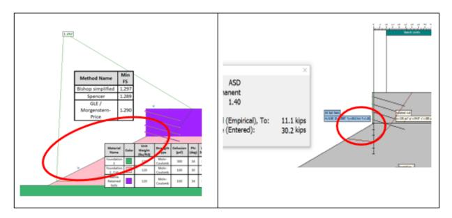
The overall stability of soil nail walls using slope stability software does not require separate models for global and compound stability, and both analyses can be performed in a single analysis model by adjusting search limits where all soil nail elements are modeled.
