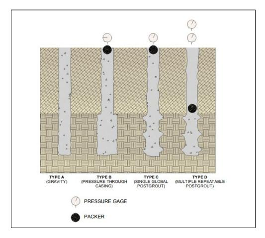
Figure 2: Micropile Types (from FHWA NHI-05-039)
