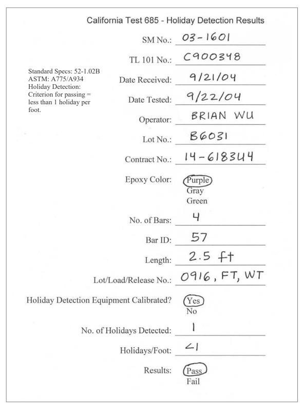
Figure 1 Test Form for Recording Holiday Detection Results
