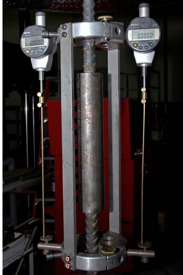
FIGURE 1A. Measuring device with dial indicators used for measuring slip.
