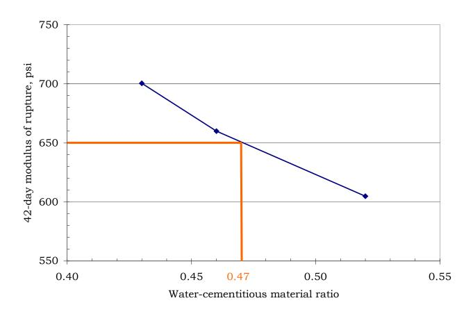
FIGURE 2. Water/Cementitious Material Ratio vs. Flexural Strength
