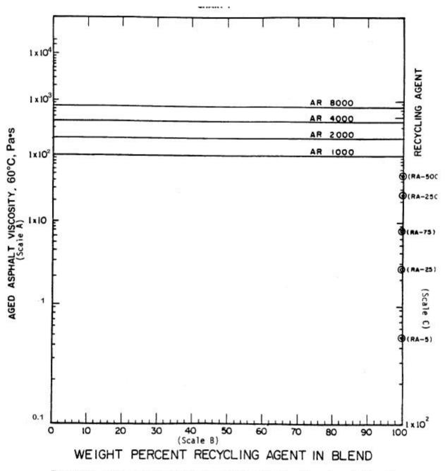
TO USE: Draw a straight line connecting viscosity of aged asphalt with viscosity of recycling agent. Draw a vertical line up from the percent recycling agent in blend. The two lines intersect at predicted approximate viscosity of the recycled asphalt.
