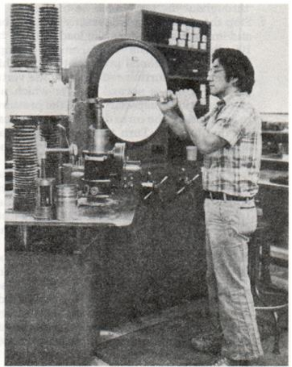
FIGURE 2. Transferring of the test specimen from the mold to the Stabilometer
