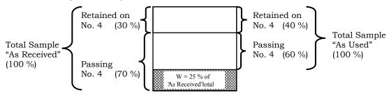
**Adjustment #3:** Single sample with a portion of the material retained on a designated sieve to be wasted.
