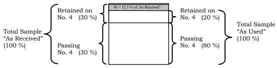
**Adjustment #4:** Single sample with all of the material passing a designated sieve to be wasted.
