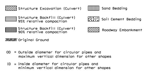
Figure 12.10.4.3.1-1—Non-Standard Installation Excavation and Backfill
