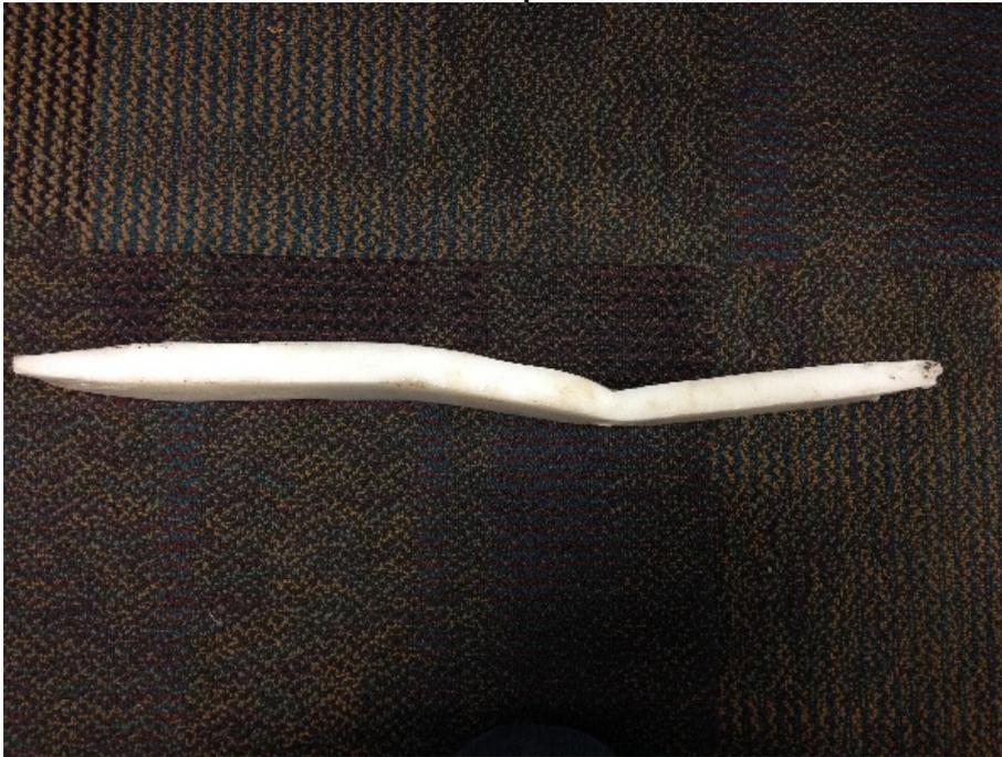
Figure 2: Damaged Deflector
