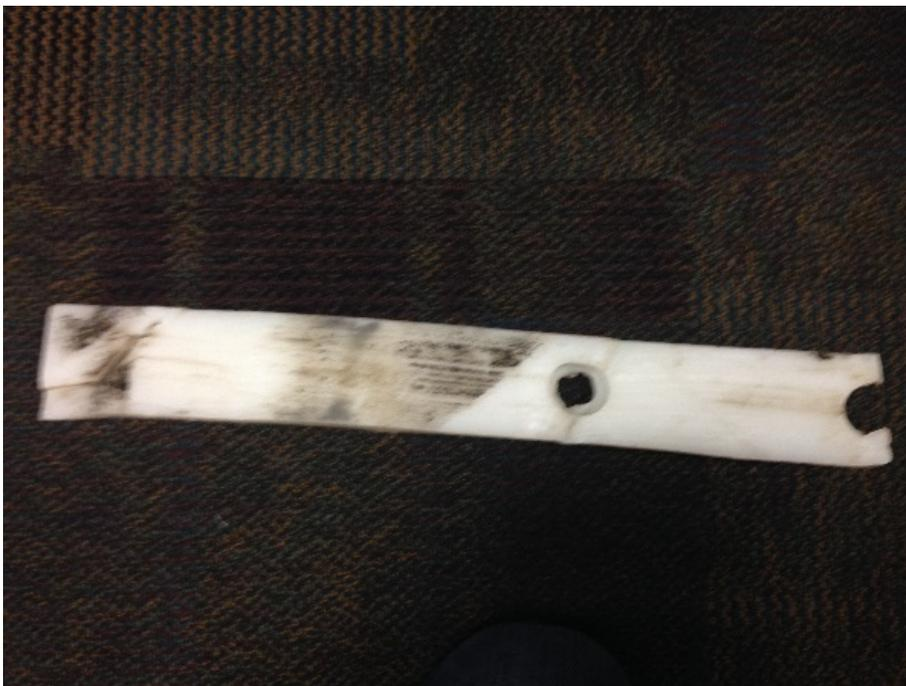
Figure 3: Damaged Deflector
