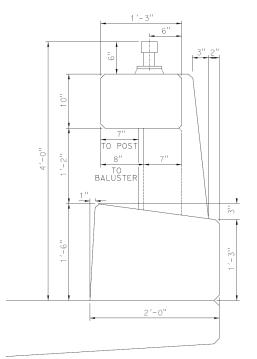
Figure 1 Typical Section of Concrete Barrier Type 86H
