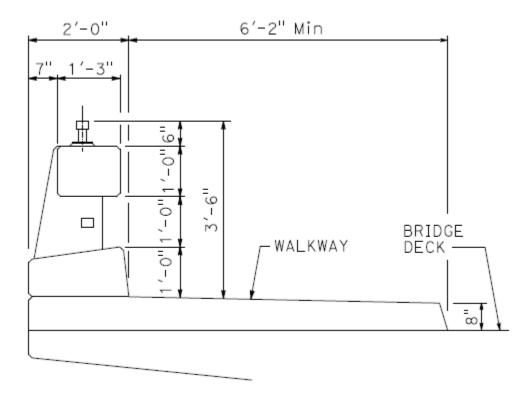
Concrete Barrier Type 85SW bridge railing (Type 85SW)
