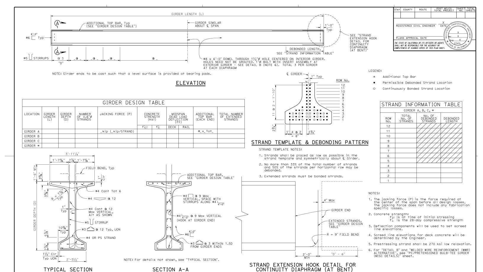
NO SCALE BRIDGE STANDARD DETAILS BRIDGE No. STATE OF DESIGN DIVISION OF XX-XXXX xs1-121-1 CALIFORNIA October 2025 DETAILS POST MILE **ENGINEERING SERVICES** PC/PRETENSIONED BULB-TEE GIRDER (DEBONDED STRANDS) CHECKED DEPARTMENT OF TRANSPORTATION QUANTITIES X.X UNIT: XXXX COUNTY/ROUTE/ZONE: XXX/XXX/X DATE PLOTTED => 29-SEP-2025 Refer to: http://www.dot.ca.gov/hq/esc/techpubs/manual/ bridgemanuals/bridge-standard-detail-sheets/index.html TIME PLOTTED => 14:30
