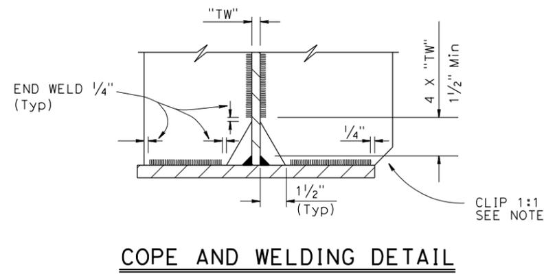
NOTE: Omit clip at bottom flange when less than 2".
