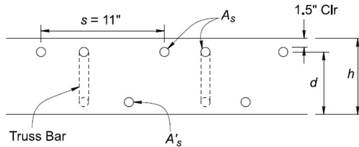
**Figure 16.8.4-2 Deck Overhang Cross-Section**
