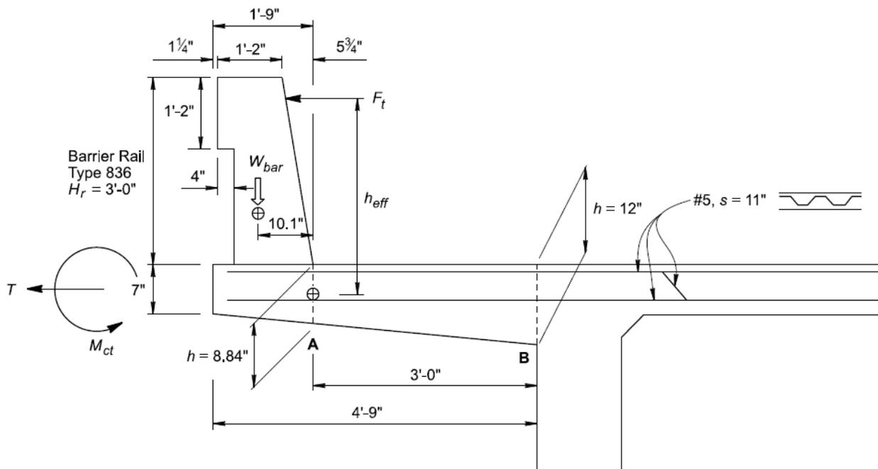
Figure 16.8.4-1 Example of Existing Deck Overhang
