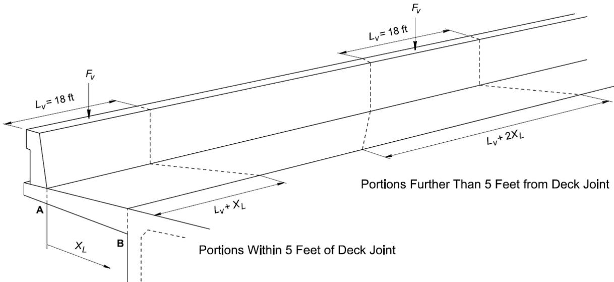
Figure 16.8.4.2-1 Effective Length of Deck Overhang Resisting  $F_v$
