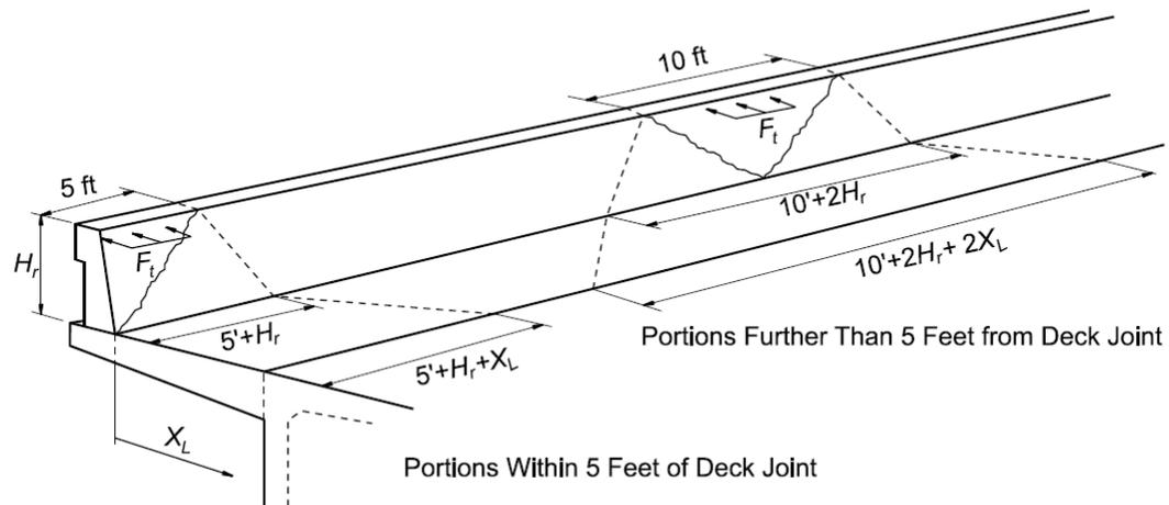
**Figure 16.8.4.1-1 Effective Length of Deck Overhang Resisting Rail Collision Force**
