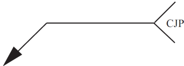
Figure 11.3.1 CJP Welding Symbol
