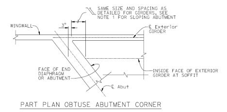
Figure 9.6.1 Stirrup Reinforcement at Abutments (Sloping Exterior Girder)
