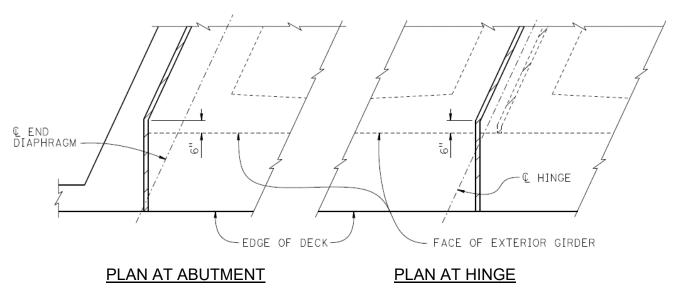
Figure 9.4.2 Deck Joints at Vertical Exterior Girders (Over 20° Skew)
