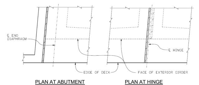
Figure 9.4.1 Deck Joints at Vertical or Sloping Exterior Girders (Skew 0° to 20°)
