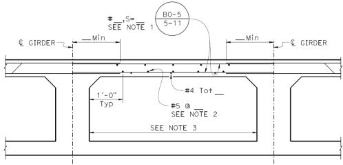
Figure 8.6.2 Transverse Reinforcement for Interior Girders
