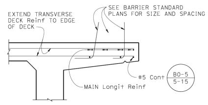
Figure 8.7.1 Barrier and Sidewalk Minimum Longitudinal Reinforcement
