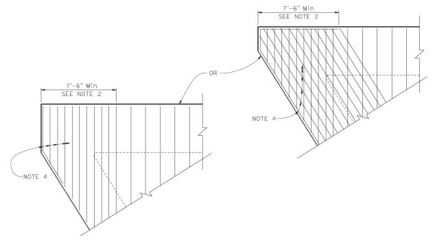
Figure 8.9.1 Skewed Deck Corner Reinforcement (Over 20° Skews)
