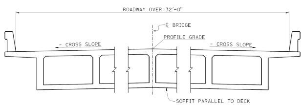
Figure 8.2.2 Box Girder Parallel Soffit
