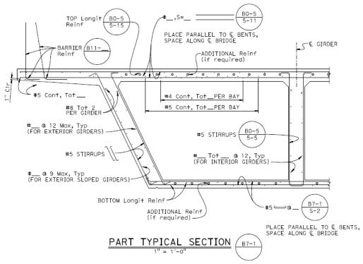
Figure 8.5.1 Part Typical Section Details
