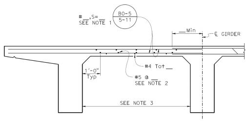
Figure 8.6.1 Transverse Reinforcement for Exterior Girders
