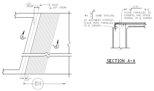
Figure 8.8.1 Transverse Deck Reinforcement Details at Abutment (≤ 20° Skew)
