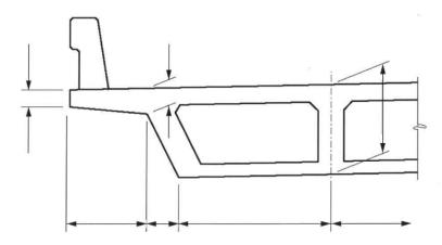
Figure 8.3.2 Sloped Exterior Girder Dimensions
