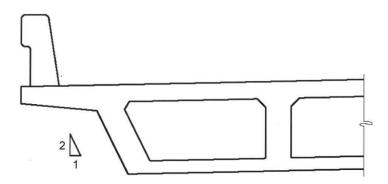
Figure 8.3.1 Sloped Exterior Girder
