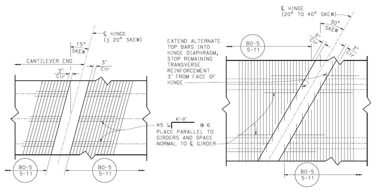
Figure 8.8.4 Transverse Deck Reinforcement Details at Hinge (≤ 40° Skew)
