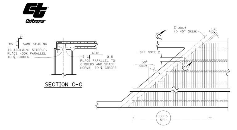
Figure 8.8.3 Transverse Deck Reinforcement Details at Abutment (> 40° Skew)
