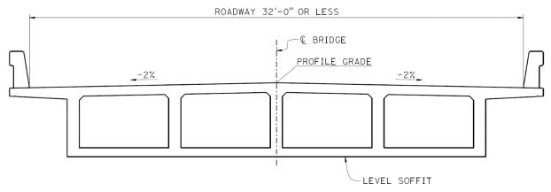
NOTE: The soffit may be cast on a straight line between the outside bottom edges of the box girder as approved by Engineer. Deck slab thickness remains as shown. Stem and stirrup heights and soffit thickness will vary to meet finished grade and provided clearances shown.
