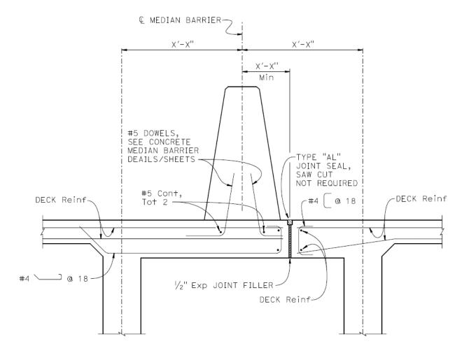
Figure 8.10.1 Median Slab with Concrete Barrier
