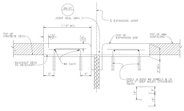
Figure 8.14.1 Polyester Concrete Expansion Dam
