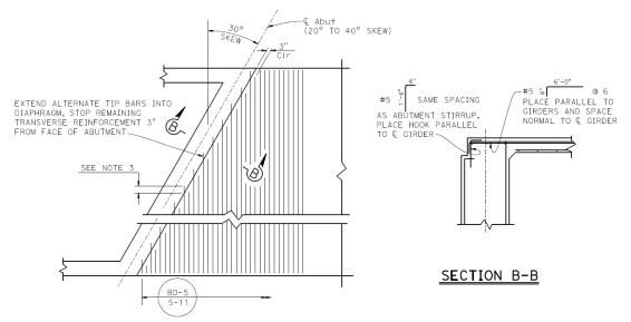
Figure 8.8.2 Transverse Deck Reinforcement Details at Abutment (20° to 40° Skew)
