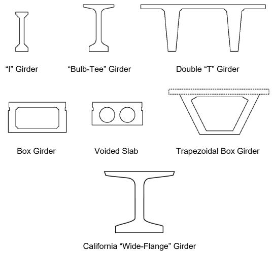
Figure 8.4.1 Standard Precast Girders
