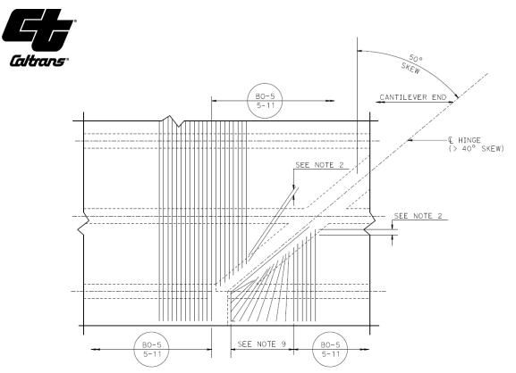
Figure 8.8.5 Transverse Deck Reinforcement Details at Hinge (> 40° Skew)
