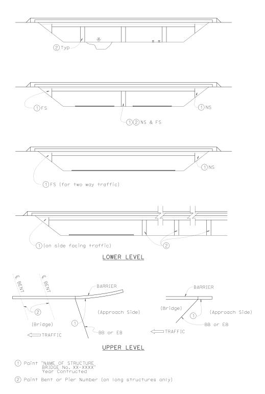
Figure 3.30.1 Structure Identification
