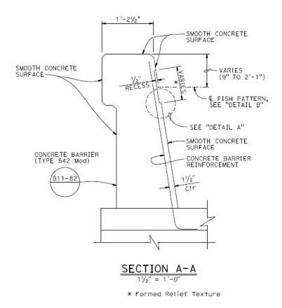
Figure 1.5.1 Example of modified barrier
