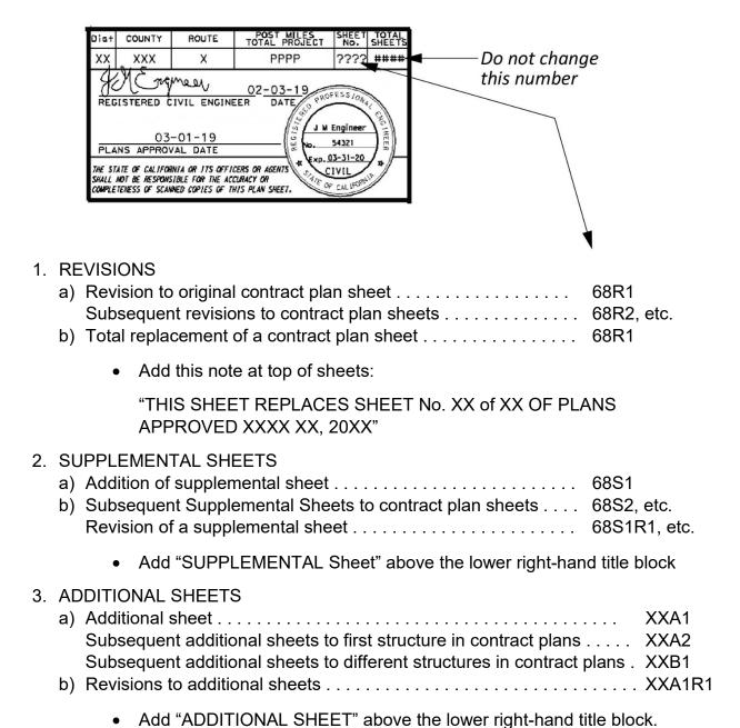
Figure 1.20.1 Seal signature and block
