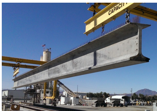
B) Pretensioned wide-flange girder
