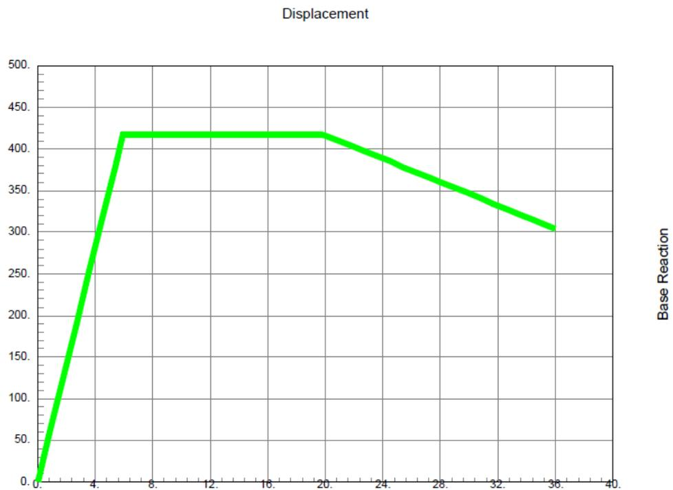
Figure 20.2.9-12 Force-Displacement Curve at Bent 2
